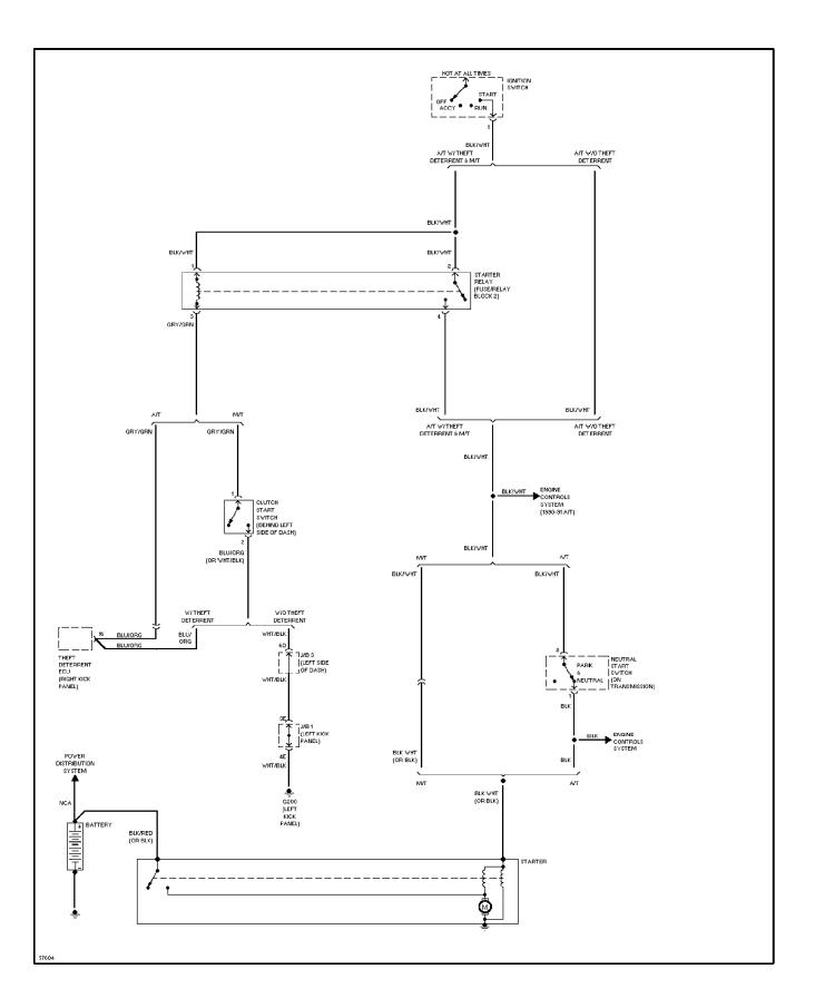
WIRING DIAGRAMS Fig. 10: Junction Block #3 (Coupe), J1 Conn, A/T Ind (Grid 36-39) 1991 Toyota Corolla
