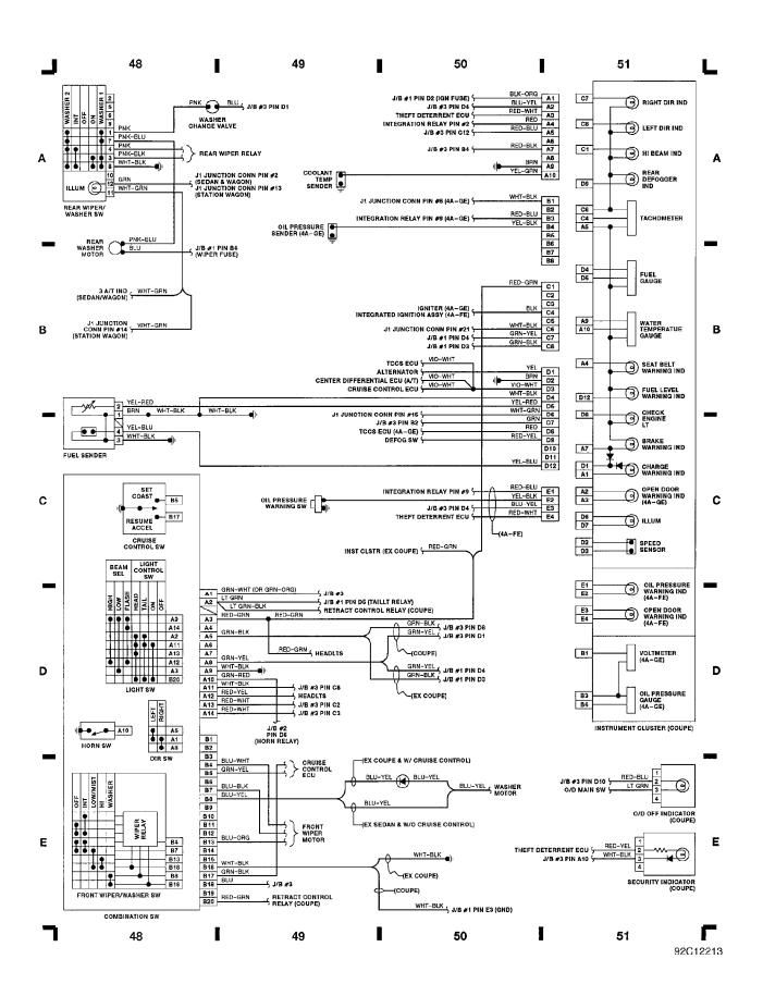
WIRING DIAGRAMS Fig. 14: Ctr Differential Ctrl Sw, Theft Deterrent (Grid 52-55) 1991 Toyota Corolla
