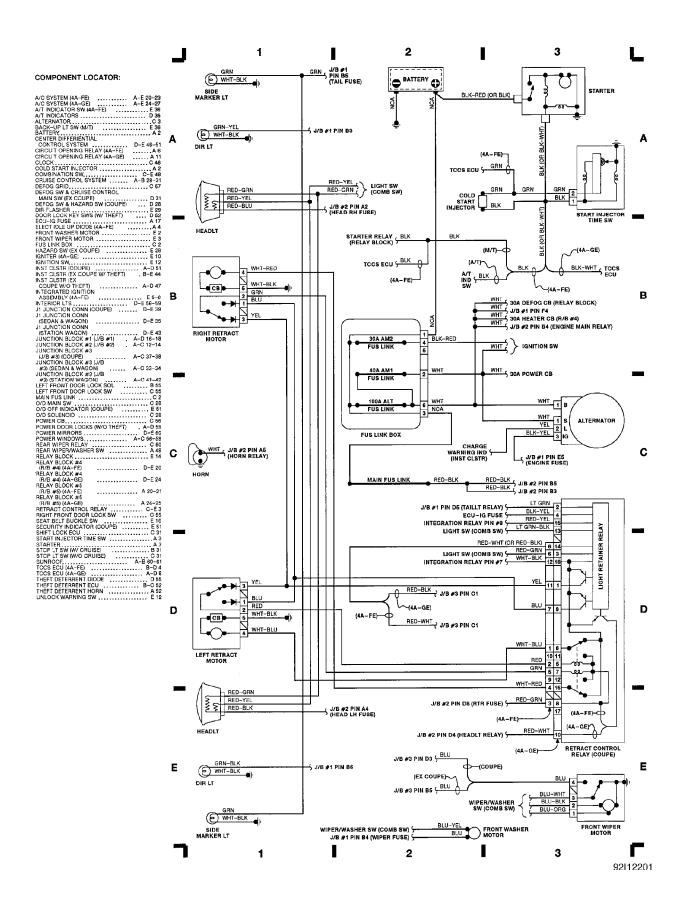
WIRING DIAGRAMS Fig. 2: Computer Engine Control (1.6L 4A-FE) (Grid 4-7) 1991 Toyota Corolla
