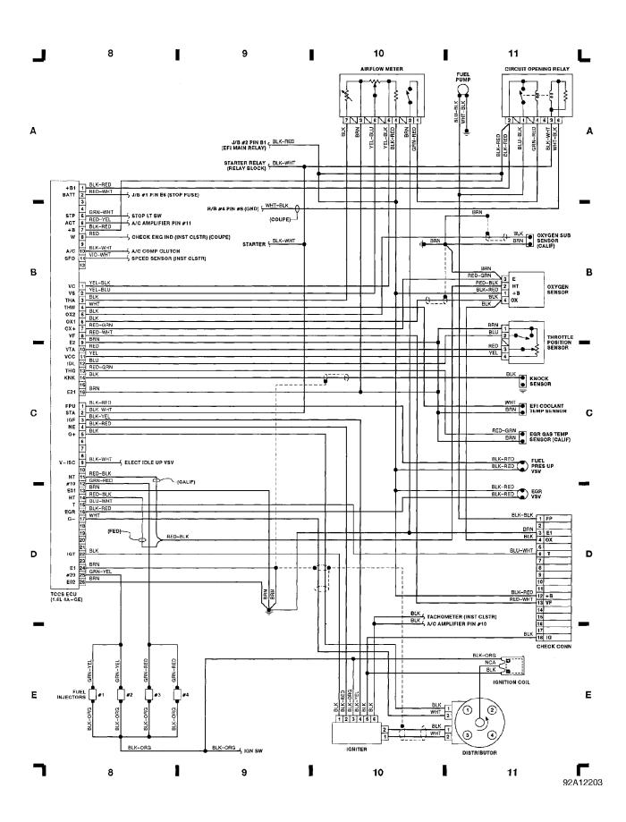
WIRING DIAGRAMS Fig. 4: Junction Block #2 (J/B #2), Ignition Sw (Grid 12-15) 1991 Toyota Corolla
