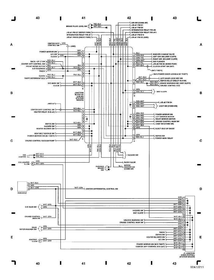
WIRING DIAGRAMS Fig. 12: Inst Clstr (Ex Coupe W/ W/O Theft), Fuel Send (Grid 44-47) 1991 Toyota Corolla
