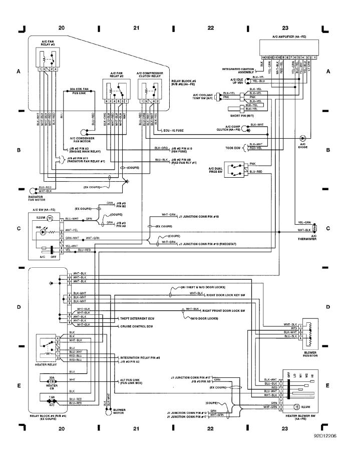
WIRING DIAGRAMS Fig. 7: 4A-GE A/C & Heater, Relay Block #4 & #6 (Grid 24-27) 1991 Toyota Corolla
