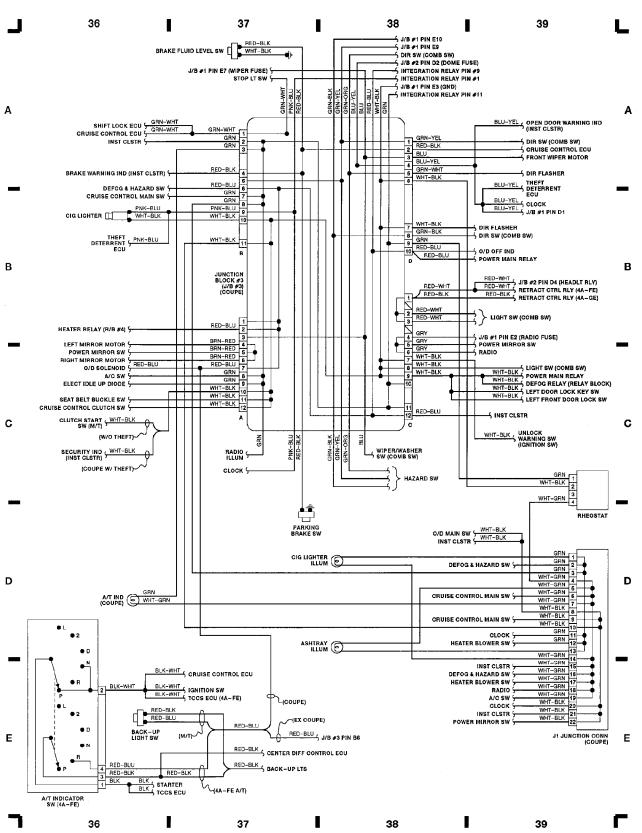
WIRING DIAGRAMS Fig. 11: Junction Block #3 (Station Wagon), (Grid 40-43) 1991 Toyota Corolla
