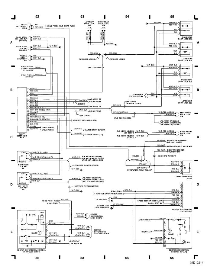
WIRING DIAGRAMS Fig. 15: Pwr Windows/Doors/CB, Interior Lights (Grid 56-59) 1991 Toyota Corolla
