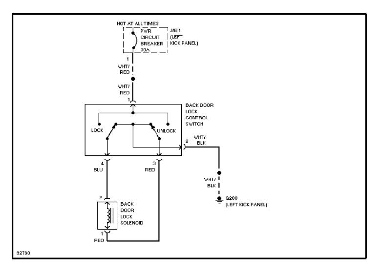
WIRING DIAGRAMS Fig. 9: Junction Block #3 (Sedan & Wagon), J1 Conn (Grid 32-35) 1991 Toyota Corolla
