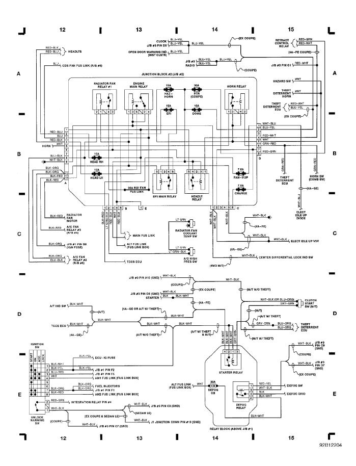
WIRING DIAGRAMS Fig. 5: Junction Block #1 (J/B #1) (Grid 16-19) 1991 Toyota Corolla
