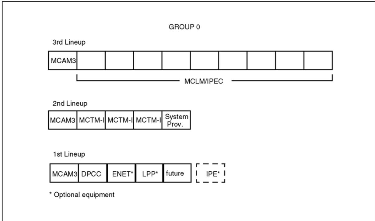
The second lineup of the primary group for a full-size SuperNode system consists of the Meridian Cabinet Auxiliary Module phase 3 (MCAM3), followed by three Meridian Cabinet Trunk Module-ISDN (MCTM-I) cabinets and a system provisionable cabinet.
