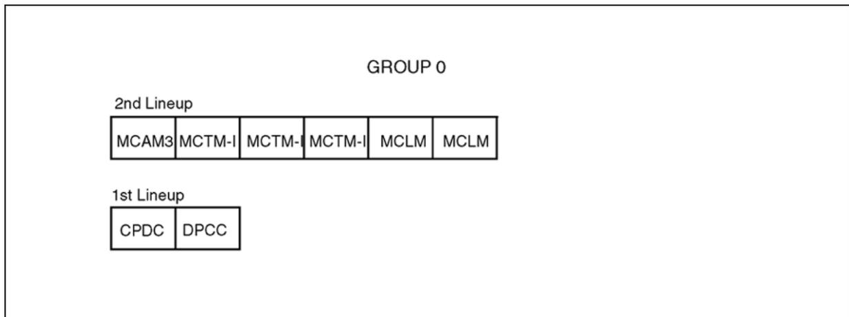
Secondary group lineups can also be merged for floor space efficiencies. Lineups 1 and 2 of a secondary group consisting of an MCAM3, MCTM-I, and MCLM can be merged into a single lineup as shown in Figure 70 "Secondary group merged into a single lineup" (page 145).
