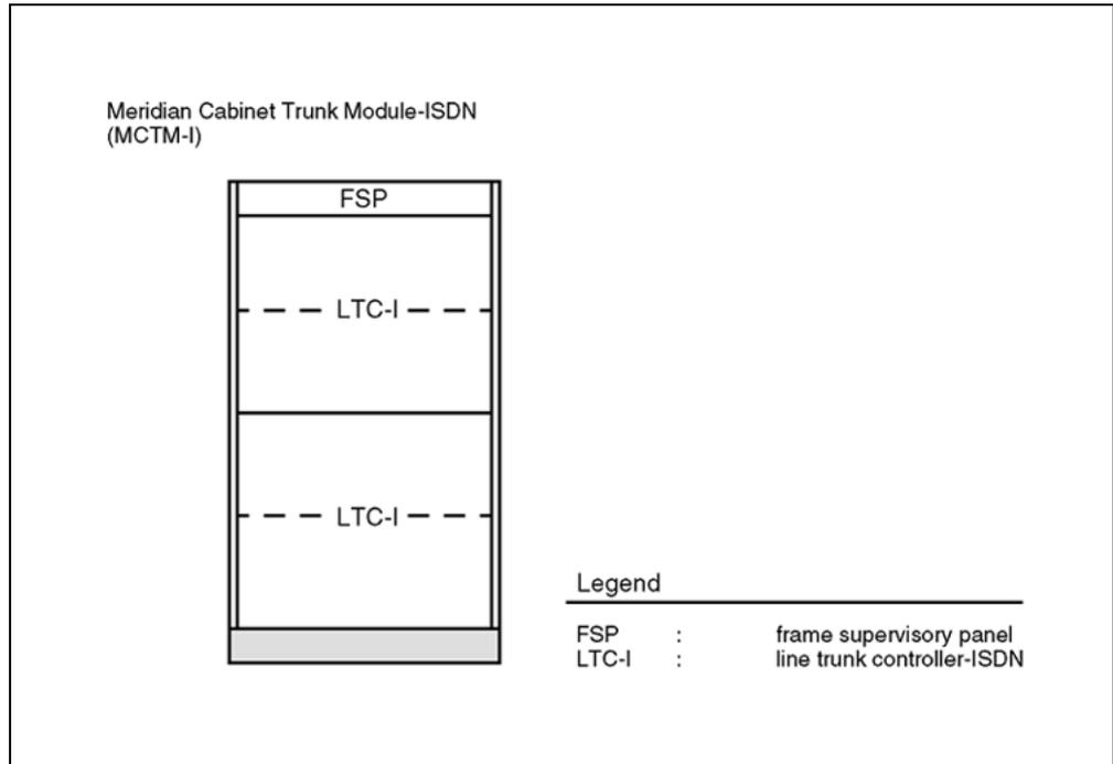
LTC-I's are provisioned with Universal Tone Receivers (UTRs) containing 30 circuits. An additional 30 circuits can be provisioned with an additional pair of circuit cards.
