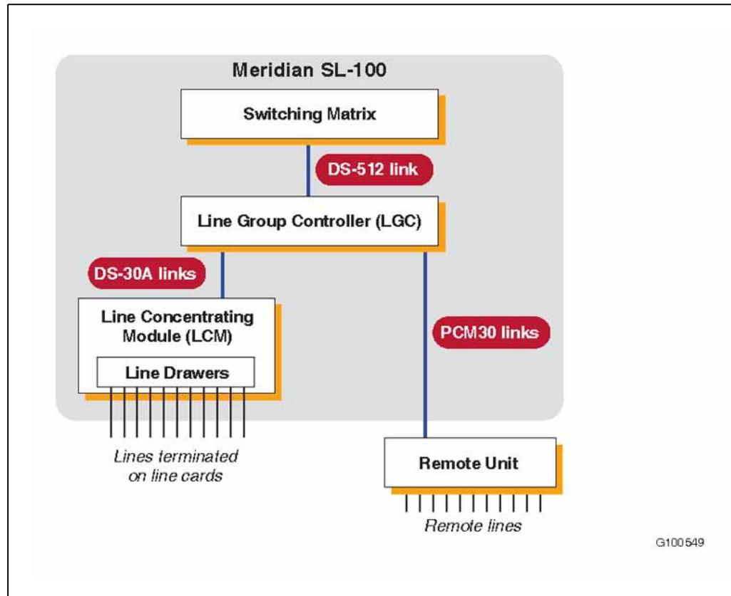
The Line Group Controller provides call processing and handling capabilities, tone circuits and a time switch that can connect individual 64 kbps P-side channels with C-side channels to/from ENET.
