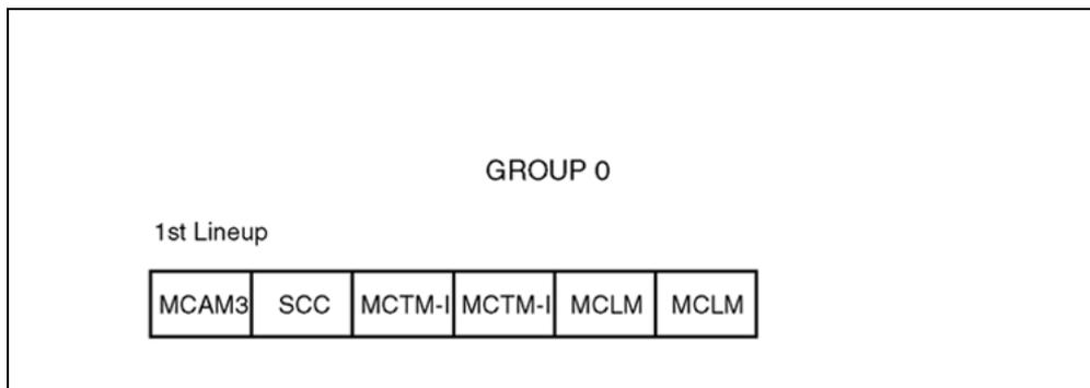
A single lineup can be engineered only if the MCAM3 is used as the power source. If a CPDC is used to power the SCC, a second lineup is required. Additionally, if an IPE, LPP, or both are added, a second lineup must be provisioned consisting of these cabinets, plus a CPDC to supply power.
