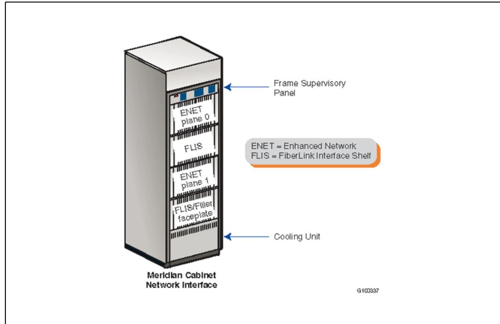
The MCNI provides a reduced-footprint solution for businesses to take advantage of the advanced capabilities of the Enhanced Network. The MCNI meets the interface requirements of evolving server-based applications such as Symposium Call Center, Symposium CompuCALL Telephony Application Programming Interface (TAPI) Driver, Optivity Telephony Manager for Meridian SL-100 (OTM-MSL) and an array of applications using the Ethernet Interface Unit (EIU).
