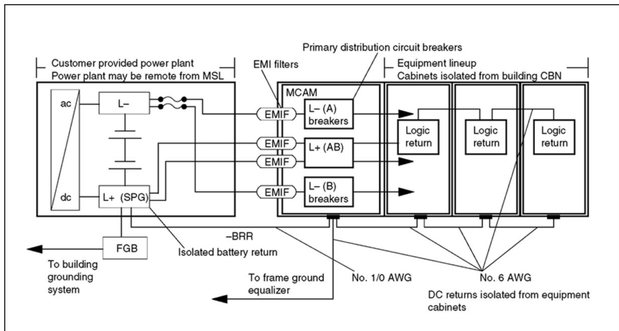
[Figure 34 "Frame ground and battery return connections"](#) (page 89) shows the frame ground and battery return connections between lineups. The frame ground connections connect the frames of each lineup to the frame grounding reference, a single point ground. The battery return connections connect the A-feed battery return to the B-feed battery return in alternate lineups to ensure battery return equalization among lineups.
