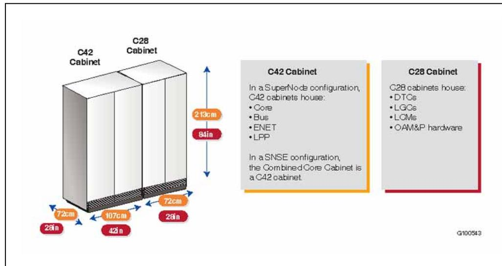
**Note:** Standard Meridian SL-100 frames are also used to house the Spectrum Peripheral Module. The dimensions of the Spectrum Peripheral Module hardware are smaller than those of equivalent Extended Peripheral Module (XPM) units, but to minimize costs adapter brackets are used to house Spectrum Peripheral Modules in existing frames. Overall footprint can still be reduced, because access to all cards in the Spectrum Peripheral Module double-height shelves is from
