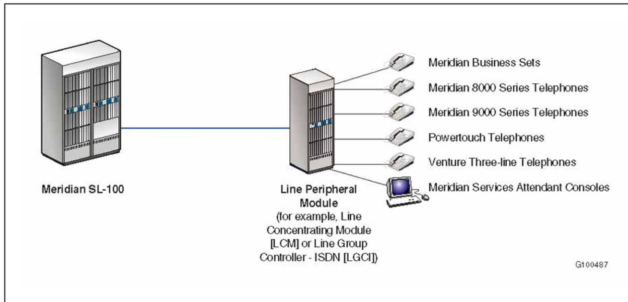
Supported Line Peripheral Module telephones can be broken down into the following families:
