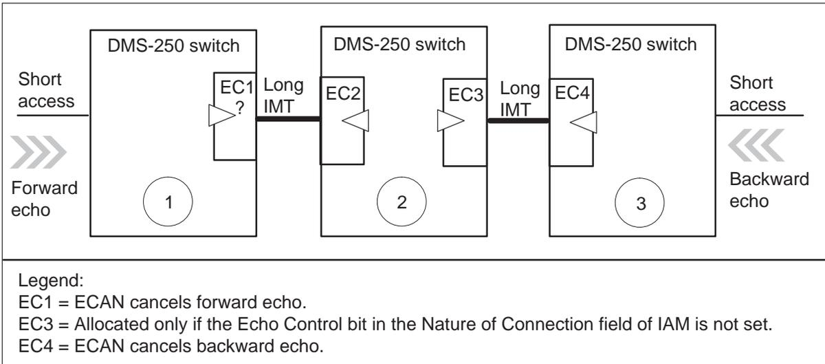
Provisioning as shown in case 4 results in redundant ECANs and wastes the internal ECAN.
