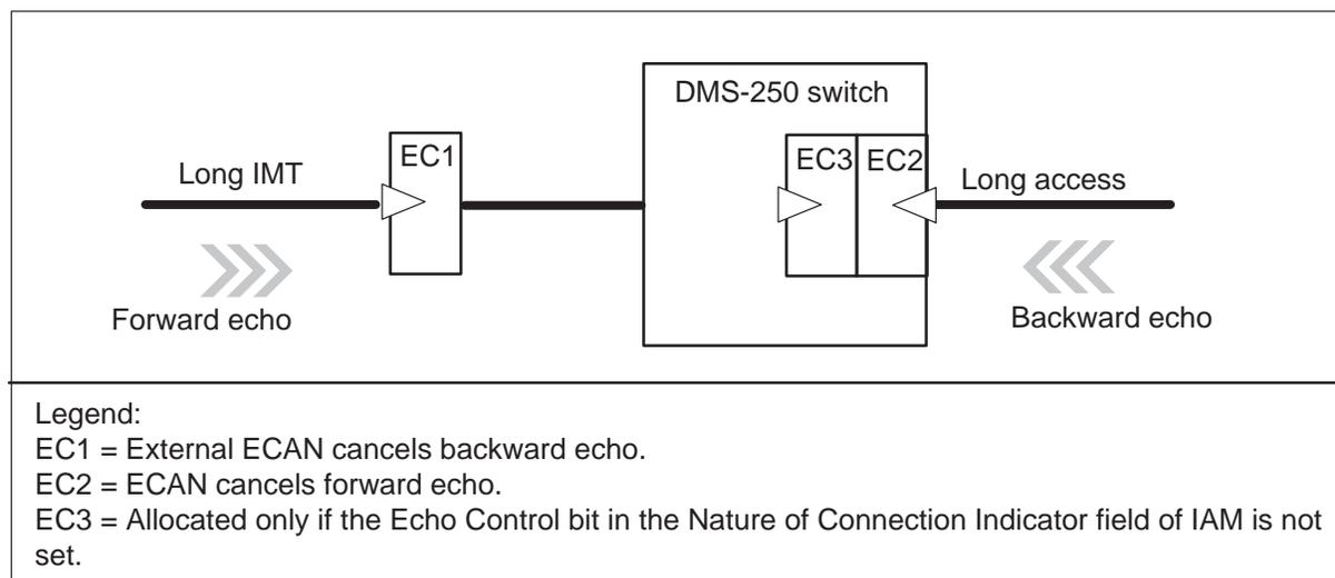
Provisioning as shown in case 4 results in redundant ECANs and wastes the the external ECAN.
