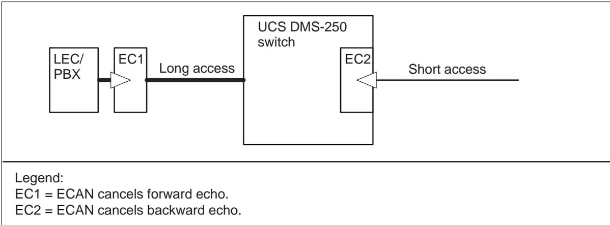
Figure 2-13 illustrates an interswitch call where Spectrum ECANs are provisioned on all access trunks.
