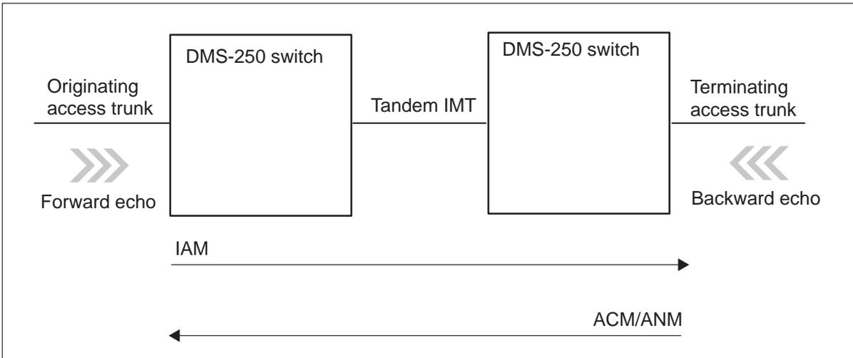
When a forward half Spectrum ECAN is enabled cancelling the outgoing echo, the Spectrum ECAN call control algorithm sets the Echo Control bit in the IAM. After this bit is set, all subsequent Spectrum ECANs in the network that cancel forward echo are not activated. The Echo Control bit is also set when the originating Spectrum trunk is provisioned with a Spectrum ECAN with the FAREC field set to “Y.”
