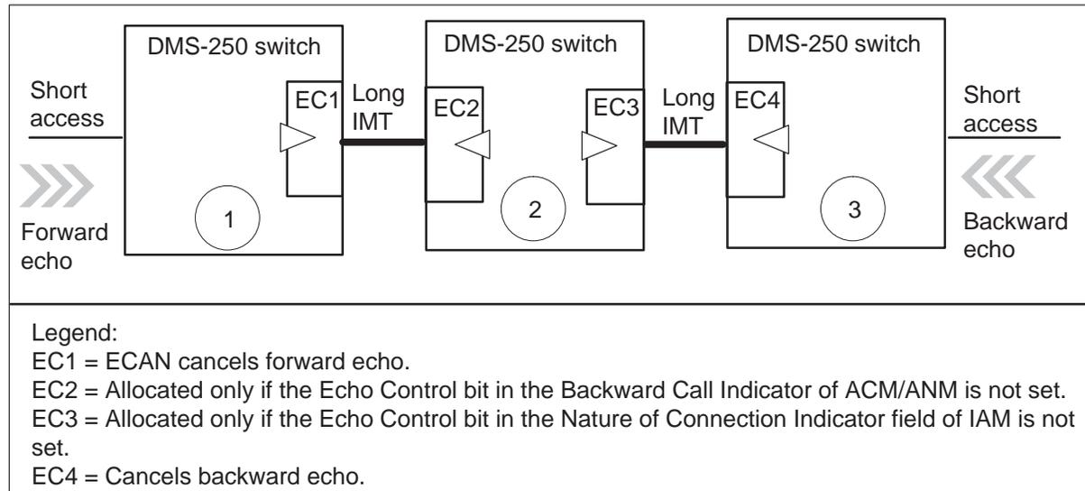
On switch 2, Spectrum ECANs are allocated only if the corresponding received Echo Control bits are not set. For example, if an ECAN provisioned on switch 3 is beyond the operating company's control, then to guarantee adequate echo cancellation, the IMT terminator on switch 2 is provisioned with back-to-back Spectrum ECANs. This is the situation encountered in case 8 and is illustrated in Figure 2-.
