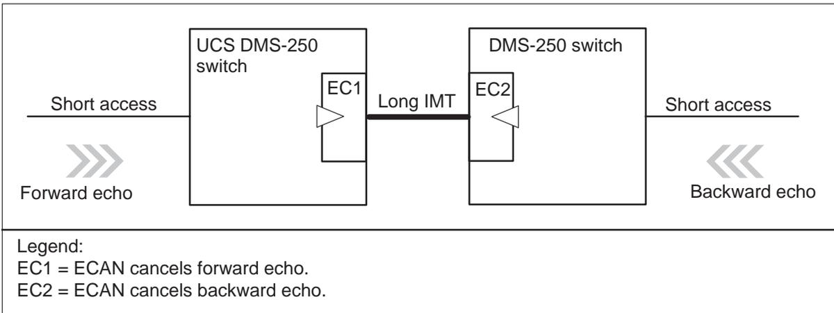
When ECAN provisioning at the other end of an IMT trunk is beyond the control of the provisioning party, back-to-back Spectrum ECANs on the IMT trunk are necessary. Although the Spectrum ECAN call control algorithm guarantees optimal ECAN allocation on the switch in concern, the lack of indication about the disposition of ECANs at the other end of the long IMT may result in redundant ECANs. Figure 2-24 illustrates this situation.
