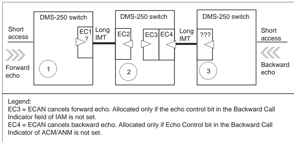
If the Echo Control bit in the Nature of Connection Indicator of the IAM is not set because EC1 is activated, ECAN EC3 is redundant.
