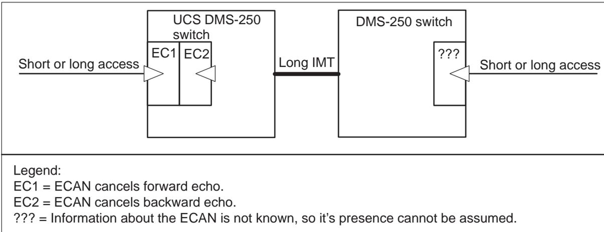
On long access trunks an external ECAN at the distant end provides better results. However, per-call control is lost. Figure 2-16 shows this configuration.
