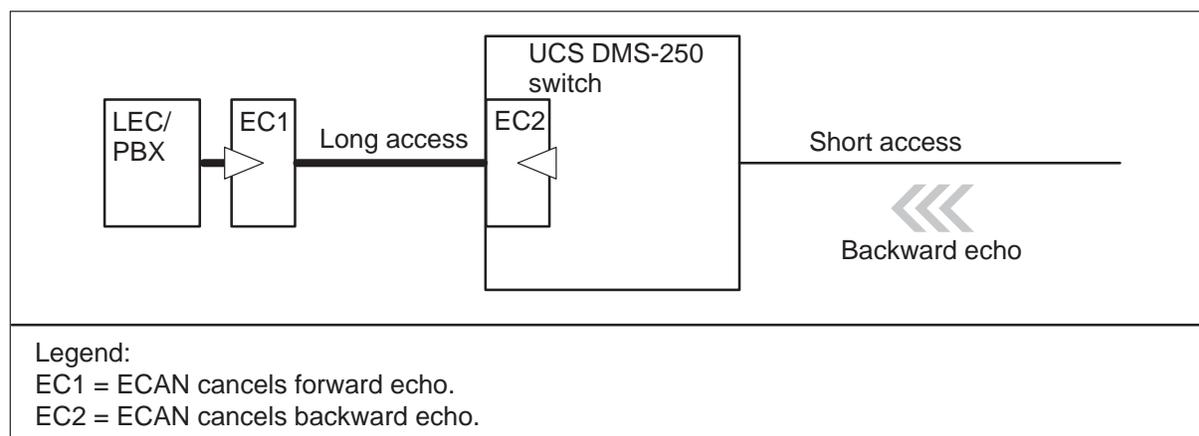
For long access to long access intraswitch calls, four ECANs are involved. Only the necessary number of Spectrum ECANs are allocated by the Spectrum ECAN call control algorithm.
