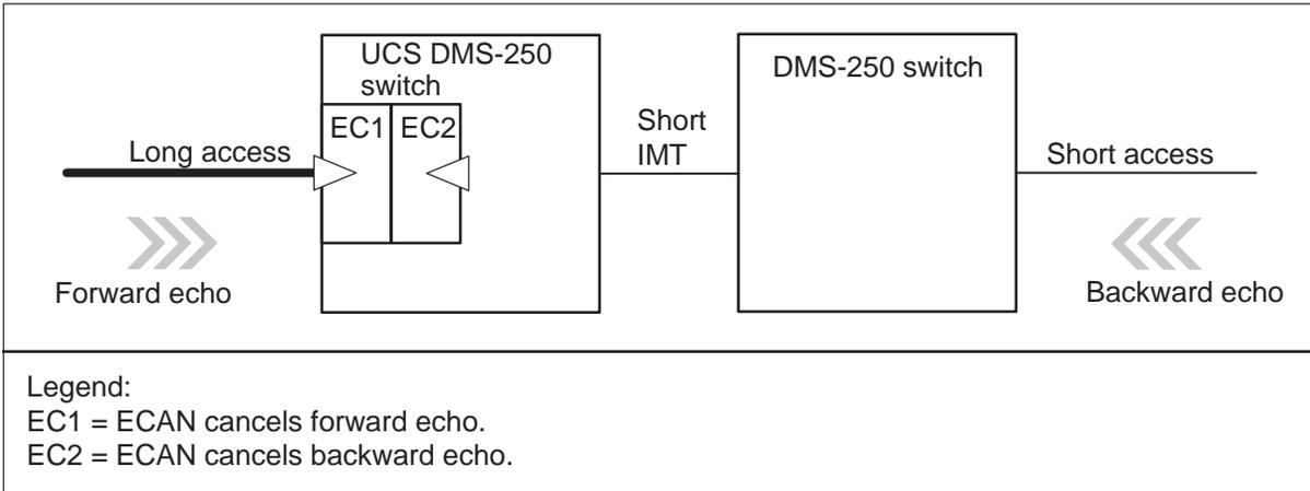
Figure 2-22 uses a long IMT provisioned with ECANs. The Spectrum ECAN call control algorithm allocates only the necessary ECANs.
