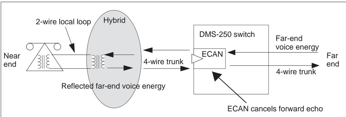
The other component necessary for the perception of echo is a delay in the reception of the reflected energy and the original energy transmission. This delay is referred to as round-trip delay. It is not possible to remove the delay component from the call. If the round-trip delay exceeds 15 milliseconds (typically), echo may be perceived if the reflected energy is at a perceivable level.
