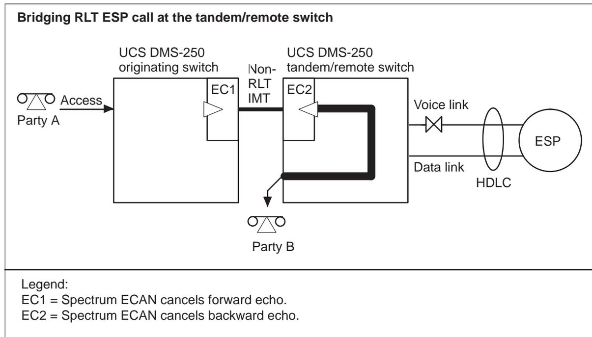
**AD9960****Spectrum ECAN Feature Interactions** (continued)**Scenario 28: Bridging RLT ESP call at the tandem/remote switch**
