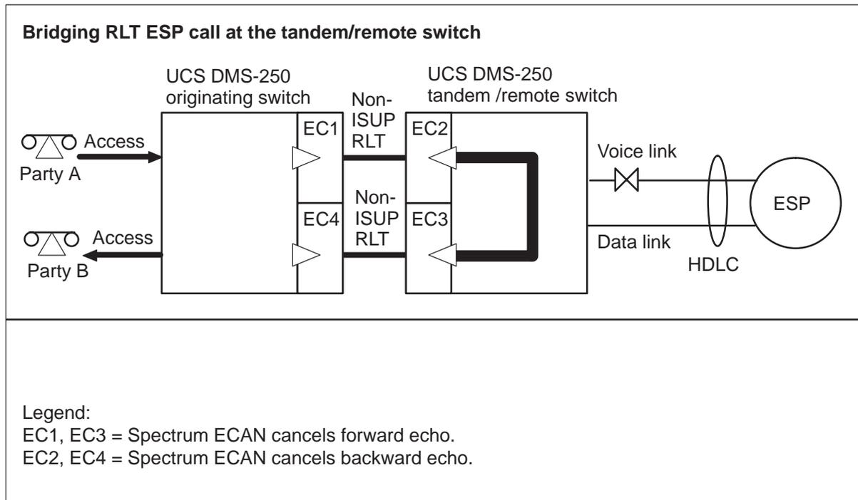
**AD9960****Spectrum ECAN Feature Interactions (continued)****Scenario 27: Bridging RLT ESP call at the tandem/remote switch**
