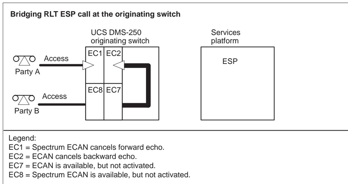
**AD9960****Spectrum ECAN Feature Interactions (continued)****Scenario 10: Bridging RLT ESP call at originating switch**
