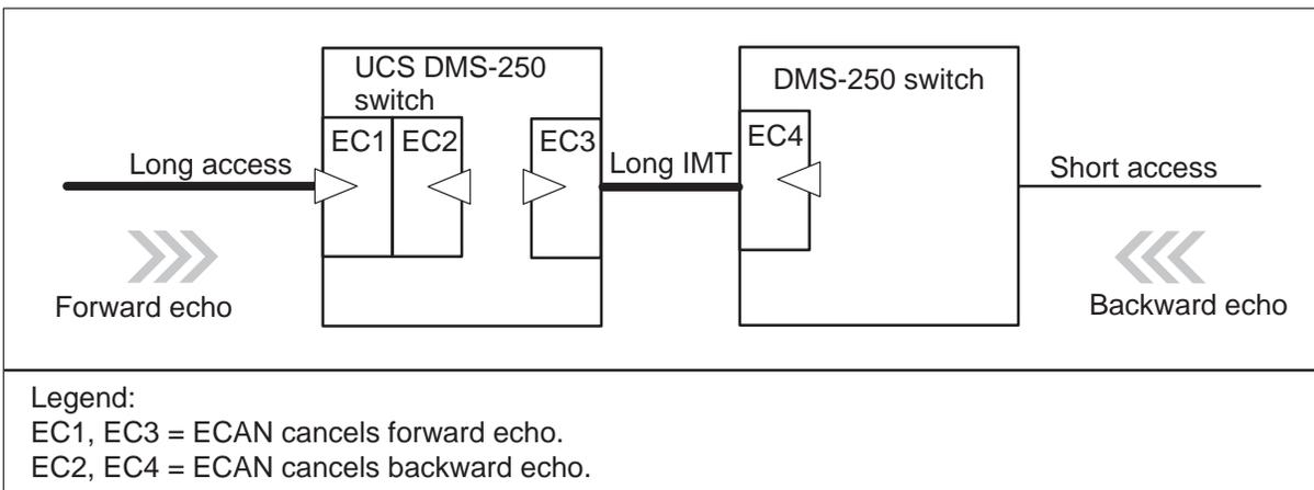
Figure 2-23 illustrates echo cancellation coverage for interswitch calls that originate and terminate on short access trunks.
