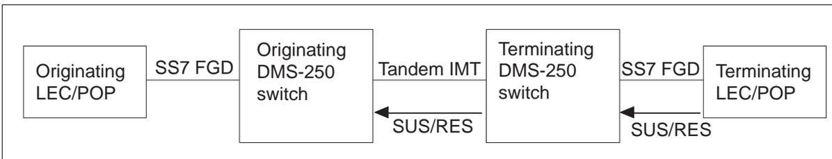
The receipt of the SUS message is interpreted as a temporary on-hook from the called party. The circuit connection remains and billing continues. The receipt of the RES message is interpreted as an off-hook from the called party and the call continues. If ECANs are present either on the originating, terminating, or both switches, when the terminator goes on-hook the ECAN
