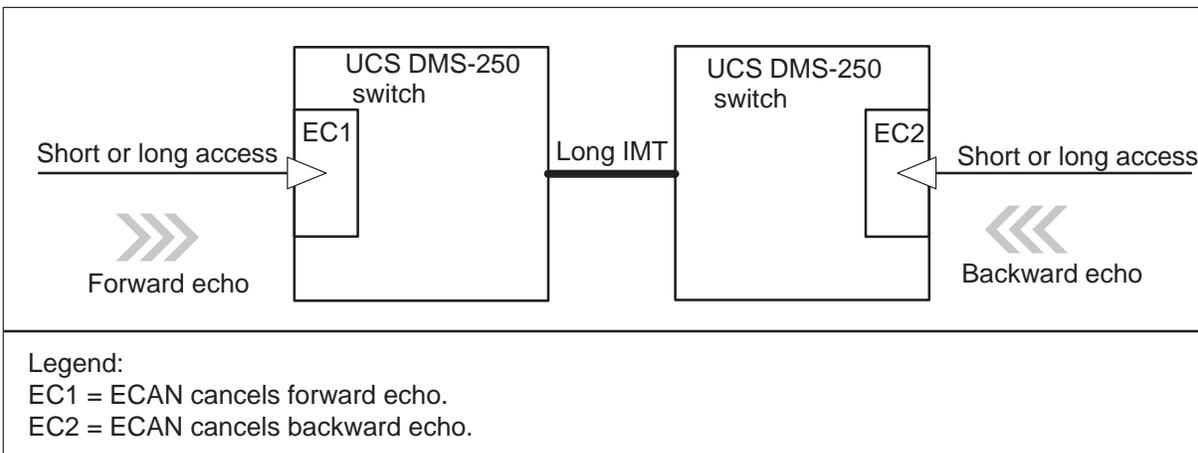
Figure 2-14 illustrates a scenario where external ECANs are used at the distant end (with respect to the DMS-250 switch) of the long access trunks. The per-call control capability is compromised for better echo cancellation.
