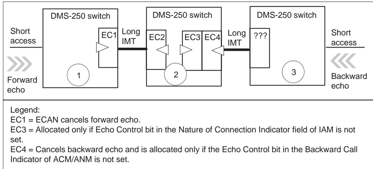
Redundant ECANs are possible in this situation if ECANs are allocated downstream and the Echo Control bit in the Backward Call Indicator of the ACM/ANM is not set. This is a case of IMT trunks displaying pseudo-access behavior. Use such configurations sparingly in order to conserve Spectrum ECAN resources.
