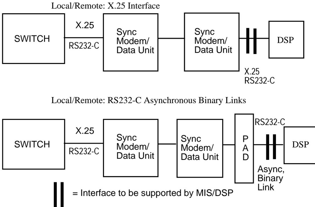
It should also be noted that the X.25 transmission path may be supported over either a direct link or over a packet switched network. However in case of Bellcore Publication 54001, see Section 2.3. It will be necessary to confirm compatibility with the particular packet switched network because this implementation of X.25 supports a (non-standard) default packet size of 256 bytes, and a Data Network address size of 8 digits which is associated with both calling and called addresses.
