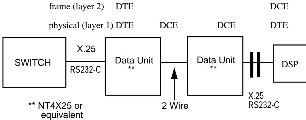
**Figure 2-4 Switch to DSP connection configuration with Synchronous Modems**
