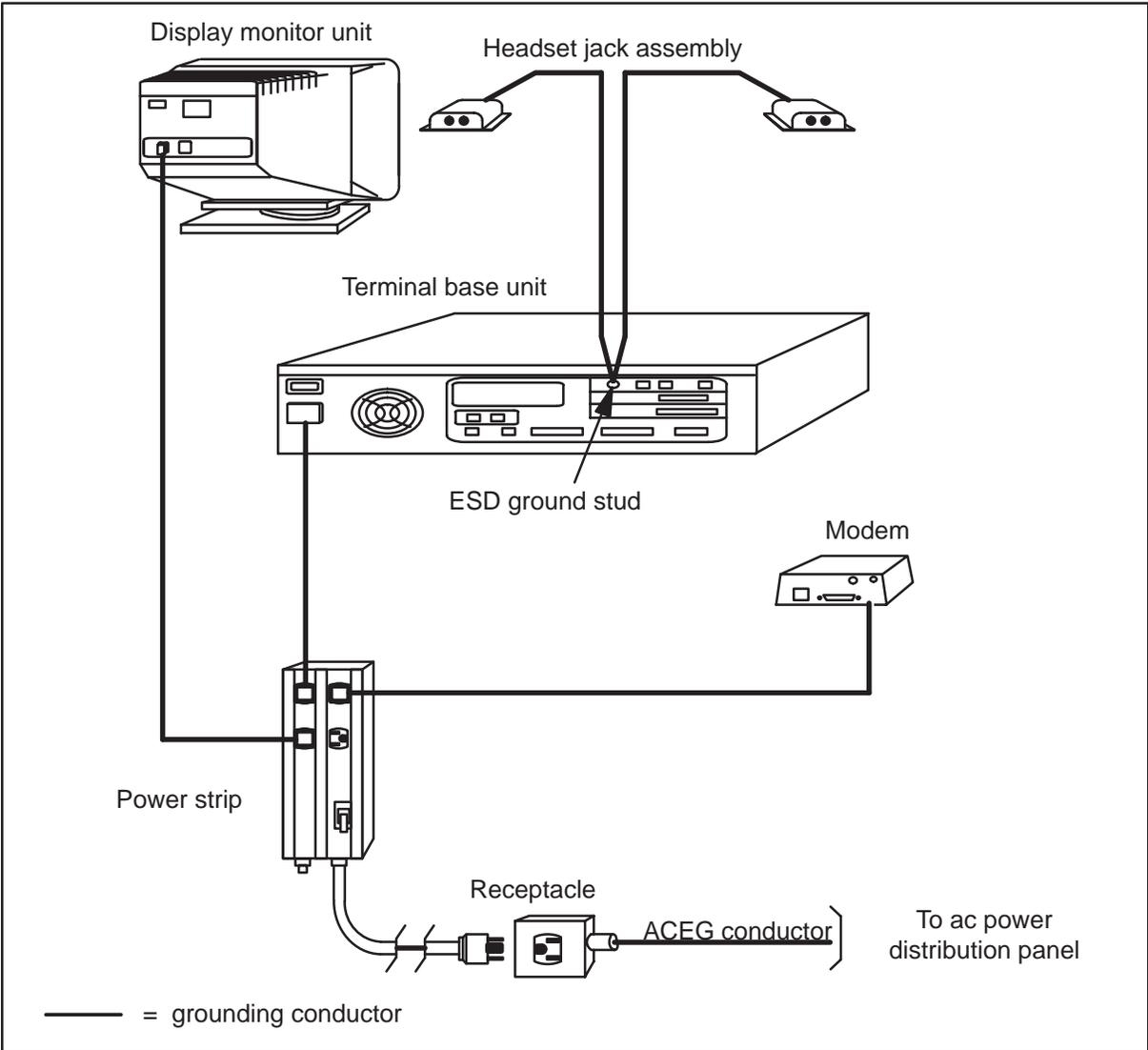
An ESD ground stud on the digital telephony card located in the terminal base unit is used to connect the ESD ground straps of the two headset jack assemblies. If required by the operating company, this ESD ground stud may also be bonded to a nearby ground reference (such as a floor ground grid) of the building grounding system.
