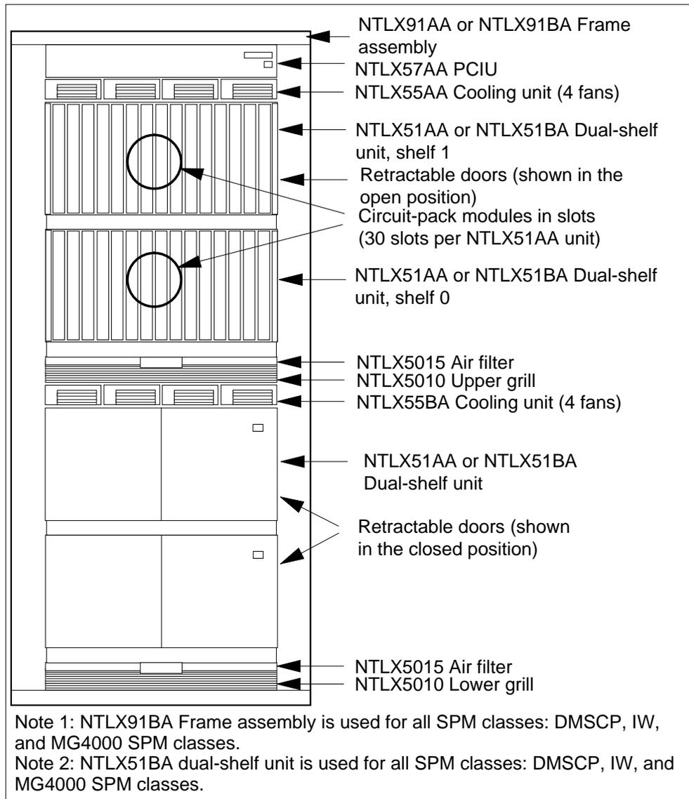
Each NTLX91AA or NTLX91BA frame assembly contains two NTLX55AA forced-air cooling units. Each NTLX55AA cooling unit contains four NTLX56AA fan assemblies to provide cooling air to the SPM modules. The NTLX57 PCIU serves as a central gathering point for all power and alarm cabling used within the NTLX91AA frame assembly. The following illustration shows the hierarchy of the major components of SPM.
