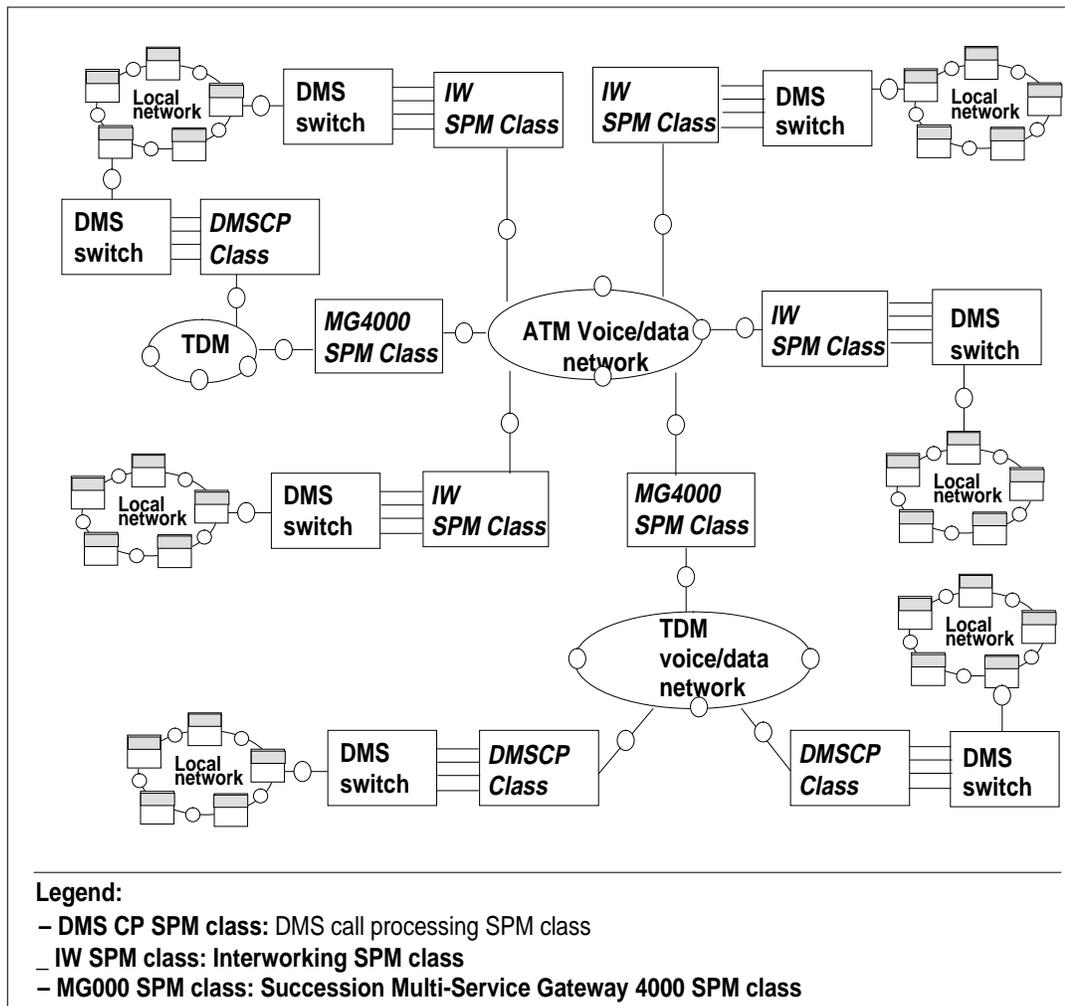
SPM nodes directly terminate an OC3 SONET carrier and feed the individual digital-signal-level-zero (DS-0) traffic from the carrier into the DMS switch.
