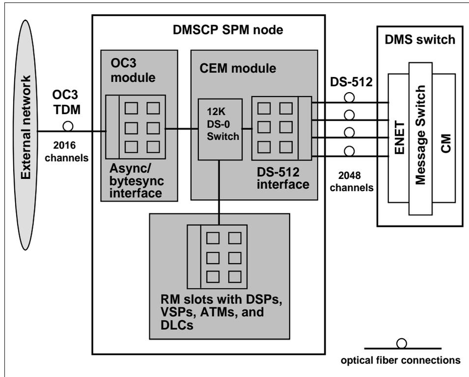
Figure 1-8 Various links of an IW SPM
