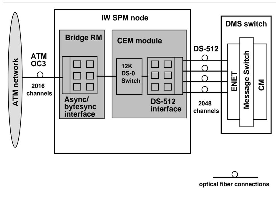
Figure 1-9 Various links of an MG4000 SPM
