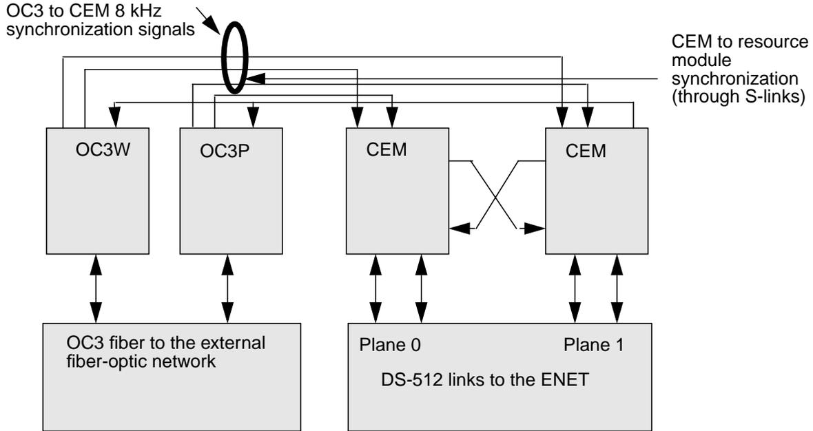
As shown in the previous figure, the CEMs form the center of a duplicated star topology and the CEMs provide the primary means of transmitting clock synchronization signals through the S-links. RMs derive their system-clock signal from the S-links to the active CEM.
