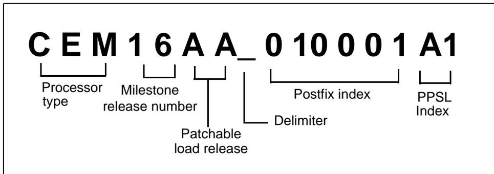
The table below, [SPM load file names for patchable loads](#), provides an explanation of the SPM patchable load file naming conventions.
