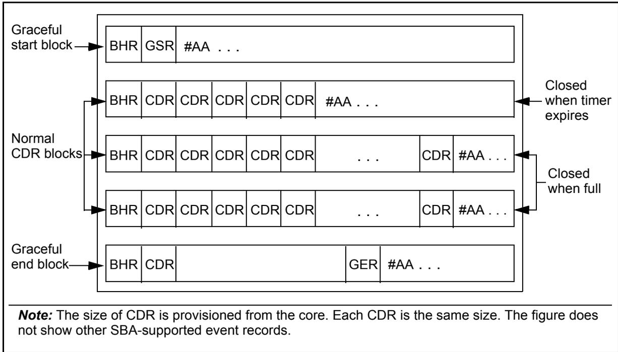
The following figure shows an example BAF DIRP file when SBA block flushing is activated.
