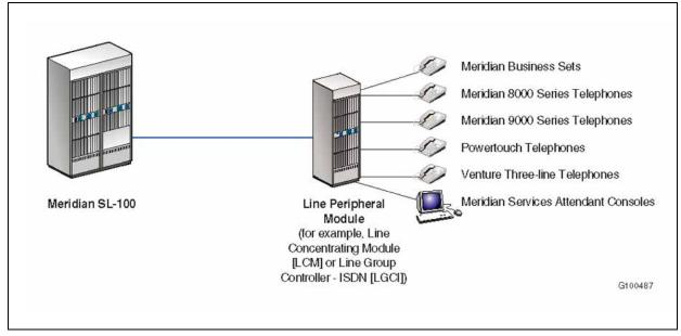
Supported Line Peripheral Module telephones can be broken down into the following families:
