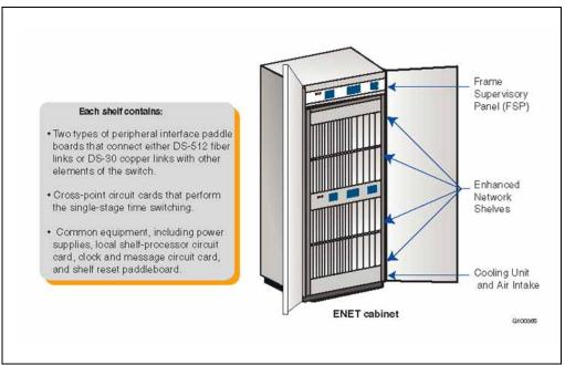
The Enhanced Network replaces the junctored network modules. It is a non-blocking, junctorless, single-stage time switch that can expand its capacity from 4k to 128k unidirectional channels. ENET is compatible with all Meridian SL-100 PMs, including the fiberized Series II PMs.
