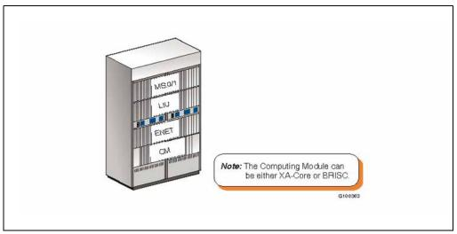
The Meridian SuperNode SE offering combines the functionality of the DMS-Core, DMS-Bus, 16K Enhanced Network (ENET) and a single-shelf Link Peripheral Processor (LPP) into one cabinet by providing the following:
