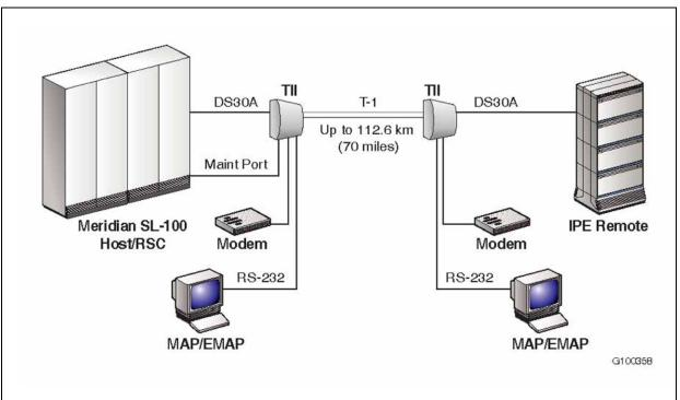
Figure 28 Remote T1 IPE Interface configuration
