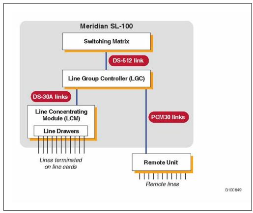
Figure 21 Line Group Controller links with other components
