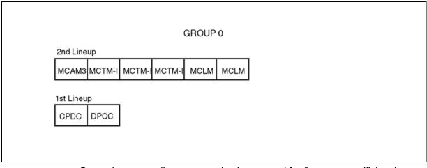
Secondary group lineups can also be merged for floor space efficiencies. Lineups 1 and 2 of a secondary group consisting of an MCAM3, MCTM-I, and MCLM can be merged into a single lineup as shown in Figure 70 "Secondary group merged into a single lineup" (page 145).
