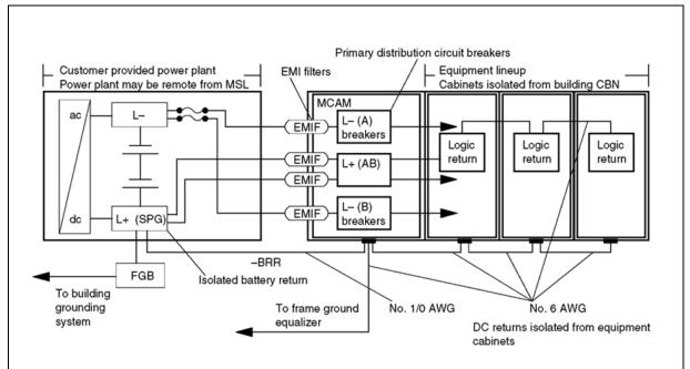
Figure 34 "Frame ground and battery return connections" (page 89) shows the frame ground and battery return connections between lineups. The frame ground connections connect the frames of each lineup to the frame grounding reference, a single point ground. The battery return connections connect the A-feed battery return to the B-feed battery return in alternate lineups to ensure battery return equalization among lineups.
