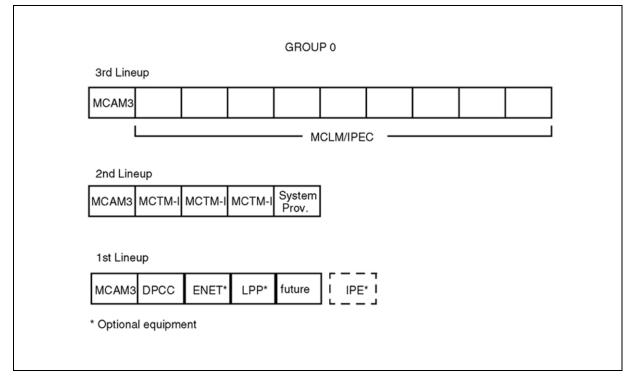
The second lineup of the primary group for a full-size SuperNode system consists of the Meridian Cabinet Auxiliary Module phase 3 (MCAM3), followed by three Meridian Cabinet Trunk Module-ISDN (MCTM-I) cabinets and a system provisionable cabinet.
