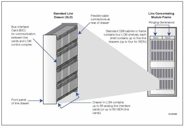
Depending on the level of concentration required, there can be from two to six 2 Mbps links between a Line Group Controller and Line Concentrating Module (up to 18 for an ISDN-enabled LCME). Each Line Group Controller has a theoretical maximum of 20 ports for 2 Mbps Line Concentrating Module links. Given the maximum of 2 Mbps links per Line Concentrating Module, a Line Group Controller can theoretically support up to 10 Line Concentrating Modules.
