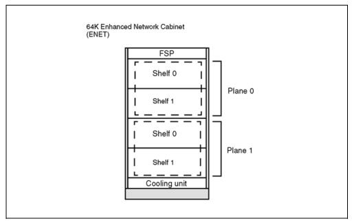
Figure 45 64K single-cabinet ENET components
