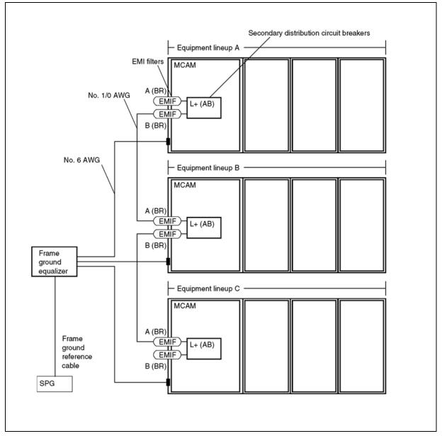
Figure 35 "Star-IBN frame grounding configuration" (page 90) shows the grounding plan that provides each frame with an individual connection to the Frame Ground Equalizer (FGE). The FGE is connected to the SPG with a single connection. In this grounding system, an individual ground cable is run from the SPG to the frame ground stud on the MCAM in each lineup. Within the individual lineups, the ground cable is daisy chained from the MCAM to each cabinet in the lineup.
