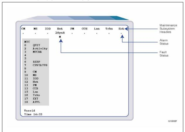
A dot beneath a header indicates that the status of the subsystem is satisfactory. Any other code indicates that an out-of-service or alarm condition exists.
