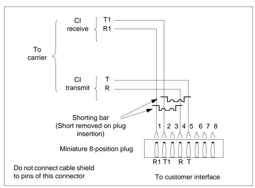
Figure 2-10 Connector pin assignment (RJ48X)
