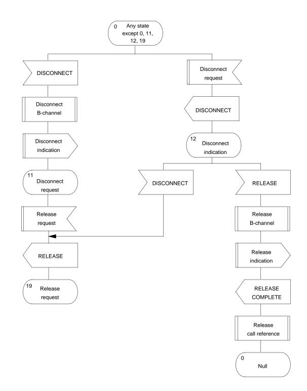
Figure 4-43 Overview protocol control: Network side (5 of 6) Clearing procedure (1 of 2)
