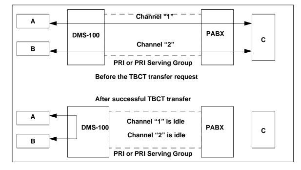
Figure 5-1 Two B-Channel Transfer
