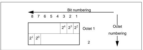
An exception to the preceding field mapping convention is the data-link-layer frame check sequence (FCS) field, which spans two octets. In this case, bit 1 of the first octet is the high order bit and bit 8 of the second octet is the low order bit (see Figure 3-5).
