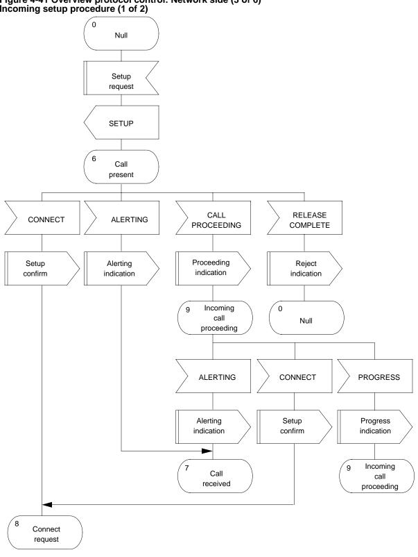
Figure 4-41 Overview protocol control: Network side (3 of 6) Incoming setup procedure (1 of 2)
