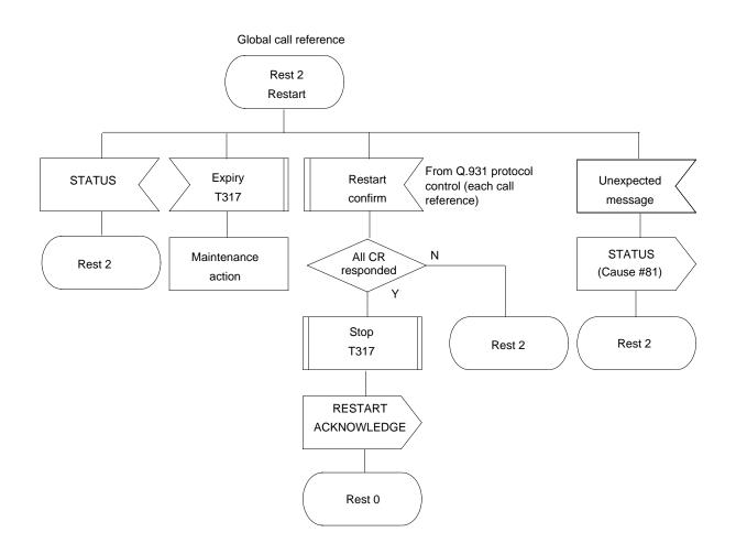
Figure 4-39 Overview protocol control: Network side (1 of 6) Outgoing setup procedure (1 of 2)
