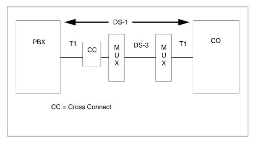
Figure 2-2 Network view of ISDN PRI functionality
