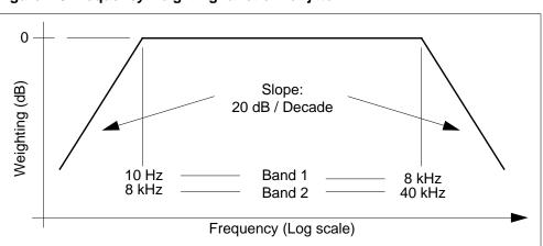
Figure 2-6 Frequency weighting function for jitter
