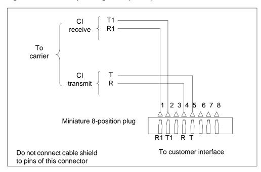
Figure 2-9 Connector pin assignment (RJ48C)
