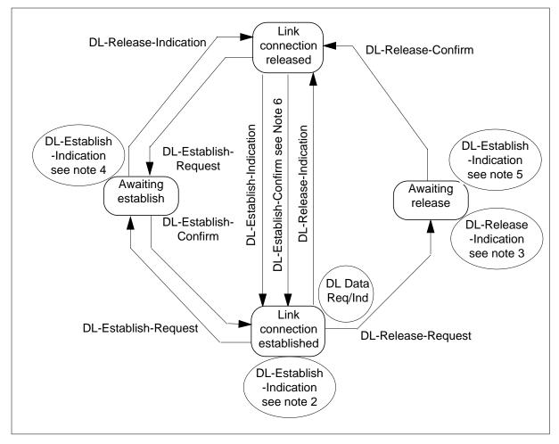
*Note 1:* If the data link layer entity issues a *DL-Establish-Indication* primitive, (for instance, if the data link layer is initiated or the peer system initiated re-establishment), a *DL-Release-Confirm* primitive, or a *DL-Release-Indication* primitive, all the data link service data units representing *DL-Data-Requests* are discarded.
