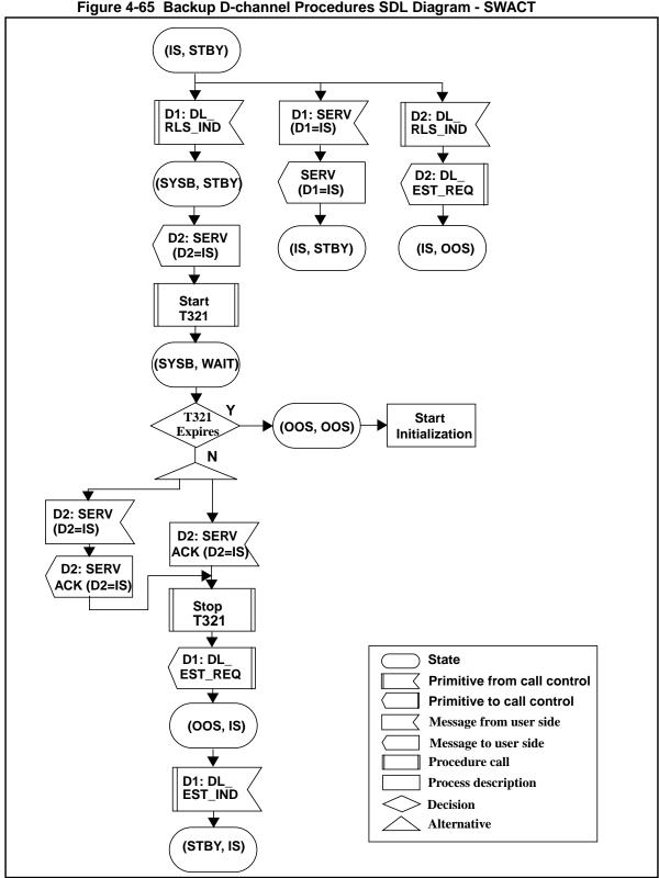
Figure 4-65 Backup D-channel Procedures SDL Diagram - SWACT
