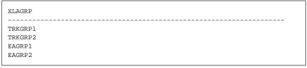
The XLAGRP of TRKGRP1 is defined for trunk group TQMSOSSIC1, and the XLAGRP of TRKGRP2 is defined for trunk group TQMSOSSIC2. Trunk group TQMSOSSIC3 reuses the XLAGRP of TRKGRP1.
