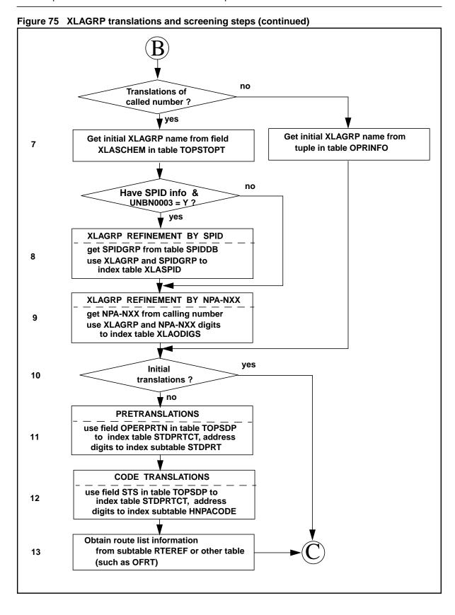
7 If translations is being performed for called number, the initial XLAGRP for the originating trunk group is obtained from field XLASCHEM in table TOPSTOPT.
