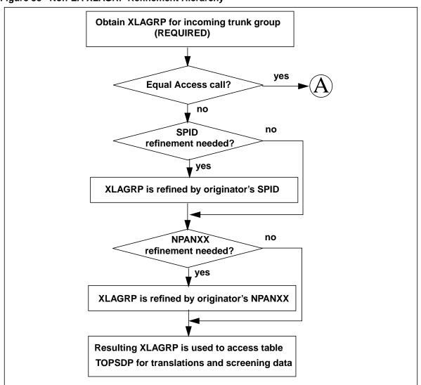
This figure shows the logic flow used to arrive at the XLAGRP used for translations and screening for Equal Access (EA) calls.
