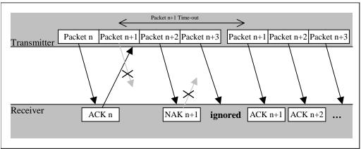
FIGURE 6.5 – "NAK PACKET LOST" TIME-OUT SCENARIO
