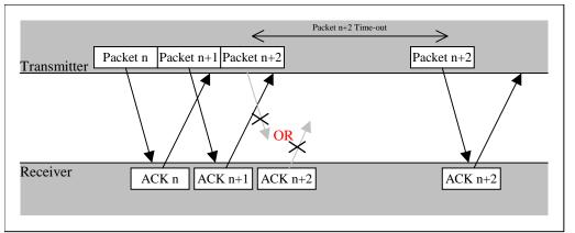
FIGURE 5.6 - "Last packet lost" time-out scenario
