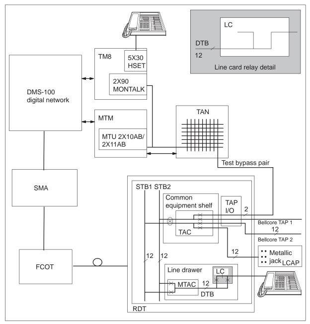
The MONLTA command uses test configuration 8 when the ICM option is equipped. The subscriber line connects through a PCM path through the network to another subscriber line or an interoffice trunk. The subscriber line connects through a digital bridge in the IMC, to a PCM path that terminates on the HSET. The HSET resides in the trunk module (TM). In this configuration, monitor an active S/DMS AccessNode circuit from a telephone that connects to a HSET.
