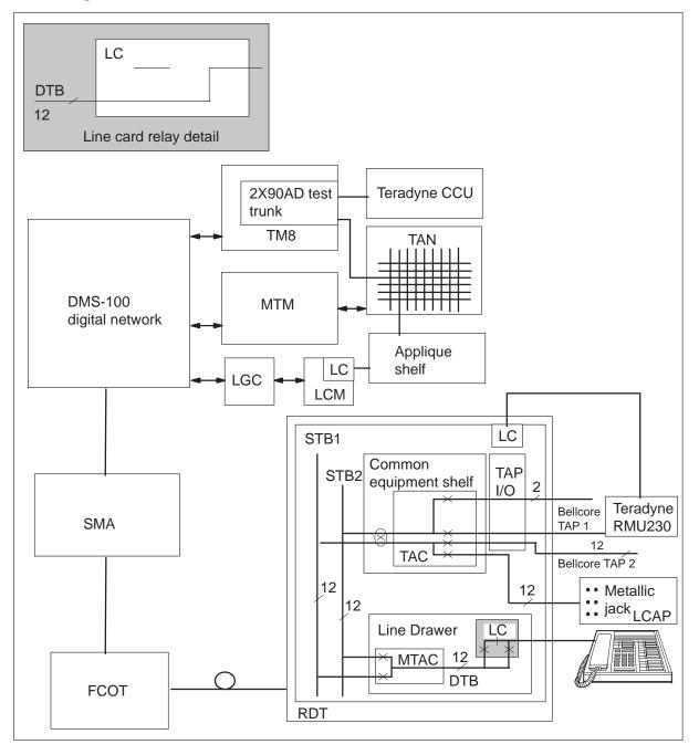
The Teradyne computer control unit (CCU) uses a path that the following links form to control the RMU230:
