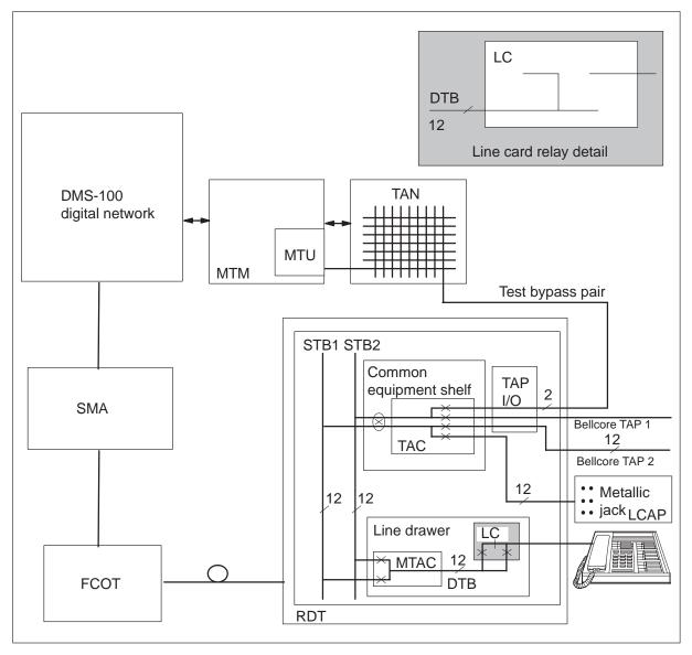
The MONLTA command uses test configuration 7 when the IMC option is not equipped. The subscriber line connects through a PCM path through the network to another subscriber line or interoffice trunk. The subscriber line is bridged to a metallic bypass pair. The subscriber line connects to the 101 communication test line (HSET) circuit through an intermediate test 2X90 trunk.
