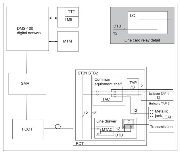
The JACK command uses test configuration 5. The subscriber line connects through a PCM path through the network to the jack-ended trunk. The jack-ended trunk allows external test equipment to connect to the circuit.
