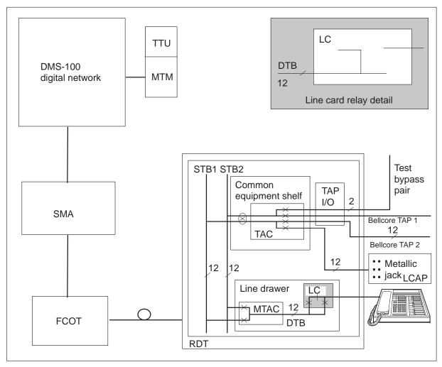
The LNTST, LIT, VDC, VAC, RES, and CAP commands use test configuration 2 when the IRTU option is not equipped. The S/DMS AccessNode line card disconnects from the subscriber line. The S/DMS AccessNode connects the subscriber line to a metallic bypass pair. This pair connects to the multi-line test unit (MTU) through the test access network (TAN). In this configuration the MTU performs different electrical measurements on the bypass pair and subscriber line.
