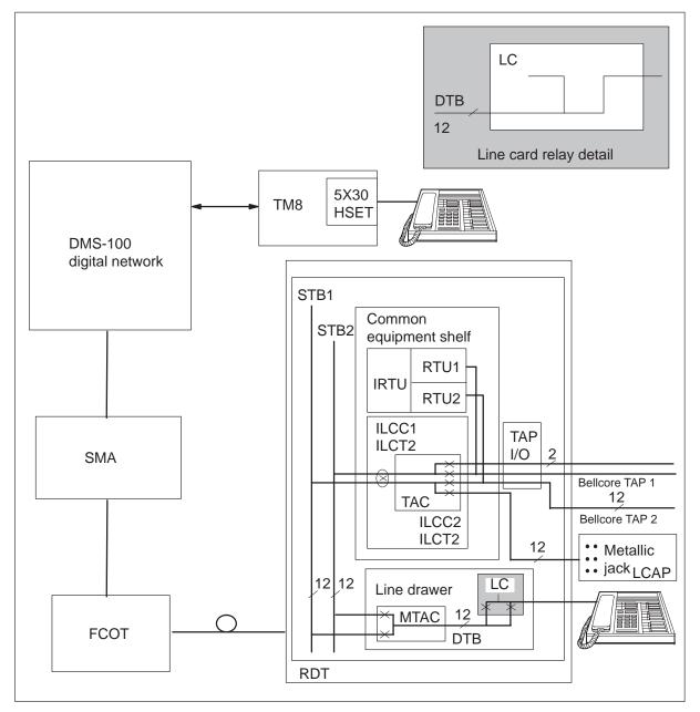
The ORIG command uses test configuration 9 when the IMC option is equipped. The subscriber line disconnects from the S/DMS AccessNode line card. The S/DMS AccessNode line card connects to a metallic bypass pair. The bypass pair connects to the MTU through the TAN. The bypass pair connects to the HSET through an intermediate 2X90 test trunk.
