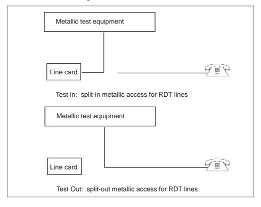
Test-in and test-out configurations for RDT lines
