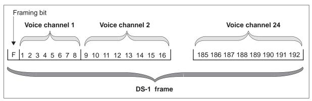
The framing bit identifies the location of the first time slot in the frame. When the RDT or SMA receives a framing bit, the RDT or SMA is notified that the following 8 bits contain information from time slot one. The framing bit can also perform frame alignment in the extended superframe alignment.
