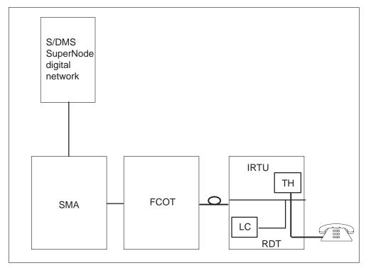
This diagram is the test configuration for the SDIAG command that supports POTS and coin lines. The EBS lines are not tested because a test can cause a loss of battery on the loop.
