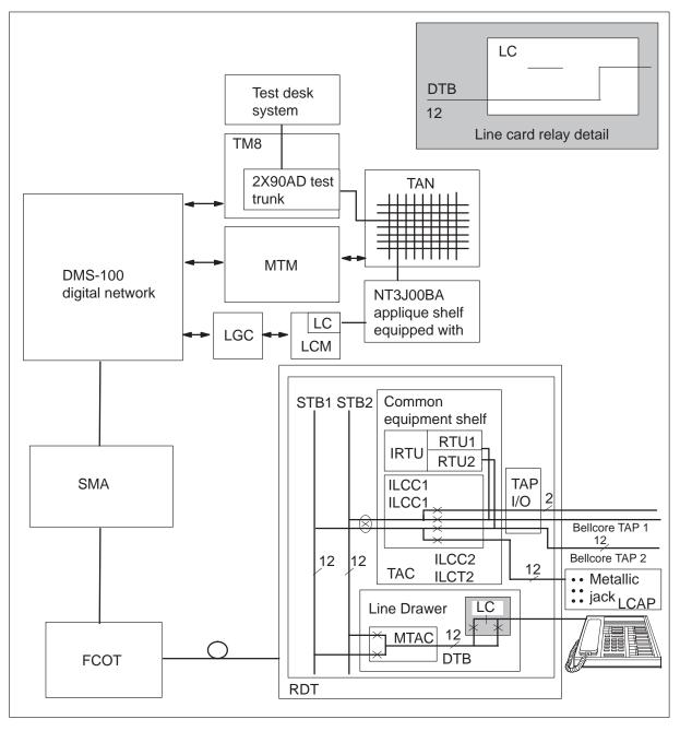
The mechanized loop tester (MLT) uses test configuration 18 when the RMU option is not equipped. The S/DMS AccessNode line card disconnects from the subscriber line.
