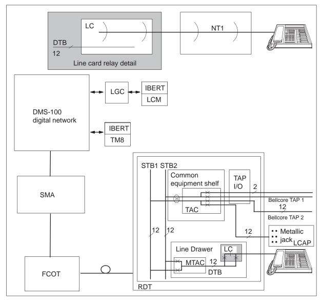
The DCHCON command uses test configuration 26. The D-channel on the subscriber line loops back in the S/DMS AccessNode or NT1. The number, location, and type of loopback points in the S/DMS AccessNode must be determined. The NT1 loopback consist of a 2B+D loopback. The CM instructs the DCH to insert a test message in the looped back D-channel. In this test configuration, the CM originates the test request message.
