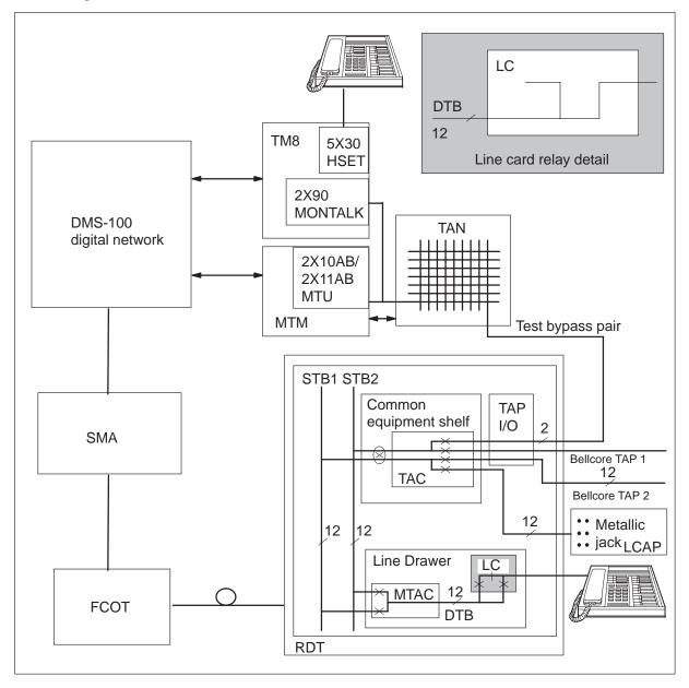
Silent switchman tests use test configuration 12. The S/DMS AccessNode line card disconnects from the subscriber line.
