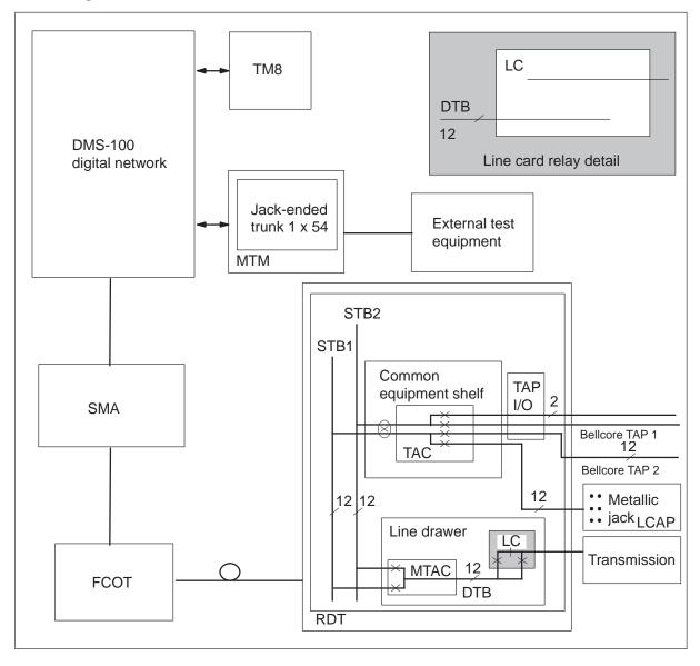
The TSTRING command uses test configuration 6. The subscriber line disconnects from the S/DMS AccessNode line card. The S/DMS AccessNode line card connects to the test access card (TAC). The TAC detects ringing voltage that the line card applies when TSTRING is implemented.
