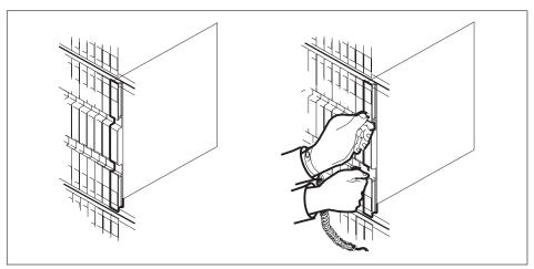
**3** Open the locking levers on the faulty card. The top locking lever opens up and the bottom locking lever opens down.
