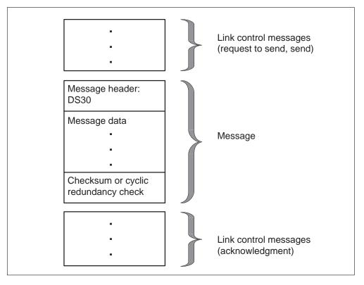
Message time-out, message checksum, or CRC calculation performs message error detection. In the event of protocol, checksum, or CRC failure on an outgoing message, the sending node tries the send sequence again.
