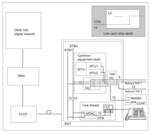
The LOSS, NOISE, and TONEGEN commands use test figure 4. The subscriber line connects through a PCM path through the network to the termination test trunk (TTT). The transmission test set consists of portable test equipment that can generate and measure voice frequency signals. This figure does not intend a specified brand of test equipment.
