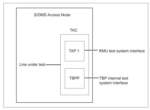
Operating company personnel want both internal (MAP terminal) and external testing through IRTU. The two IRTU test heads and four current line appearances for ILCs are assigned. Table entries for the fields that this feature affects are as follows. The following illustrates this setup.
