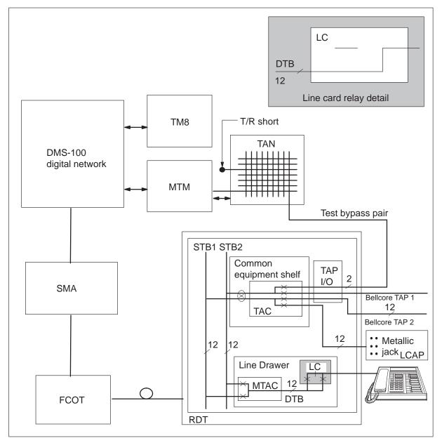
The dialable short circuit test uses test configuration 15 when the IMC option is equipped. The S/DMS AccessNode line card disconnects from the subscriber line. The subscriber line connects through the S/DMS AccessNode to a shorting termination in the IMC card.
