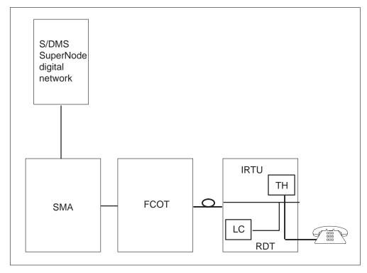
The DIALABLE SHORT CIRCUIT command uses this configuration when the IRTU is available. The S/DMS AccessNode line card disconnects from the subscriber loop. The S/DMS AccessNode connects the subscriber loop to the IRTU test head. In this configuration the IRTU test head provides a short across the tip and ring leads of the subscriber loop. Plain ordinary telephone service (POTS), COIN, and Meridian business set (MBS) lines use dialable short circuit.
