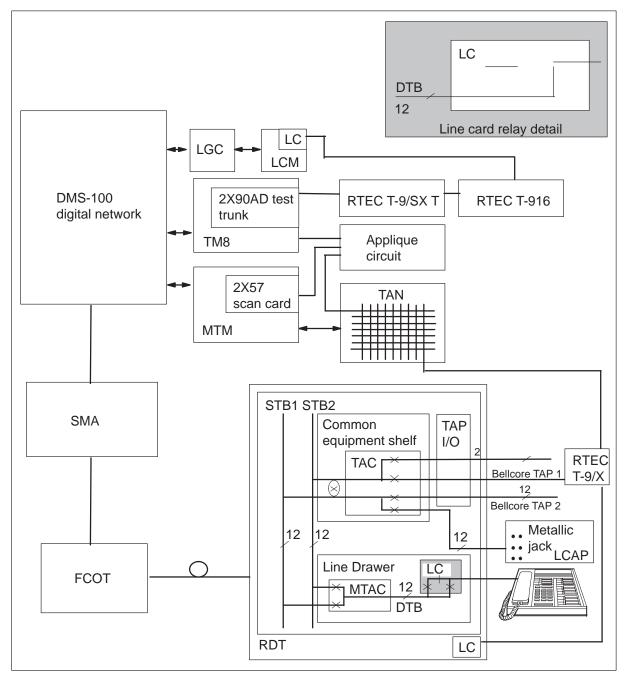
Teradyne uses test configuration 21. The S/DMS AccessNode line card disconnects from the subscriber line. The subscriber line connects through the S/DMS AccessNode to the RMU230. The RMU230 performs electrical measurements on the subscriber line.
