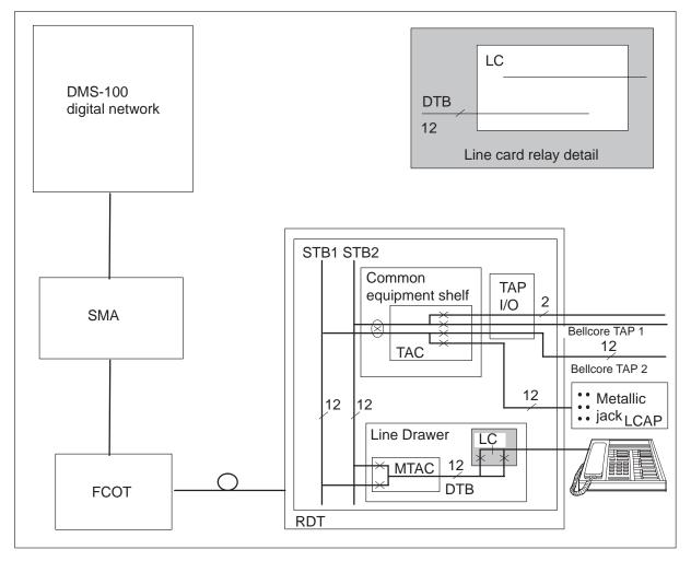
The dialable short circuit test uses test configuration 14 when the IMC option is not equipped. The S/DMS AccessNode line card disconnects from the subscriber line. The subscriber line connects through the S/DMS AccessNode to a metallic bypass pair through the S/DMS AccessNode. The bypass pair connects to a shorting termination through the TAN. This test requires the MTM because the TAN contains the interface to control the TAN.
