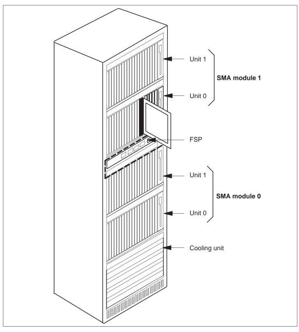
Two to ten DS-1 interface cards, are distributed across the shelves of an SMA module. These cards provide a maximum of 20 DS-1 ports. The DS-1 ports service DS-1 links to S/DMS AccessNode fiber central office terminals (FCOTs). The SMA provides an interface for ISDN through the Enhanced D-channel handler (EDCH) circuit card.
