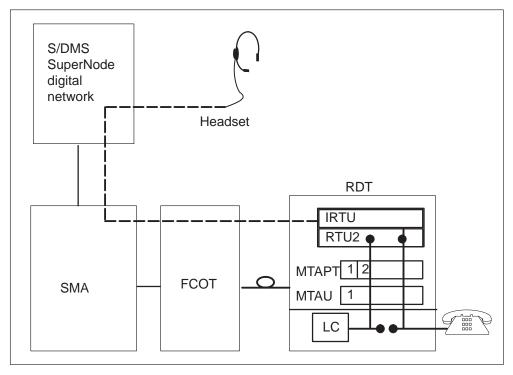
The TONEGEN METALLIC command uses this test configuration when the IRTU is available. The S/DMS AccessNode line card is disconnected from the subscriber loop. The S/DMS AccessNode connects the subscriber loop to the IRTU test head. In this configuration the IRTU test head provides tones on the subscriber loop.
