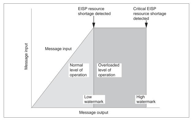
When operation reaches the *low watermark* for resource congestion, the EISP enters the overloaded level of operation. Logical links on the EOC are placed in the receiver-not-ready (RNR) state. The exception is the logical link used for protection switch control. This action reduces the number of incoming messages.
