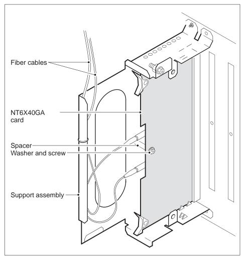
**21** Using the levers located at the top and bottom of the 6X40 card, remove the card from the support assembly by firmly pulling horizontally until the connector pin socket on the card has cleared the connector pins on the backplane.
