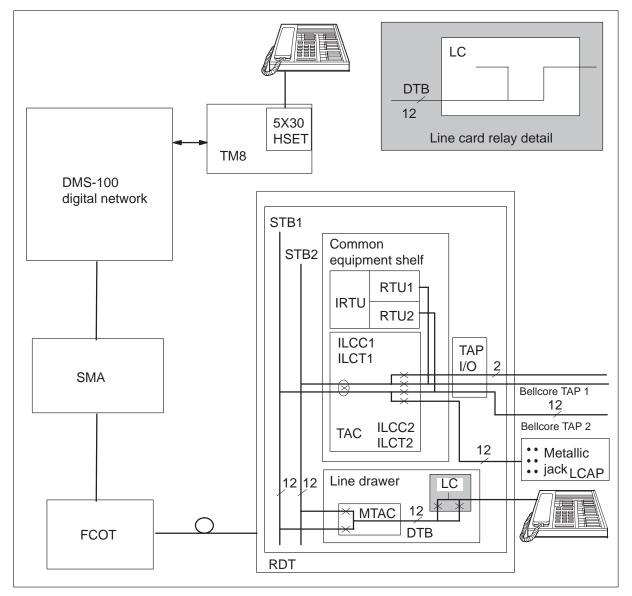
The TALKLTA, COIN, RING, and DGTTST tests use test configuration 11 when the IMC card is not equipped. The subscriber line connects through a PCM path, through the network to the HSET through the MONTALK circuit.
