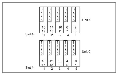
14 If the NT6X50 to be replaced is connected to IDT message links, then the appropriate message channels (CSC and EOC) must be busied.
