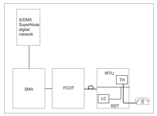
The ALT LIT command uses this test configuration when the IRTU is available. The S/DMS AccessNode line card disconnects from the subscriber loop. The S/DMS AccessNode connects the subscriber loop to the IRTU test head. In this configuration the IRTU test head performs DC, AC, RES, and CAP measurements on the subscriber loop.
