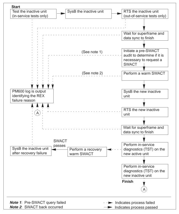
If a REX test fails, the system generates a PM600 log. The PM600 log initiates a major alarm for the XPM that failed the REX test. The major alarm appears at the MAP terminal under the PM banner at the top of the display.
