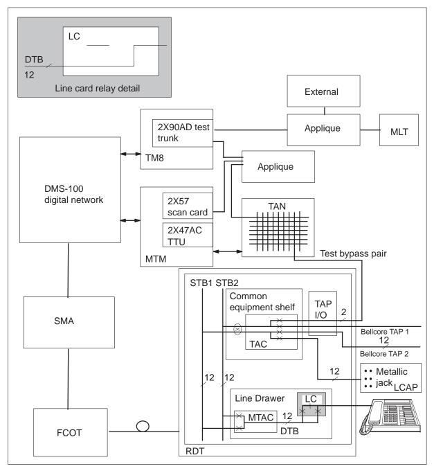
The subscriber line connects to the MLT through a metallic path. The links used to form the path are as follows:
