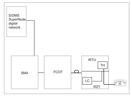
The test configuration for the TSTRING command when the IRTU is available is as follows. The S/DMS AccessNode line card is disconnected from the subscriber loop. The LTA direction is inward. The S/DMS AccessNode connects the line card to the IRTU test head. In this configuration the IRTU test head detects ringing voltage that the line card applies.
