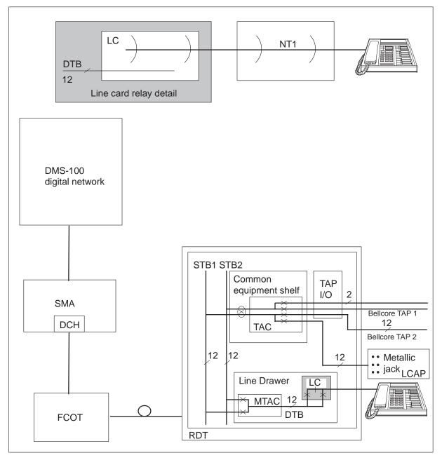
The BERP command uses test configuration 25. A system establishes loopback point in the SMA, S/DMS AccessNode, or NT1 through the LOOPBACK command. The IBERT card inserts a continuous test pattern. This pattern passes to the loopback point and is reflected back. The IBERT card monitors the returning signal and maintains statistics that reflect signal quality.
