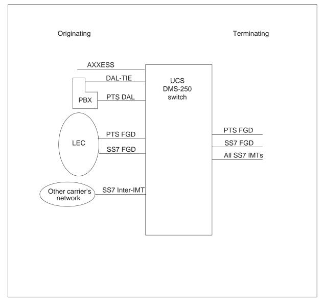
*Note:* The originating side of the UCS DMS-250 switch shows the trunk groups which support CIC Routing, while the terminating side shows the trunk groups which support CIC delivery.
