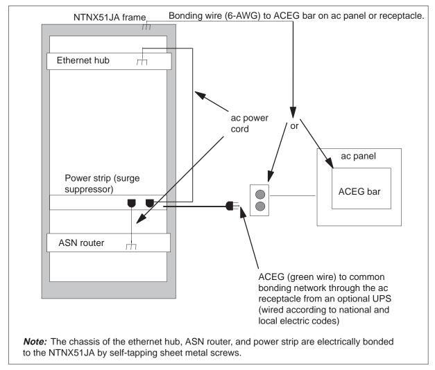
The following requirements apply to the frame installation:
