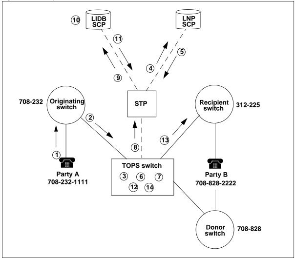
Figure 31 Example flow for collect call LIDB validation
