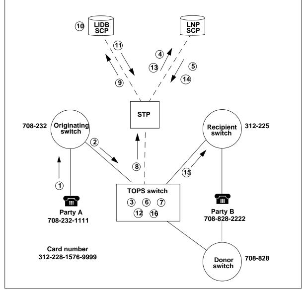
Figure 32 Example flow for calling card LIDB validation
