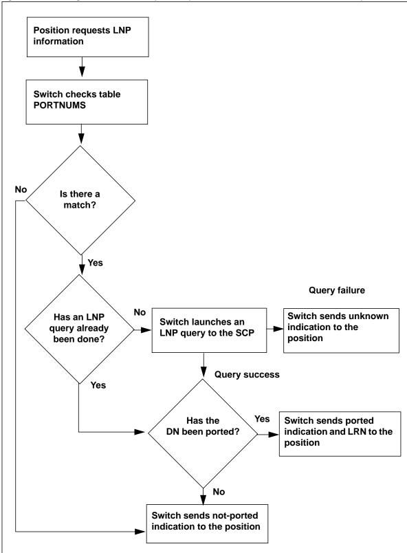
Figure 34 Message flow between operator position and TOPS switch in an LNP request
