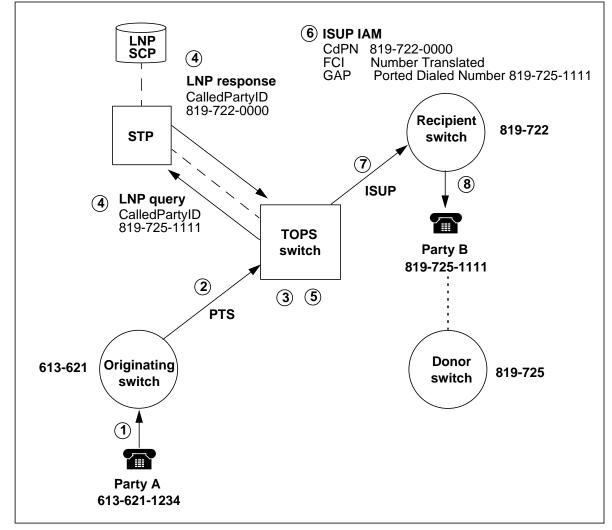
Figure 15 Example signaling flow for outgoing ISUP without SPN
