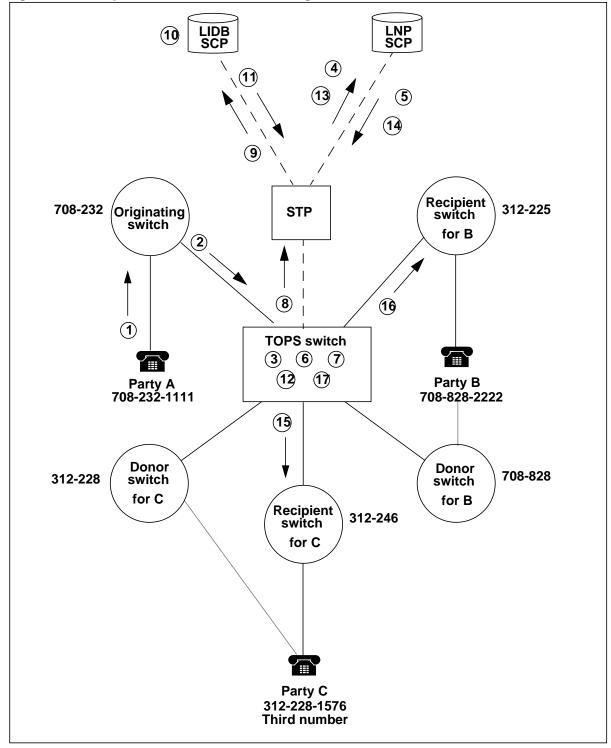
Figure 33 Example flow for third number billing LIDB validation
