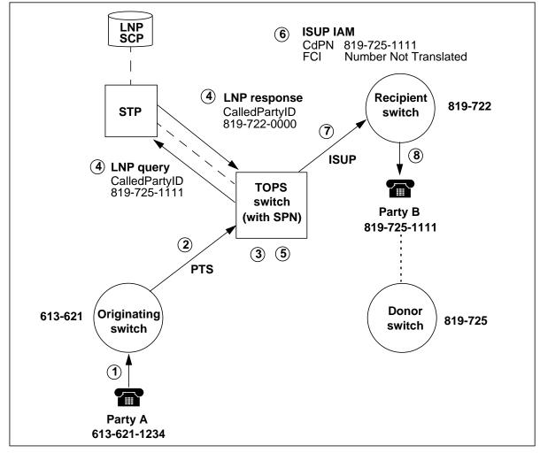
Figure 16 Example signaling flow for outgoing ISUP with SPN
