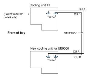
The BIP-to-cooling unit (CU) wiring harness is factory installed on the left side of the bay. To add a CU for use with the UE9000, you must install power harness NTNP85AA on the right side of the bay, between the first CU and the new CU.
