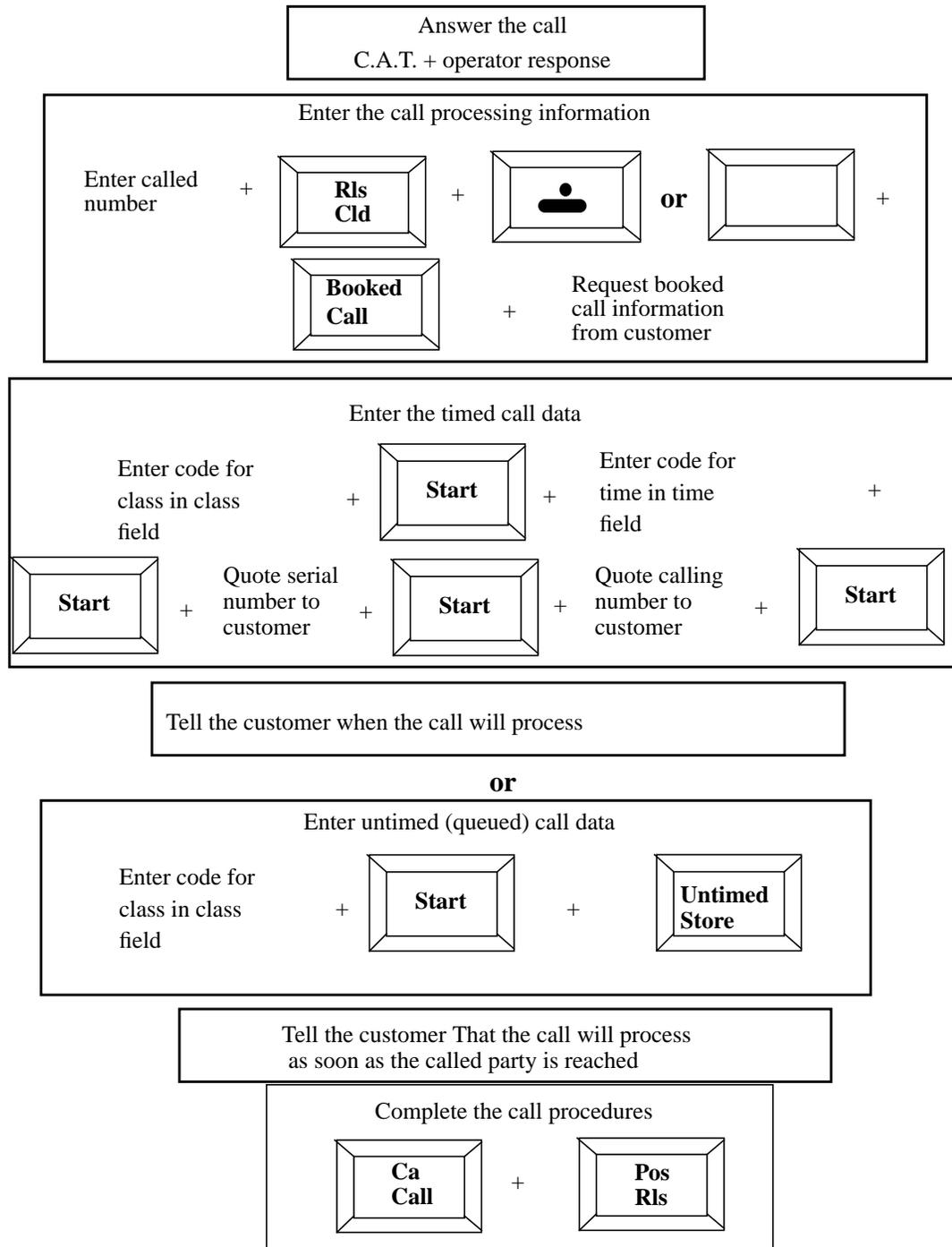
**Figure 179. Automatic booked call retrieval processing procedures**
