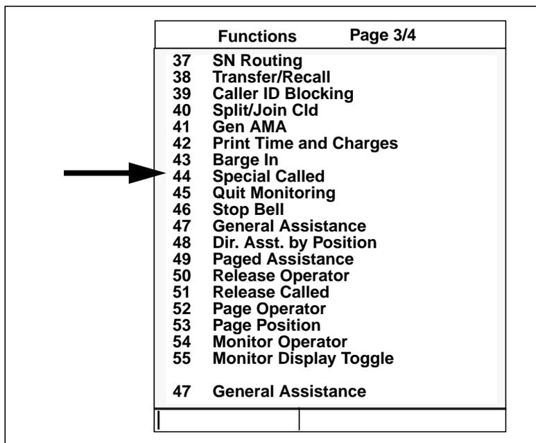
In this example, the operator types **43** and presses the **Start** key to barge in on the line.
