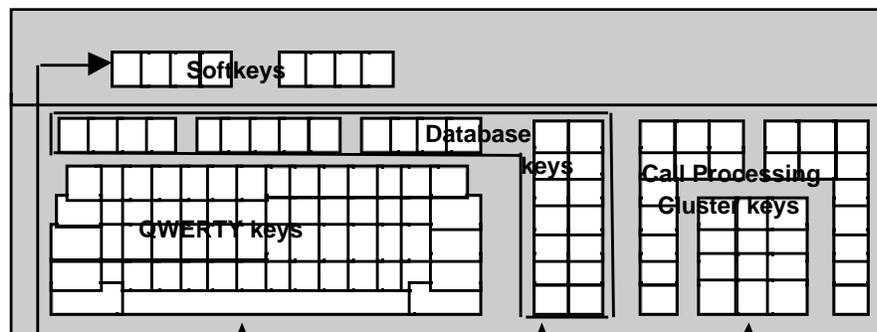
The keyboard comes with a default set of general functions, key names for those functions, and locations for keys. However, keyboard functionality is customizable. Each operating company can designate other TOPS IWS functions and define keys for those functions. Operating companies can also change the key names and locations of general functions.
