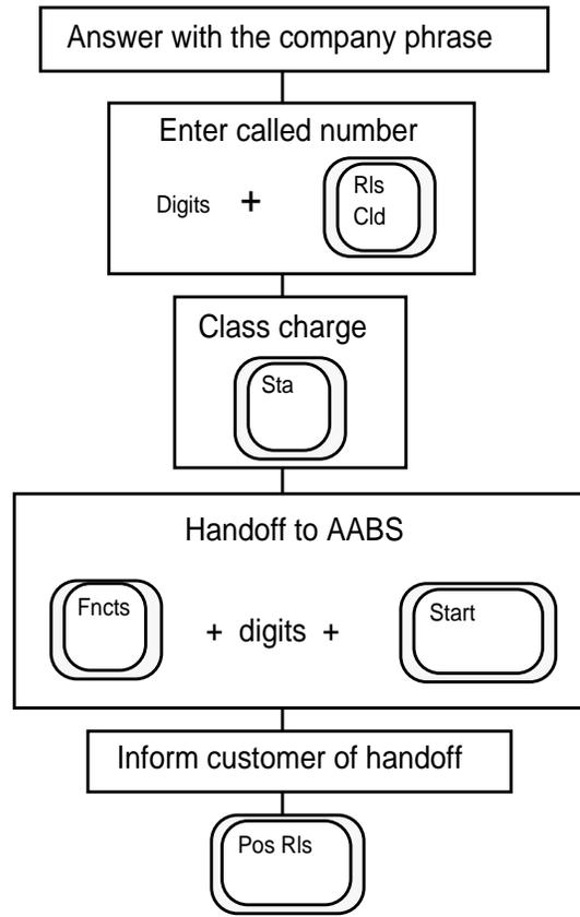
AABS provides operator assistance without the use of live operators, which reduces operator handling time of calls. AABS automates completion of calling card calls with the use of a voice service node (VSN). AABS also automates station collect and third number billing calls by using voice recognition technology and prompt generation to communicate with the billed party.
