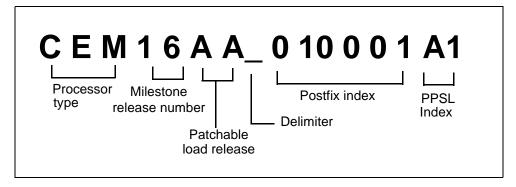
The table below, <u>SPM load file names for patchable loads</u>, provides an explanation of the SPM patchable load file naming conventions.
