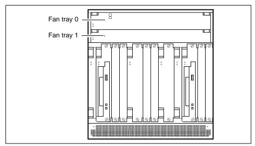
Two removable fan trays (NTRX50FE and NTRX50FF) provide horizontal (front-to-rear) cooling to the chassis. Both trays contain in-service and out-of-service LEDs.<sup>1</sup> The top tray (NTRX50FE) also contains system status LEDs. The following figure shows the fan trays and fan tray LEDs.
