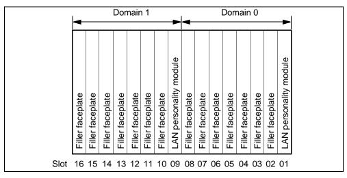
Provisionable personality modules in the I/O expansion chassis are not restricted to specific slot numbers. The LAN personality module mounts in any two slots. The slot numbers must match in each domain, and with the system module installed at the front of the chassis.
