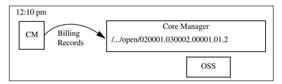
Assume the file is set up to close every 5 minutes. At 12:15 p.m. file 020001.030002.00001.01.2 is closed and moved to the "closedNotSent" subdirectory, as shown below:
