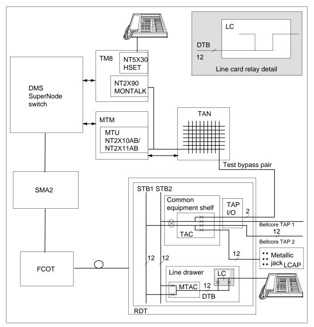
The MONLTA command uses test configuration 8 when the IMC option is equipped. A PCM path through the network connects the subscriber line to another subscriber line or an interoffice trunk. A digital bridge in the IMC connects the subscriber line to a PCM path that terminates on the HSET in the TM. In this configuration, a telephone that connects to an HSET allows operating company personnel to monitor an active S/DMS AccessNode circuit.
