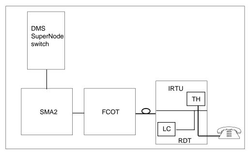
The following diagram shows the test configuration for the SDIAG command that supports POTS and COIN lines. Tests do not occur for EBS lines because this condition causes a battery loss on the loop.
