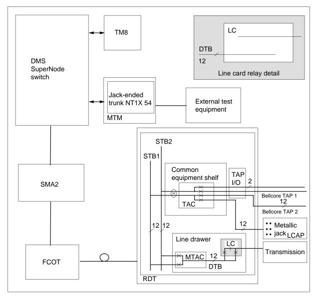
The TSTRING command uses test configuration 6. The system disconnects the subscriber line from the S/DMS AccessNode line card. The S/DMS AccessNode line card connects to the TAC. The TAC detects ringing voltage that the line card applies when the implementation of TSTRING occurs.
