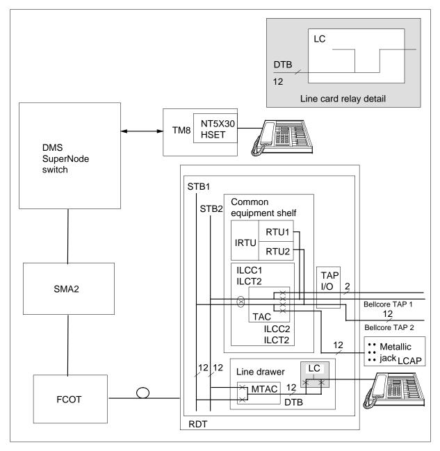
The ORIG command uses test configuration 9 when the IMC option is equipped. The system disconnects the subscriber line from the S/DMS AccessNode line card. The S/DMS AccessNode line card connects to a metallic bypass pair. The TAN connects the bypass pair to the MTU by the TAN. An intermediate NT2X90 test trunk connects the bypass pair to the HSET.
