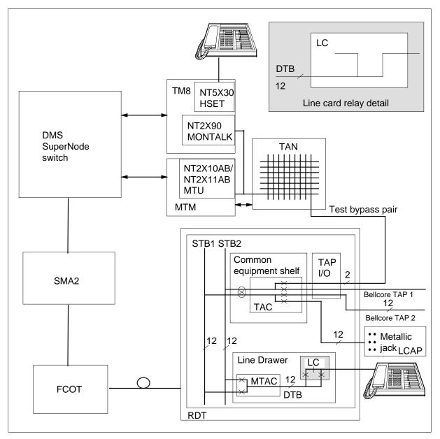
The silent switchman test uses test configuration 12. The system disconnects the S/DMS AccessNode line card from the subscriber line.
