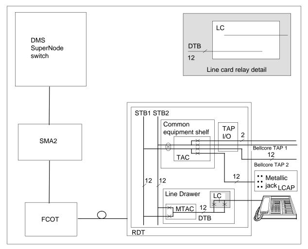
The dialable short circuit test uses test configuration 14 when the IMC option is not equipped. The system disconnects the S/DMS AccessNode line card from the subscriber line. The S/DMS AccessNode connects the subscriber line to a metallic bypass pair. The TAN connects the bypass pair to a termination that has a short circuit. The MTM contains the interface necessary to control the TAN.
