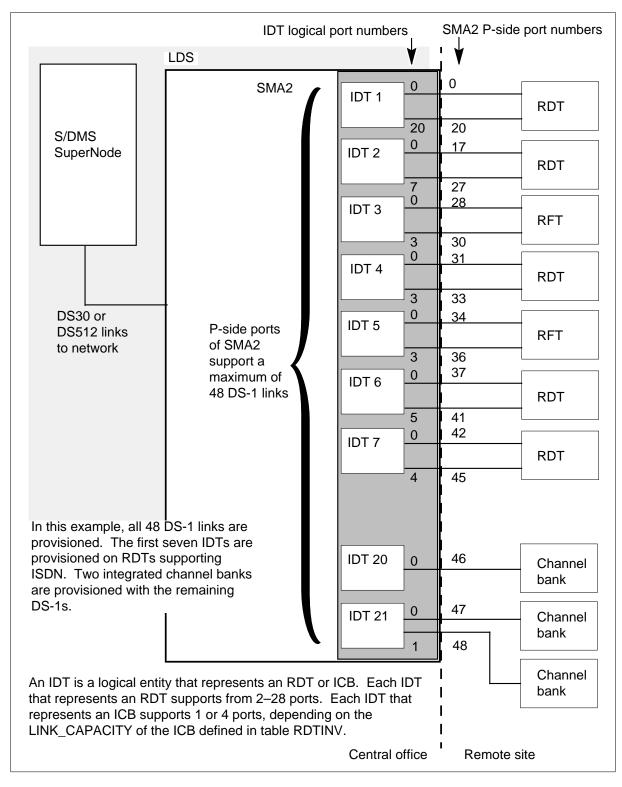
Figure 1-3 Example DS-1 links mapped to IDT ports
