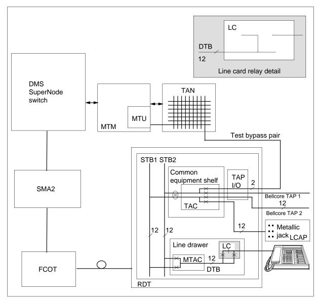
The MONLTA command uses test configuration 7 when the IMC option is not equipped. A PCM path through the network connects the subscriber line to another subscriber line or interoffice trunk. The intermediate test NT2X90 trunk bridges the subscriber line to a metallic bypass pair. Test NT2X90 trunk connects the line to the 101 communication test line (HSET) circuit.
