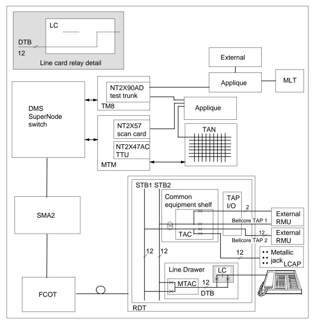
Reliance Telecommunication Electronics Inc. (RTEC) use test configuration 20. The system disconnects the S/DMS AccessNode line card from the
