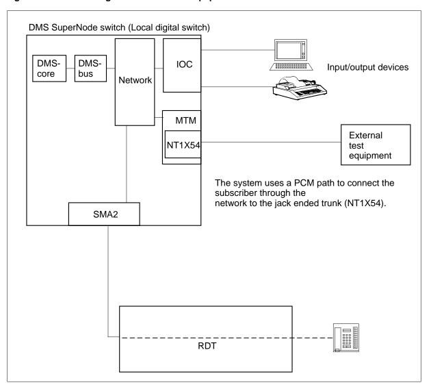
Figure 6-14 Line testing with external test equipment
