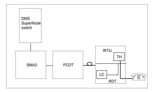
Figure 6-25 Test configuration for tonegen metallic
