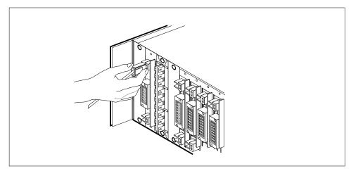
c Using the connector removal tool, manually disconnect the power connectors to the circuit card. Working from the bottom of the MSP shelf to the top of the MSP shelf, manually disconnect the smaller black power connectors located below the larger blue power connector. Manually disconnect the large blue power connector. Disconnect the smaller black
