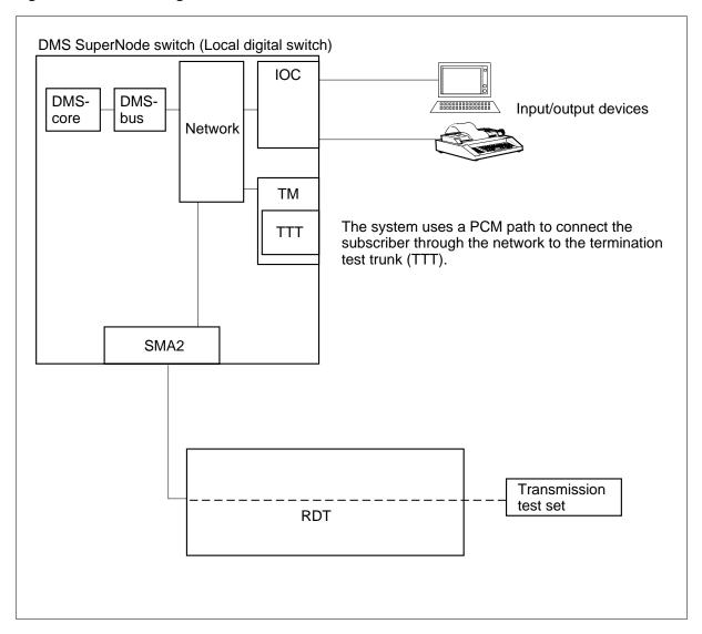
Figure 6-13 Line testing with a transmission test set
