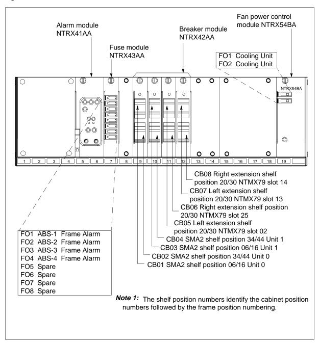
Figure 2-11 MSP shelf for SMA2 cabinet or frame with extension shelf in a CMVI and MVIE
