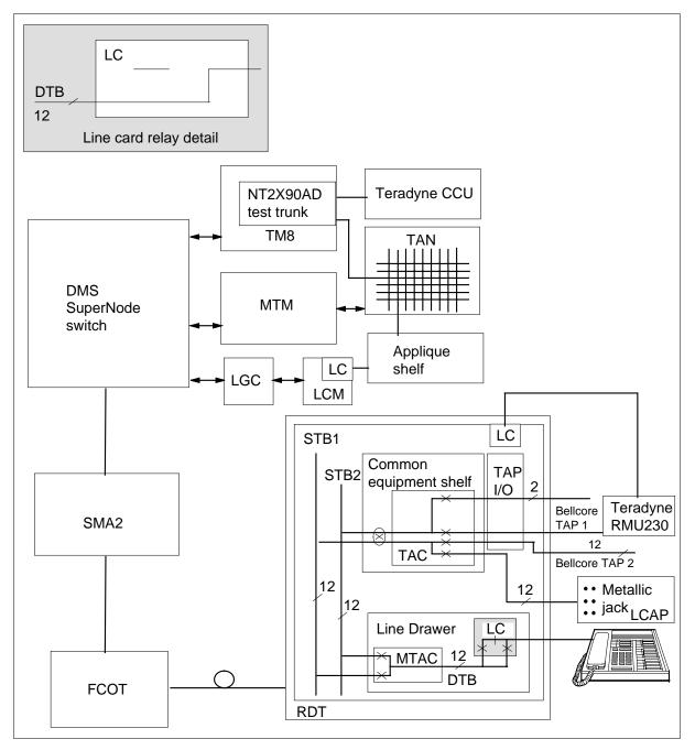
The BAL and BALNET commands use the test configuration 22. A PCM path through the network connects the subscriber line to the TTU. Now, the BAL and BALNET commands are not supported on S/DMS AccessNode lines.
