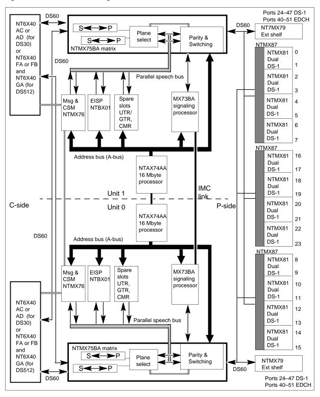
Figure 2-9 Functional block diagram of the SMA2
