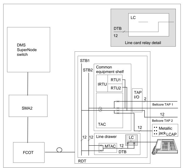
The local test cabinet number 13 and local test desk number 14, use test configuration 16. The 3703 local test cabinet uses this test configuration when the IMC option is not equipped. The TAN and the NT2X90 test trunk can connect the subscriber line or S/DMS AccessNode line card. The MTM contains the necessary interface to control the TAN.
