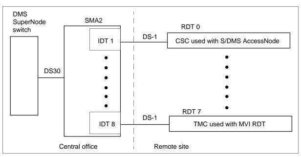
Figure 1-4 How the SMA2 supports different signaling types
