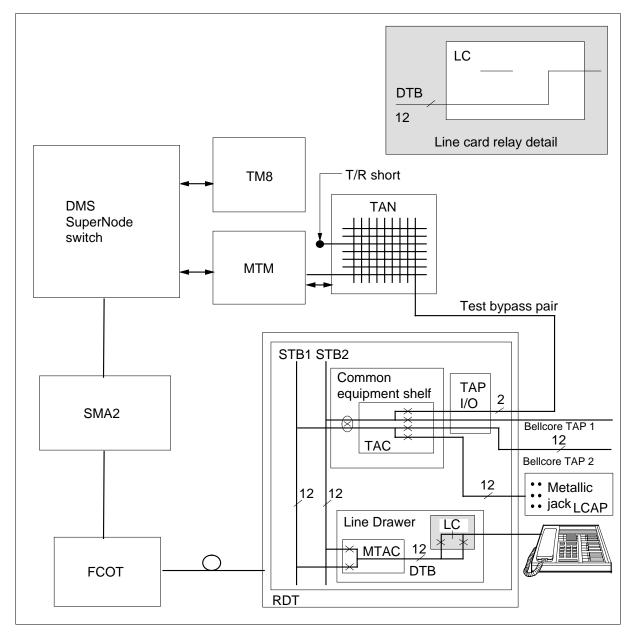
The dialable short circuit test uses test configuration 15 when the IMC option is equipped. The system disconnects the S/DMS AccessNode line card from the subscriber line. The S/DMS AccessNode connects the subscriber line to a termination that has a short circuit, in the IMC card.
