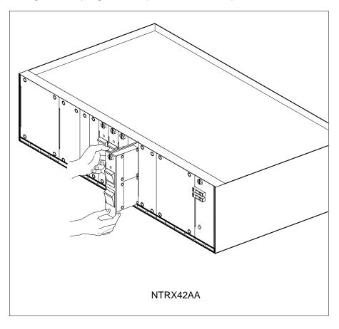
21 Replace any jumper connectors and cables removed in step 19. Reinsert the power connectors at the rear of the circuit card.
