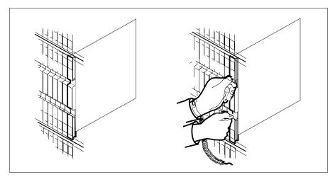
**3** Open the locking levers on the faulty card. The top locking lever opens up and the bottom locking lever opens down.
