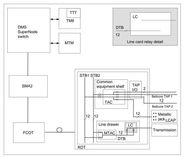
The JACK command uses test configuration 5. A PCM path through the network connects the subscriber line to the jack-ended trunk. The jack-ended trunk allows external test equipment connected to the circuit.
