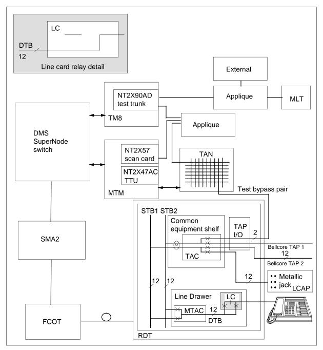
The MLT use test configuration 19 when the RMU option is equipped. The system disconnects the S/DMS AccessNode line card from the subscriber line. The S/DMS AccessNode connects the subscriber line to the RMU. The RMU performs electrical measurements on the subscriber line. Applique circuit 1 provides a DC signature to the MLT to indicate the tested line is on a remote access vehicle. The TAN maintains compatibility with current DMS-100 test
