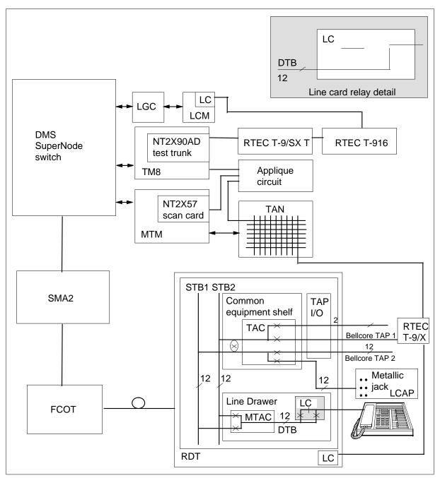
Teradyne uses test configuration 21. The system disconnects the S/DMS AccessNode line card from the subscriber line. The S/DMS AccessNode connects the subscriber line to the RMU230. The RMU230 performs electrical measurements on the subscriber line.
