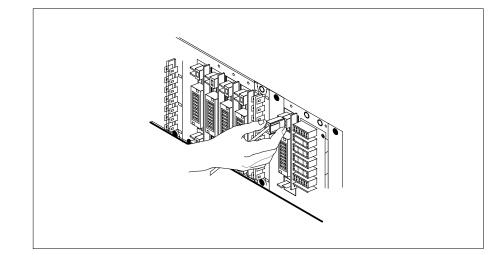
**10** Install the jumper connectors and cables removed in step 6 onto the replacement circuit card.
