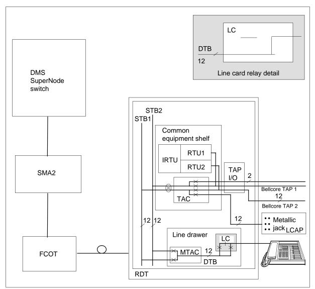
The LOSS, NOISE, and TONEGEN commands use test configuration 4. A PCM path through the network connects the subscriber line to the TTT. The transmission test set contains portable test equipment that can generate and measure voice frequency signals. This test configuration does not require a specified brand of test equipment.
