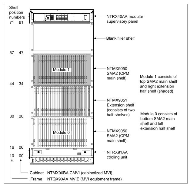
Figure 2-1 MVI cabinet and frame layout for the CMVI and MVIE (Cabinet is shown. Frame is like cabinet)
