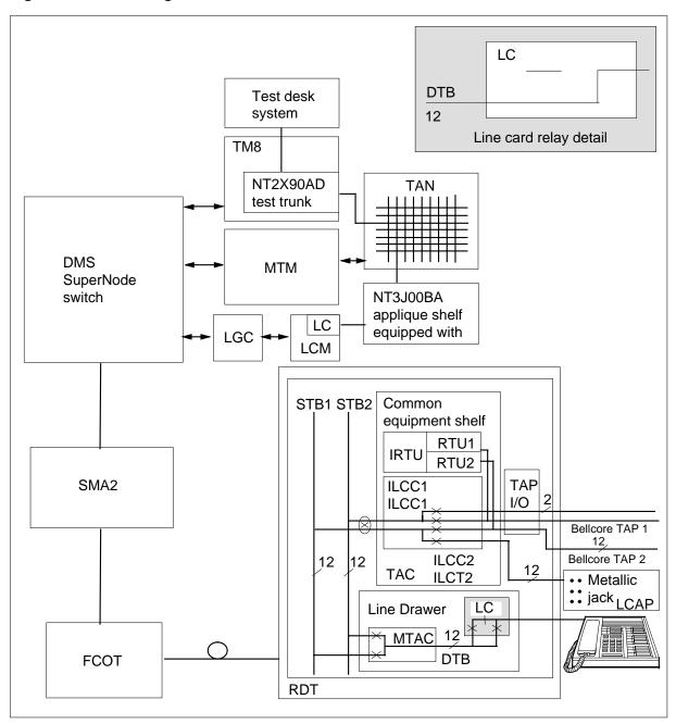
The mechanized loop tester (MLT) uses test configuration 18 when the RMU option is not equipped. The system disconnects the S/DMS AccessNode line card from the subscriber line.
