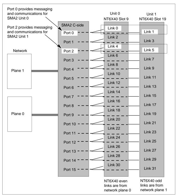
Figure 2-4 SMA2 C-side interface to the network
