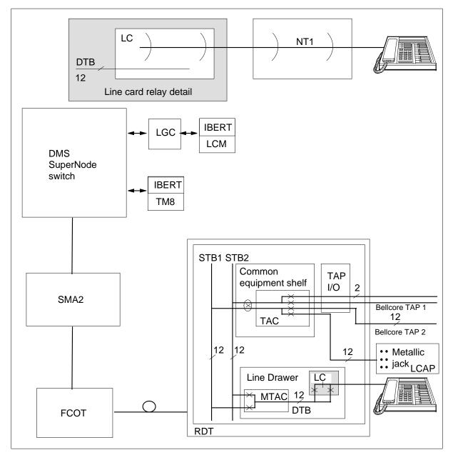
The DCHCON command uses test configuration 24. The D-channel on the subscriber line is looped back in the AccessNode or NT1. The number,
