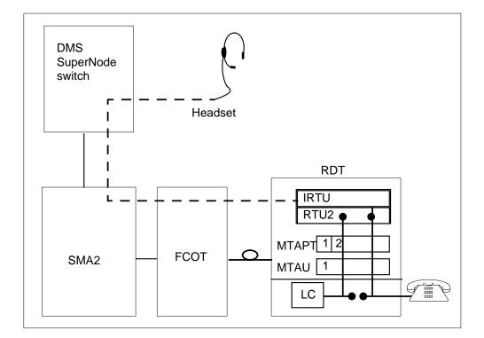
Figure 6-24 Test configuration for TALKLTA with battery
