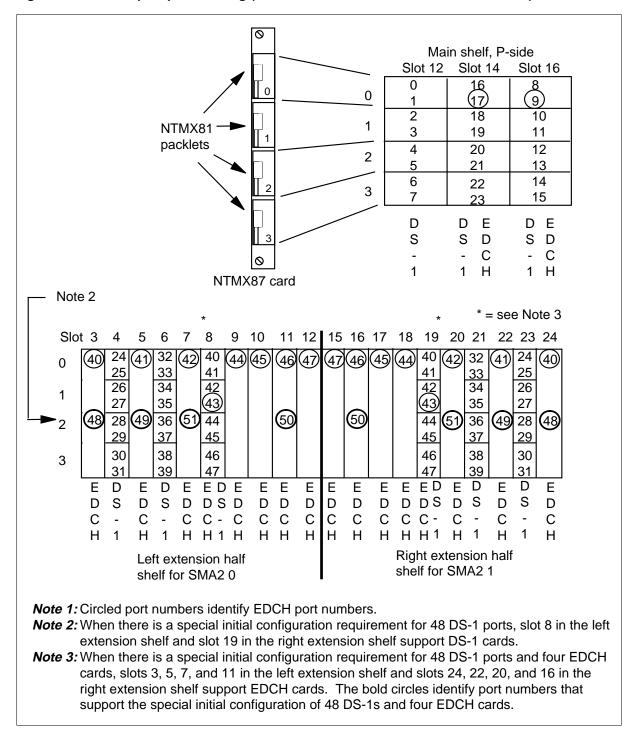
Figure 2-10 P-side port provisioning (in a CMVI and MVIE with an extension shelf)
