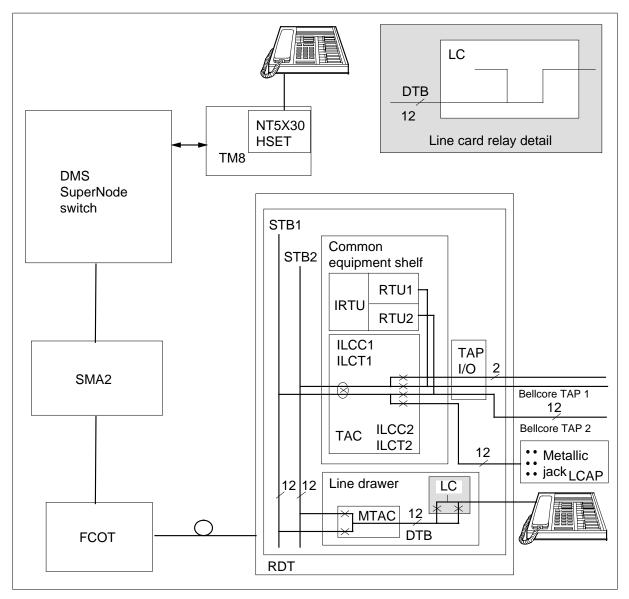
The TALKLTA, COIN, RING, and DGTTST tests use test configuration 11 when the IMC card is not equipped. A PCM path through the network connects the subscriber line to the HSET with a MONTALK circuit.
