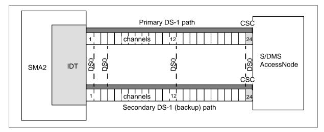
Figure 3-10 SMA2 to S/DMS AccessNode connectivity
