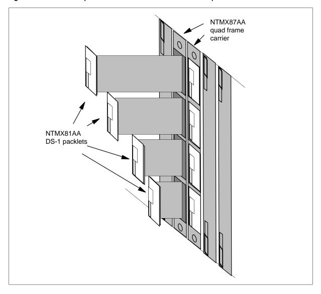
Figure 2-6 NTMX87AA quad frame carrier card with NTMX81AA packlets
