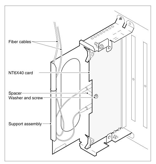
**c** Remove the screw and the spacer located between the card and the support assembly.
