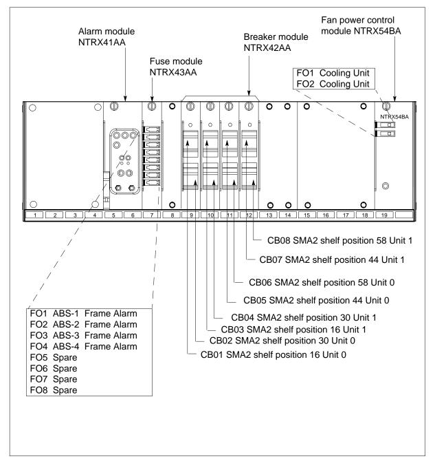
4 Use the previous MSP figures and the breaker designation label to identify which cards are serviced by each circuit breaker (CB). Many RX42 modules service two separate devices (or units); both units must be powered down prior to removal of the associated RX42 circuit card.
