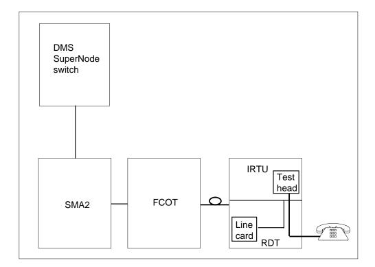
Figure 6-21 Test configuration for VDC, VAC, RES, CAP, and LNTST
