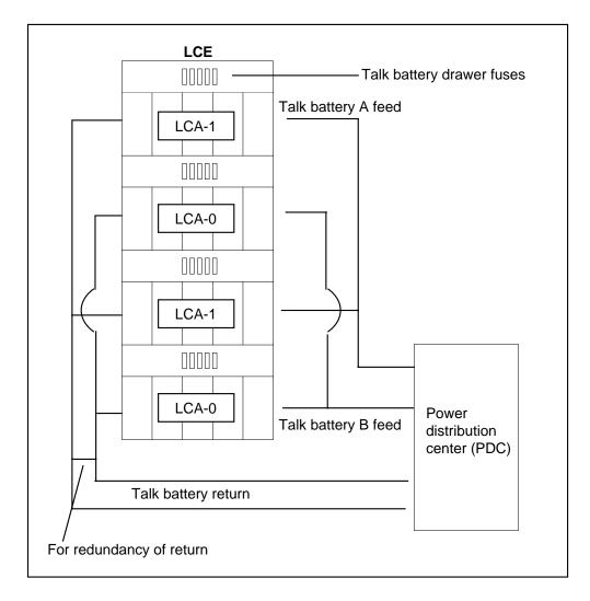
Figure 1-22 Talk battery distribution on LCE frame
