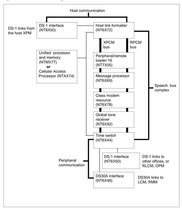
Figure 1-5 Functional block diagram of the RCC2
