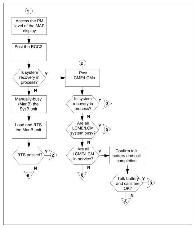
Summary of clearing a CPDC single power feed failure alarm (continued)
