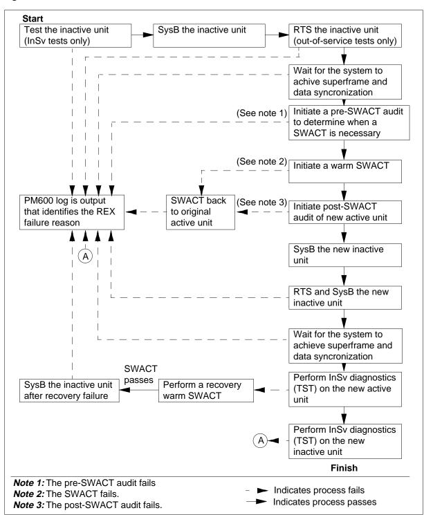
Figure 1-13 REx test state machine actions
