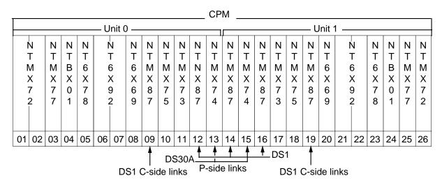
In NA010 and lower, up to 16 C-side ports are available. This configuration requires the NTMX87AA/AB in slots 9 and 19. NA011 and higher supports these packs when an office needs only up to 16 C-side links.
