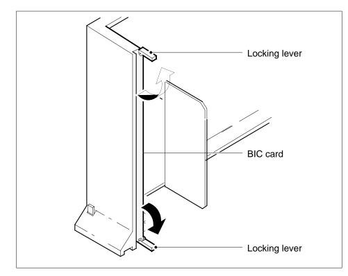
**15** Grasp the locking levers. Carefully pull the card toward you until the card clears the drawer.
