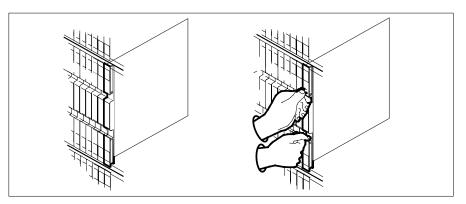
**b** Open the locking levers on the card to be replaced and gently pull the card toward you until it clears the shelf.
