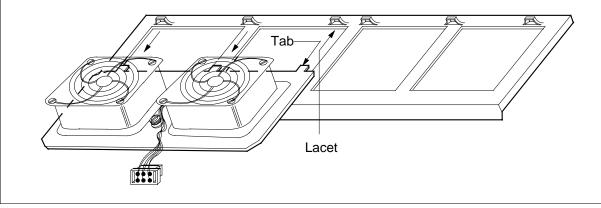
17 Carefully move the defective fan unit assembly (NTMX2658) around the bulkhead. Refer to the following diagram.
