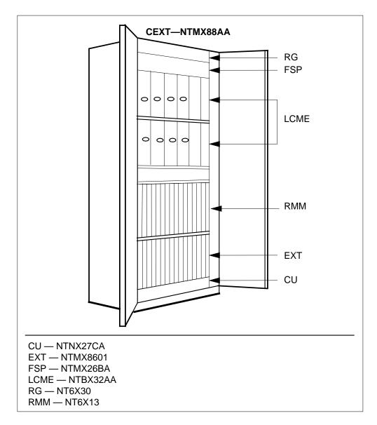
The CEXT provides room for additional DS-1 interfaces and DCH cards. The CEXT units 1 and 2 require the DS60 card that provides DS60 links to the CRSC. The extension card contains 12 DS60 links that connect the card to the RCC2 shelf. The EXT shelf uses two-extension cards.
