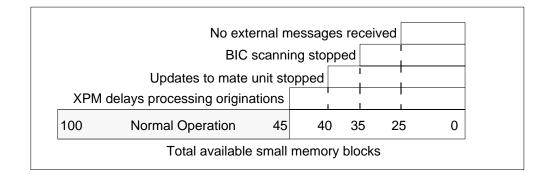
Figure 1-16 XLCM overload protection system
