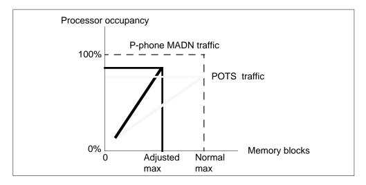
The XLCM is not equipped to handle real-time overload because the XLCM is memory block limited. This problem can allow the following conditions to cause outages:
