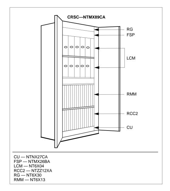
Figure 2-2 CRSC cabinet with LCM
