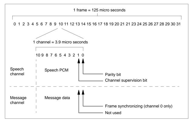
A frame synchronization bit is at channel 0 bit 0. This bit makes sure the RCC2 and the LCME or RMM recognize the start of each frame sequence.
