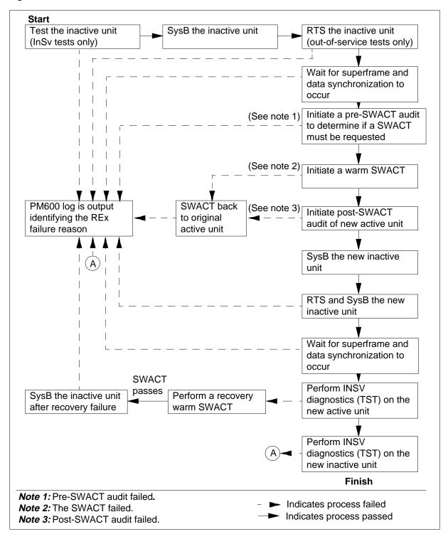
Figure 1-18 REx test state machine actions
