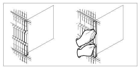
**b** Open the locking levers on the card to be replaced and gently pull the card toward you until it clears the shelf.
