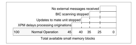
Previous POTS models of the small memory LCM (64k) can be memory block limited. The LCM uses the small memory blocks before the LCM runs out of real-time use. The design of the LCM depends on this loss of memory blocks before a loss of real-time use. Memory block limited is an LCM functionality that also applies to XLCMs.
