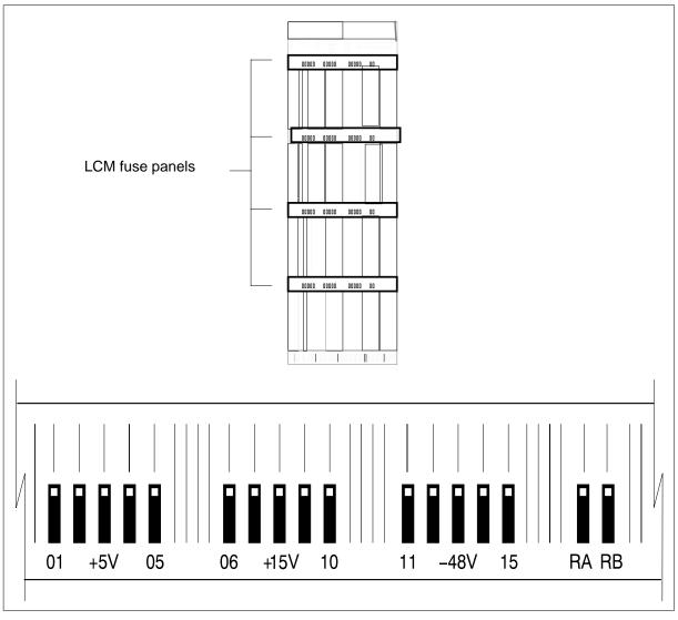
$\it Note:$  Fuses are coded for position. The colored square on the face of the fuse identifies the top edge.
