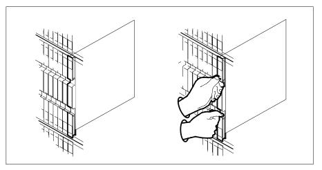
**b** Open the locking levers on the card to be replaced and gently pull the card toward you until it clears the shelf.
