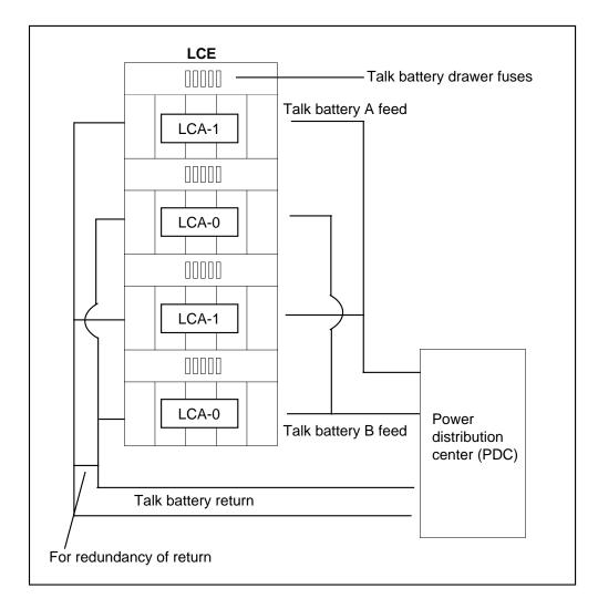
Figure 1-27 Talk battery distribution on an LCE frame
