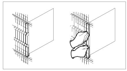
**b** Open the locking levers on the card to be replaced and gently pull the card toward you until it clears the shelf.
