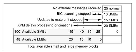
Figure 1-25 Overload protection system variable thresholds
