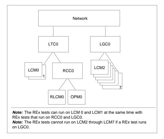
When the LCM\_REx\_TEST and the LCMCOV\_REx\_TEST are separate, faster completion of site REx\_TEST coverage occurs. The LCM\_REx\_TESTs that do not have limits of the converter voltage and ring tests run at the same time. The coordinator schedules these tests separately for maximum start periods.
