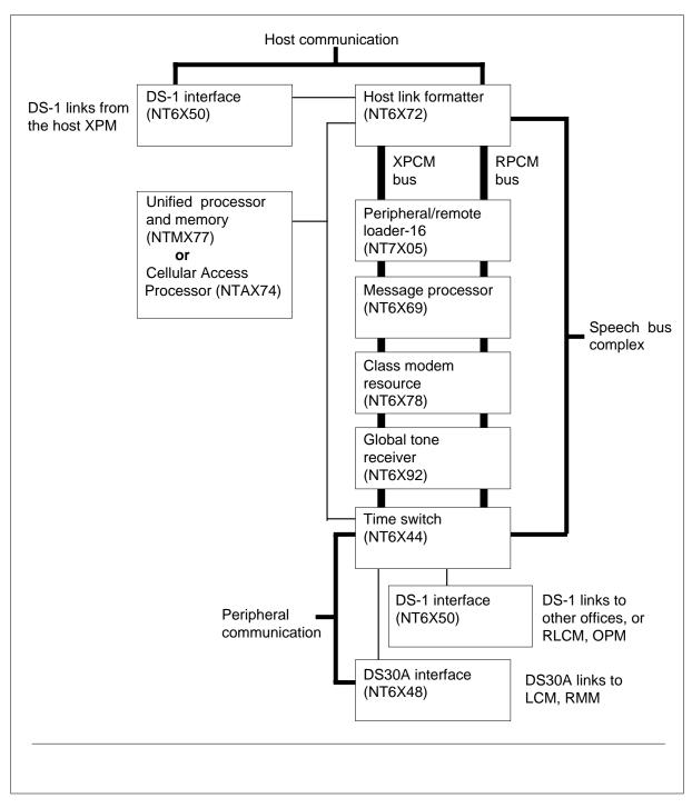
Figure 1-10 Functional block diagram of the RCC2
