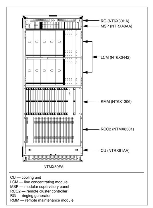
Figure 2-2 CRSC cabinet with LCM
