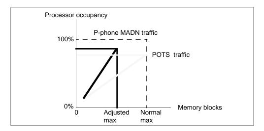
The XLCM is memory block limited. The XLCM cannot handle real-time overload. Outages can occur because of the following conditions:
