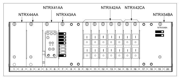
**Ringing generators** The provisionable NT6X30HA RGs module provides analog ringing voltage. The RG unit operates with the NTRX40AA MSP.
