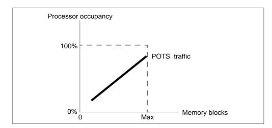
Figure 1-22 Processor occupancy or real-time use compared to memory blocks
