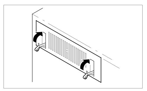
**23** Turn circuit breakers back ON. Ensure that ringing generator 0 is on circuit breaker 03-65-01. Ensure that ringing generator 1 is on circuit breaker 03-65-02.
