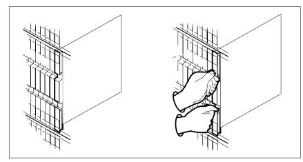
**b** Open the locking levers on the card to be replaced and gently pull the card toward you until it clears the shelf.
