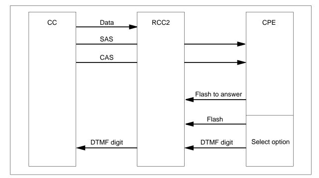
Alerting signals are sent to the CPE when a GTR channel is not available. If GTR channels are not available, data is not sent to the CPE. In the proprietary
