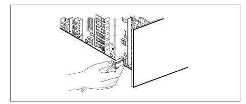
**13** Install the jumper connectors and cables removed in step 9 9 onto the replacement circuit card.
