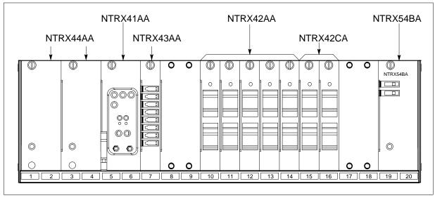
4 Power down circuit breaker supplying fuse module. Safety tag the front of the circuit breaker. When servicing the fuse module, fans may shut down, alarms may sound, or there may be a loss of alarms.
