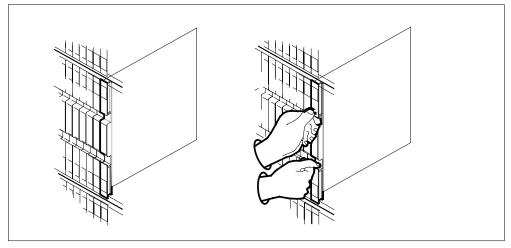
**b** Open the locking levers on the card to be replaced. Carefully pull the card toward you until the card clears the shelf.
