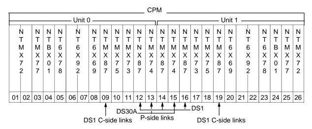
Figure 2-3 RCC2 circuit card layout
