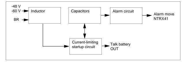
The NTRX44AA uses a 20A QHP77C bracket-mounted power inductor and six 80-V capacitors that provide 6800µF of capacitance.
