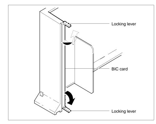
Open the locking levers on the face of the card.
