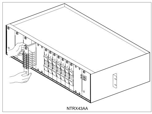
**10** Ensure the replacement circuit card has the same PEC, including suffix, as the circuit card just removed.
