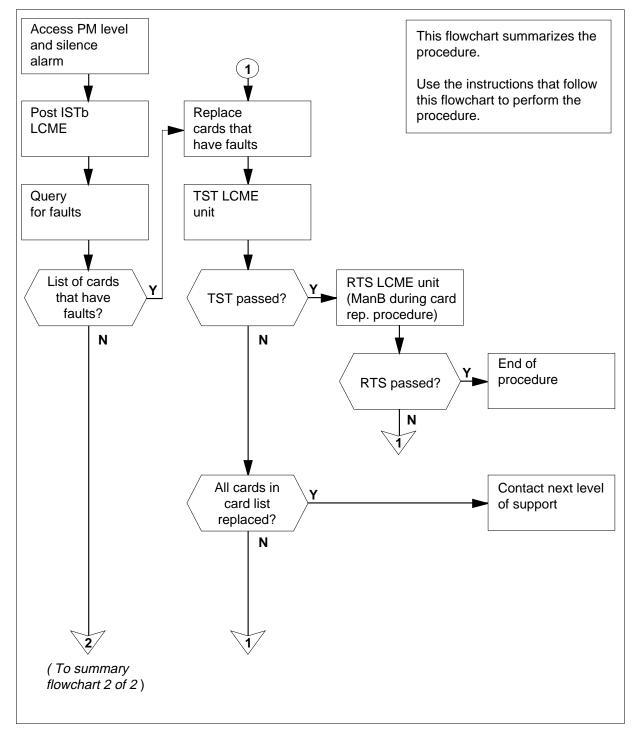
Summay of clearing a PM LCME (RG) minor alarm (flowchart 1 of 2)
