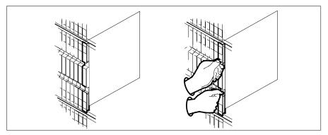
**b** Open the locking levers on the card to be replaced and gently pull the card toward you until it clears the shelf.
