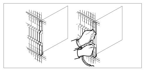
**b** Open the locking levers on the card to be replaced and gently pull the card towards you until it clears the shelf.
