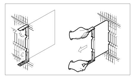
**c** Make sure the replacement card has the same PEC, including suffix, as the card you just removed. Also make sure the DIP switch settings on the replacement card match the settings of the card just removed.
