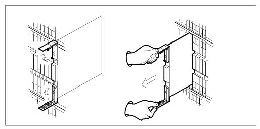
**c** Make sure the replacement card has the same PEC and PEC suffix, as the card you removed. Make sure all replacement card DIP switch settings match settings of the card you removed.
