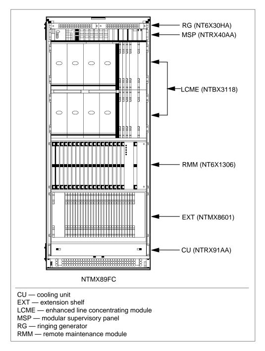
The CEXT provides room for more DS-1 interfaces and DCH cards. The CEXT units 0 and 1 require the DS60 card that provides DS60 links to the CRSC. The extension card contains 12 DS60 links that connect the card to the RCC2 shelf. The EXT shelf uses two extension cards.
