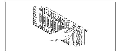
12 Install the jumper connectors and cables removed in step 8 onto the replacement circuit card.
