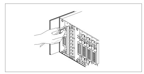
c Using the connector removal tool, manually disconnect the power connectors to the circuit card. Working from the bottom of the MSP shelf to the top of the MSP shelf, manually disconnect the smaller black power connectors located below the larger blue power connector. Manually disconnect the smaller black
