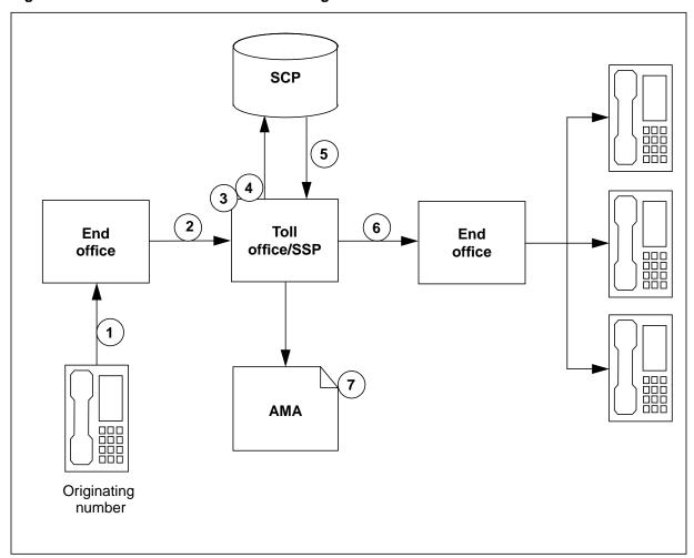
Figure 5 Call with COB overflow call routing from a toll office/SSP
