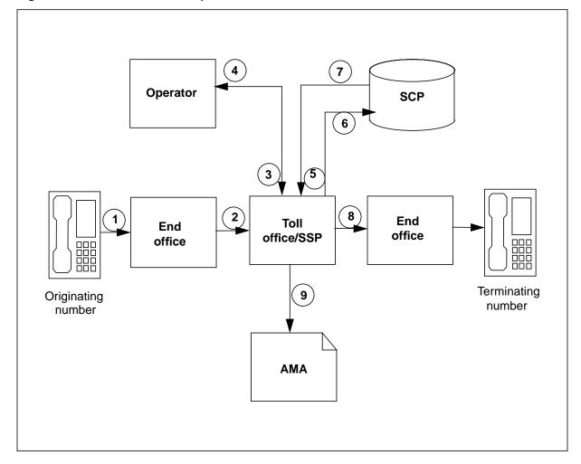
*Note:* This call goes to the operator only for entry of the calling number and does not receive full operator processing. It is treated like a nonoperator call once the calling number is entered. It does not produce TOPS AMA indicating operator handling of the call.
