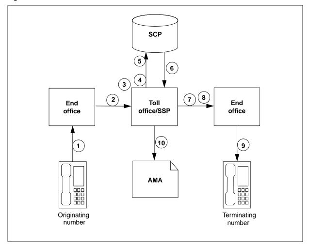
This 800Plus call proceeds normally, but the FTI flags in the SCP response indicate that the called DN has subscribed to EOD calling number (CID) or dialed number (DNID). This causes an initial address message (IAM) with a generic address parameter (GAP) to send the dialed 800 number (DNID) over an ISUP connection to the subscriber's phone set.
