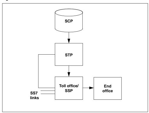
Figure 1 SS7 network architecture with toll office SSP
