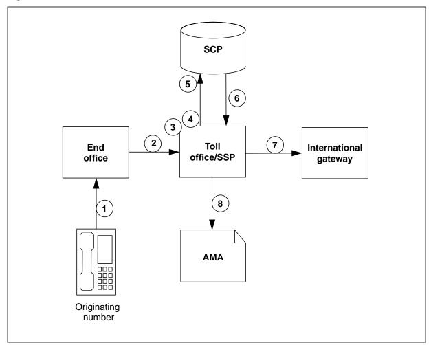
A number of signaling and call processing differences exist between routing to an SSP and an international carrier. The numbers in the figure relate to the call steps that are indicated in the following description.
