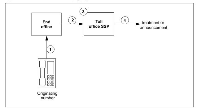
Figure 4 Call with automatic call gapping from an end office
