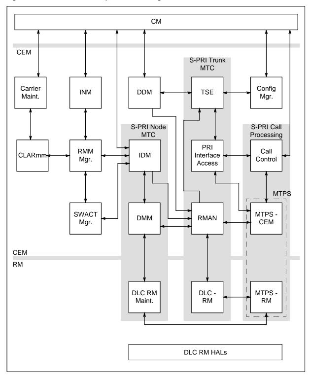
Figure 3-1 SPRI functional component block diagram
