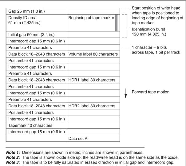
Note 4: The per-track placement tolerance is 0.075 mm (0.003 in.)
