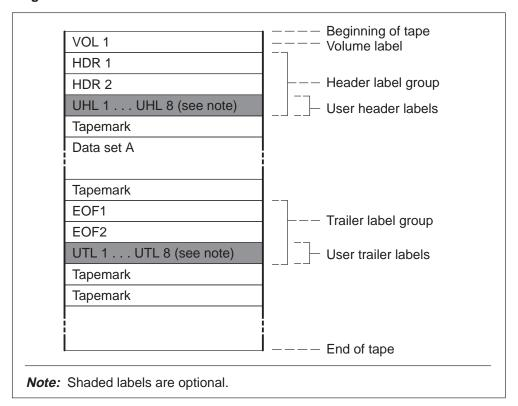
Figure 2-4 Label Structure - Multiple Data Sets - One Volume
