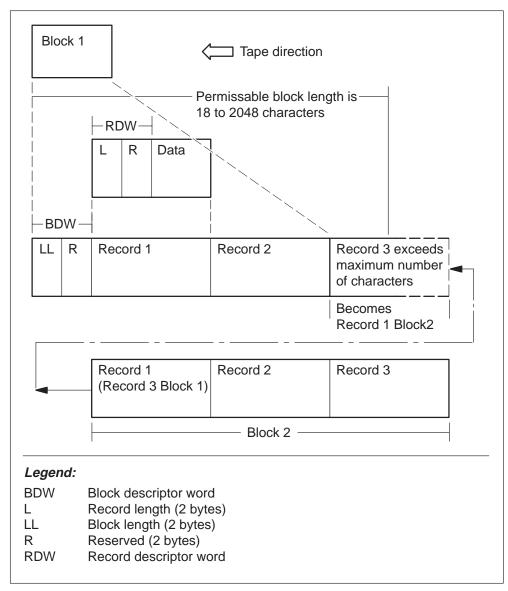
Figure 4-2 Variable-length, Blocked, Spanned (VBS) Format
