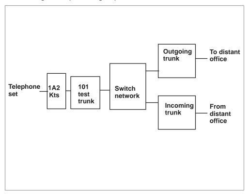
The test sequence for originating 101 test lines (TL101 communication trunks) is as follows.
