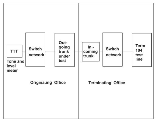
Figure 8-5 TL104 configuration (block diagram)
