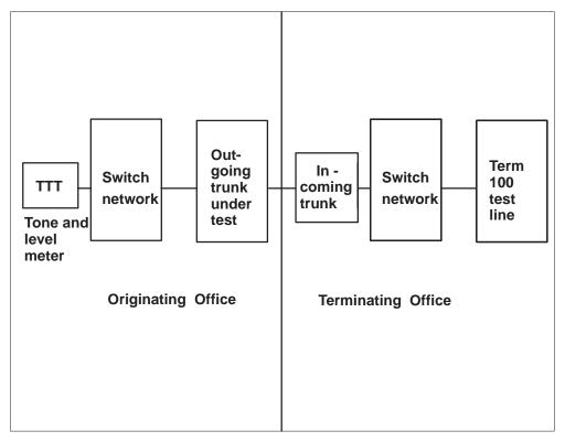
Figure 8-1 TL100 configuration (block diagram)
