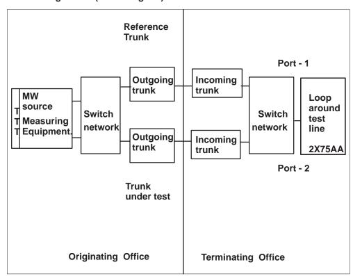
Figure 8-11 TLPA configuration (block diagram)
