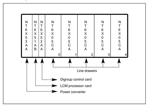
Two host LCMs, each one supporting a maximum of ten PLDs, are housed in a standard DMS-100 single-bay frame that is referred to as a line concentrating equipment frame. A maximum of 20 PLDs are assigned in one line concentrating equipment frame, as shown in Figure 1-6.
