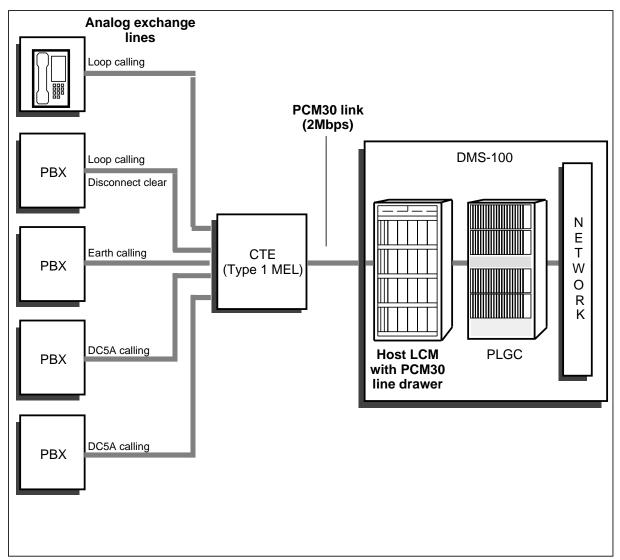
Figure 1-2xxx Provision of exchange lines from a PRLCM
