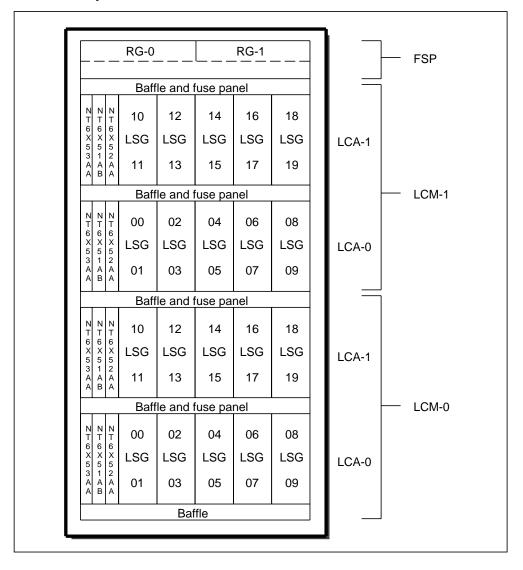
The PRLCM is a remote LCM. Similar to the host LCM, the PRLCM provides low-level functions, for example, line scanning and ringing. It is located at a remote site and connects to the PLGC through PCM30 links. Figure 1-7 illustrates the physical configuration of the PRLCM, which consists of the following components:
