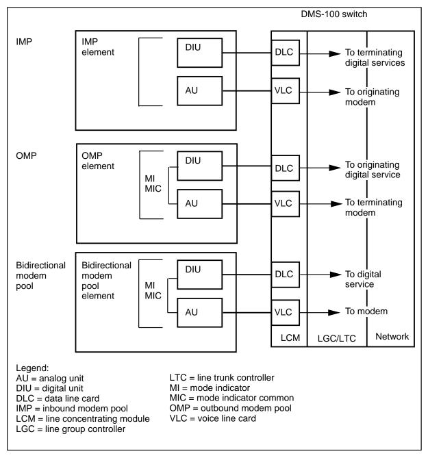
The number of elements (DU/modem pairs) in a modem pool is determined by traffic requirements for that particular pool. Each modem pool can have up to 256 elements. The total number of modem pools is constrained by the number of available common language location identifiers (CLLI). Several pools with different operating characteristics may be configured for use in different applications. Each modem pool is configured to handle inbound calls, outbound calls, or both inbound and outbound calls.
