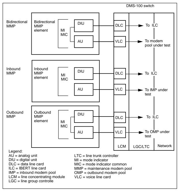
Figure 1-4 shows an MMP connection.
