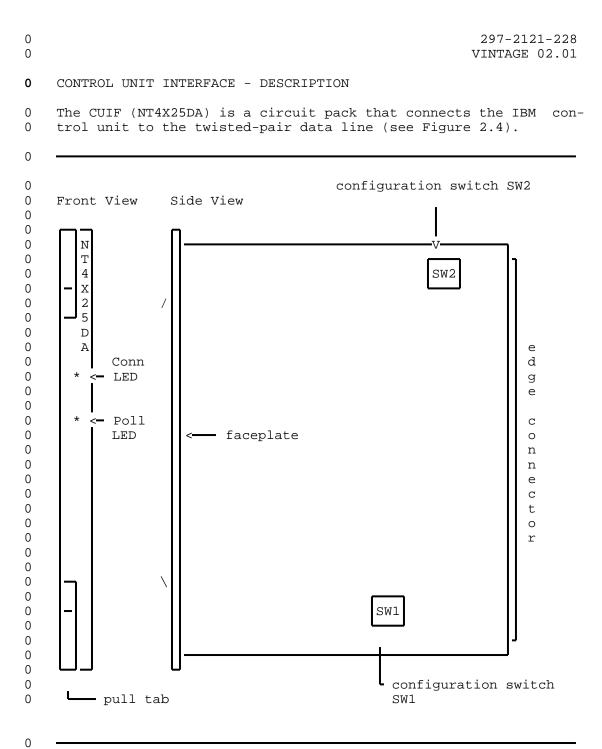
0 Figure 2.4 CUIF Circuit Pack - Front and Side View
