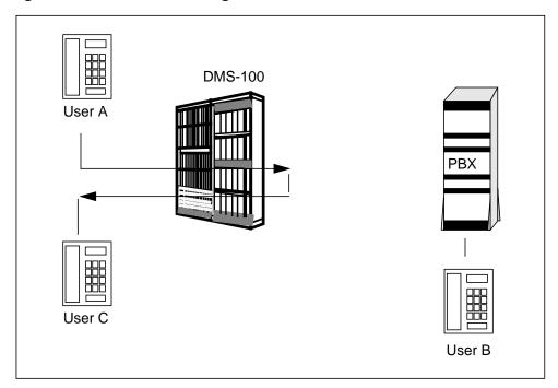
Figure 17-2 Results of invoking RLT
