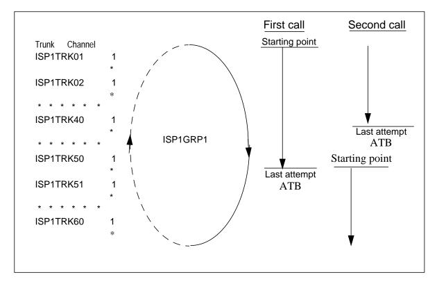
Figure 8-2 Representation of the route selection process when CHCL and SG\_CWCTH are datafilled
