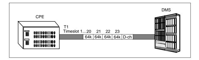
Two configurations for PRI, facility associated and non-facility associated (NFAS), are also referred to as 23B+D and NFAS, respectively. With facility associated PRI, a D-channel controls each DS1 span individually. With NFAS, one D-channel controls multiple spans. The concept is called nB+D. One D-channel can control as many as 20 DS-1 spans or 479 B-channels. With NFAS, there is also an option for a backup D-channel. The following figure shows examples of PRI configurations.
