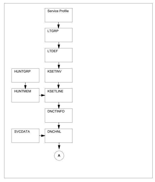
Figure 18-1 Table flow for PRI with Semipermanent Packet
