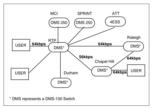
Figure 12-1 Illustration of Bearer Capability Routing
