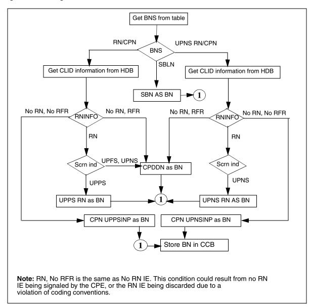
Figure 16-4 Billing number determination flow
