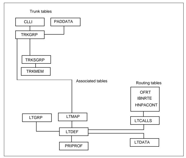
*Note:* Trunk tables assign the PRI trunk group to specific hardware port locations. Associated tables assign and link services to the trunk group. Routing tables describe how calls will be routed to the appropriate destination.
