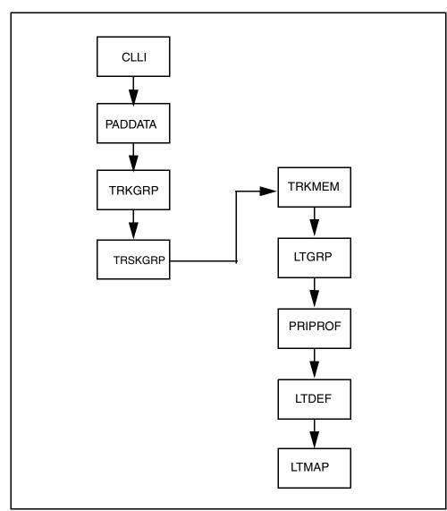
Figure 3-1 Table flow for PRI Base Service
