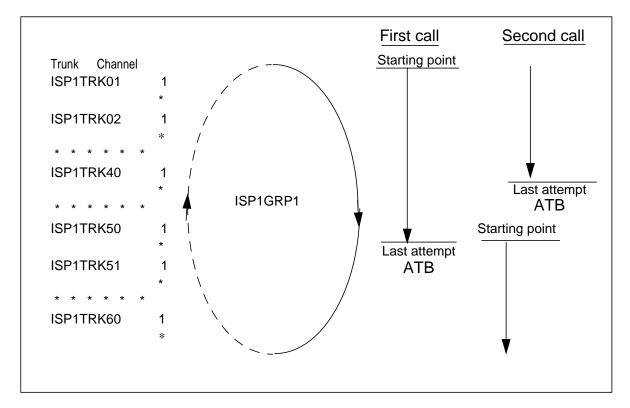
Figure 11-2 Representation of the route selection process when CHCL and SG\_CWCTH are datafilled
