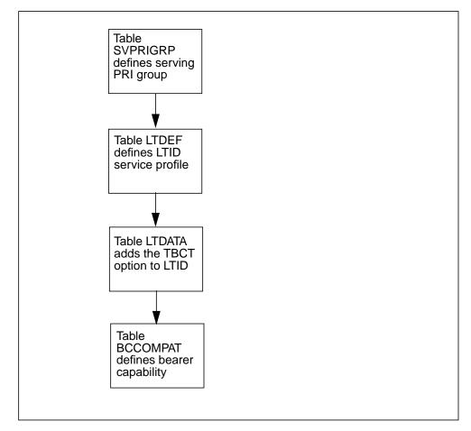
Figure 22-2 Table flow for PRI Two B-channel Transfer
