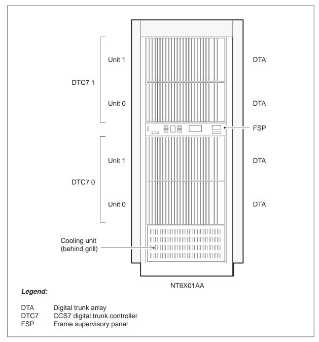
Figure 2-3 CCS7 digital trunk controller equipment cabinet NT6X01
