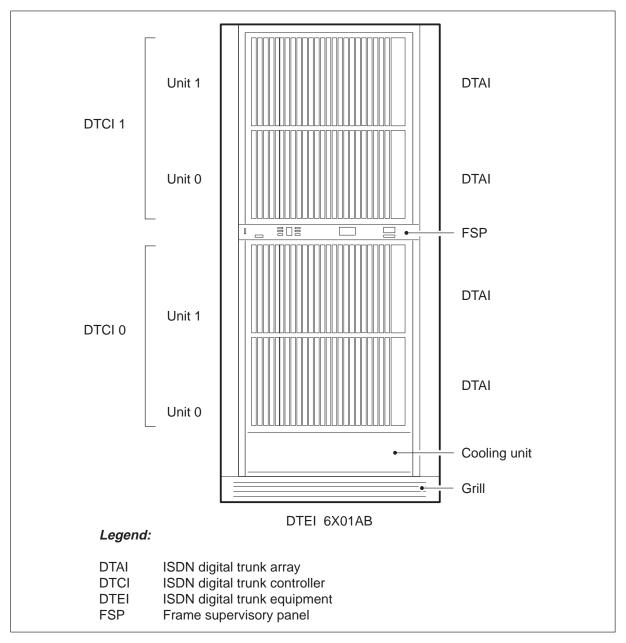
Figure 2-2 ISDN digital trunk controller equipment frame NT6X01
