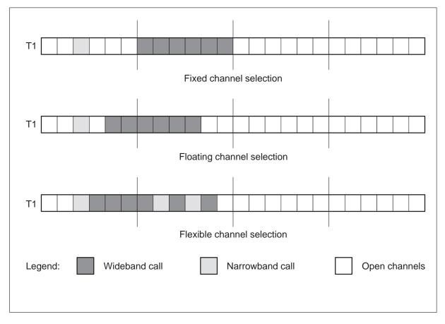
Figure 3-1 Trunk selection methods for T1 links
