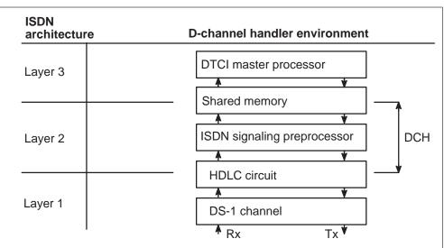
Figure 3-1 D-channel handler and ISDN layer comparison
