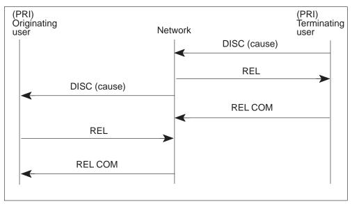
The UCS DMS-250 switch supports a two-message release sequence when handling abnormal error conditions. This sequence involves a REL-REL COM sequence of messages. The net results are identical to the three-message release sequence, in which the release sequence begins with a DISC message.
