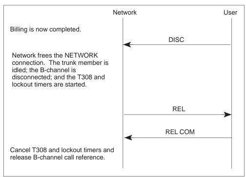
Figure 6-5 PRI-to-PRI trunk disconnect, user initiates call clearing
