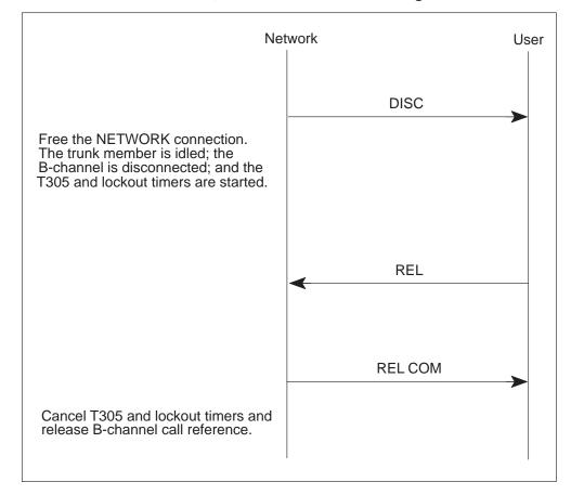
Figure 6-6 PRI-to-PRI trunk disconnect, network initiates call clearing
