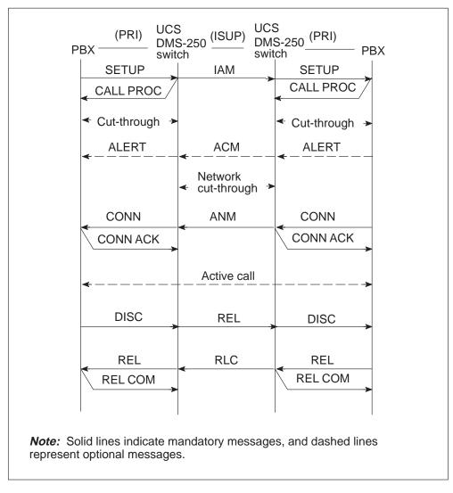
Figure 8-2 illustrates two-stage call clearing where a Q.931 REL message maps into the ISUP REL message at the interworking switch initiating call clearing (that is, the calling-access UCS DMS-250 switch) and an ISUP REL message maps into a Q.931 DISC message on the other interworking switch (the called-access UCS DMS-250 switch).
