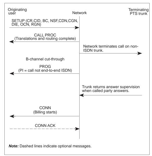
Figure 6-3 Q.931 message sequence for a PRI-to-non-ISDN trunk call setup
