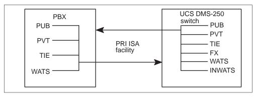
Enhancements to the PRI signaling protocol permit access to the segregated facilities within the network. The services provided over a single PRI include
