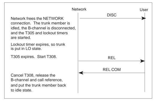
Figure 6-17 PRI-to-PRI call setup, no response from terminator
