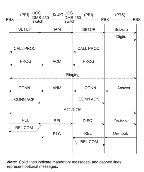
Figure 8-6 Interworking between PRI-to-PTS trunk
