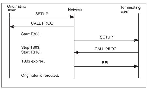
Figure 6-18 PRI-to-PRI call setup, no response after CALL PROC
