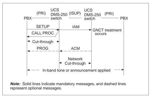
Figure 8-5 illustrates a call interworking with a non-ISUP trunk within the network. Note that the ACM is mapped to a PROG (instead of an ALERT message, indicating that interworking has been encountered. At the PTS/PRI interface, all Q.931 messages are received but ignored.
