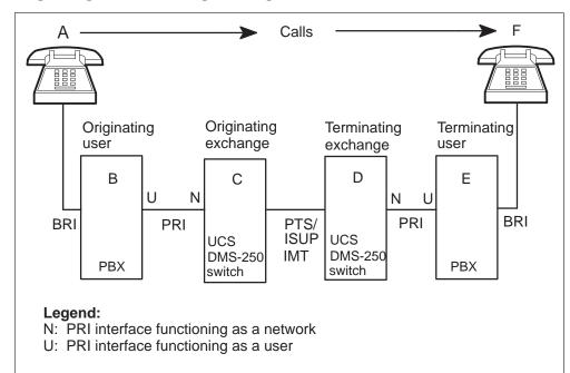
Figure 6-1 Originating and terminating exchanges in a PRI connection
