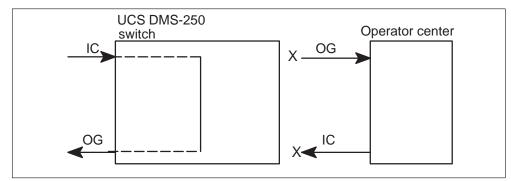
Figure 9-3 Trunk configuration for operator services bridging
