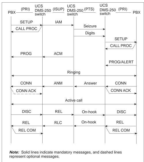
Figure 8-5 Interworking with a non-ISUP trunk within the network
