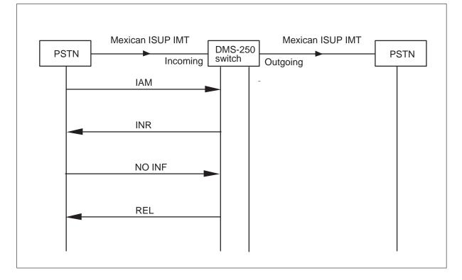
When an INF does not arrive after the UCS DMS-250 switch sends an INR, the call is taken down.
