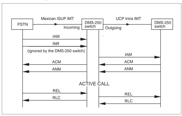
When an unsupported message is received from the originator, the unexpected message is ignored by the UCS DMS-250 switch, as shown in Figure 5-10.
