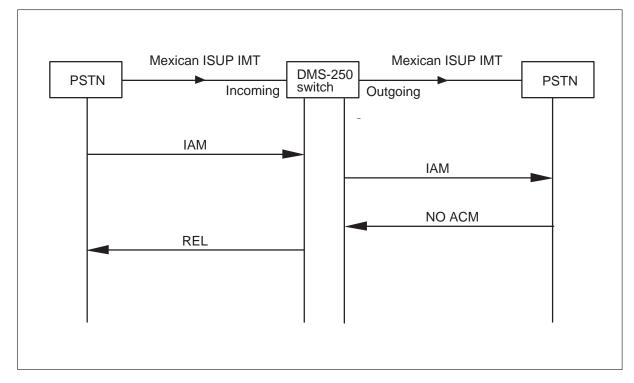
When an ACM does not arrive after the UCS DMS-250 switch sends an IAM, the call is taken down.
