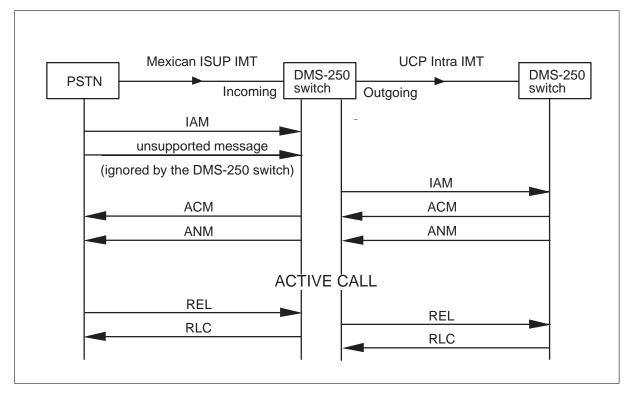
The Connect (CON) message is reported internally to the UCS DMS-250 switch as an ANM. UCP ISUP does not support the Connect message. The Connect message is interworked to a UCP trunk as an ANM.
