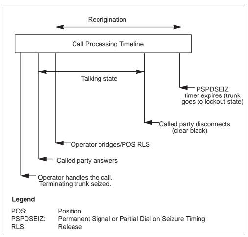
Figure 1-8 STR reorigination timeframe, operator bridge after answer
