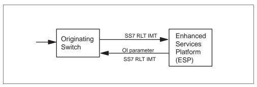
The host switch sends the OI parameter to the originating switch. The OI parameter can be included in one of the following SS7 messages:
