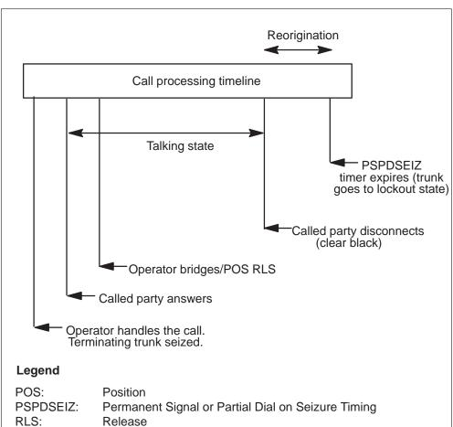
Figure 1-6 DTMF reorigination timeframe, operator bridge after answer
