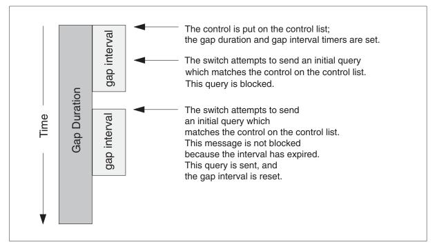
For the duration of an ACG control, the actual length of time that elapses before the switch can send a query is specified by the gap value. The gap value is a randomized length of time, between 90 and 110% of the gap interval for the control. The gap value is randomized each time the gap interval is reset.
