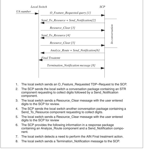
In this example the customer is using a debit card. This customer may dial a Universal Access (UA) number which triggers at *O\_Feature\_Requested*. The SCP decides it needs additional information to complete the call (the users access code) and sends a **send\_to\_Resource**. The user complies by entering in their personal access code at which the switch sends a **Resource\_Clear**
