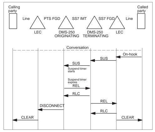
• If the originating switch receives an SUS for the terminating circuit and then receives an RES before it receives either an on-hook on the originating circuit or an REL for the terminating circuit, it cancels the suspend timer and returns the call to the talking state.
