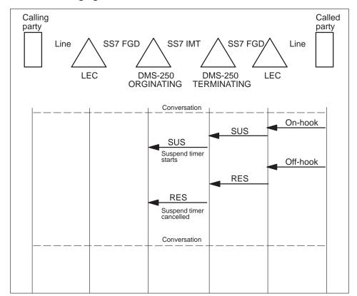
Figure 15-2 SUS-RES messaging, end-to-end SS7
