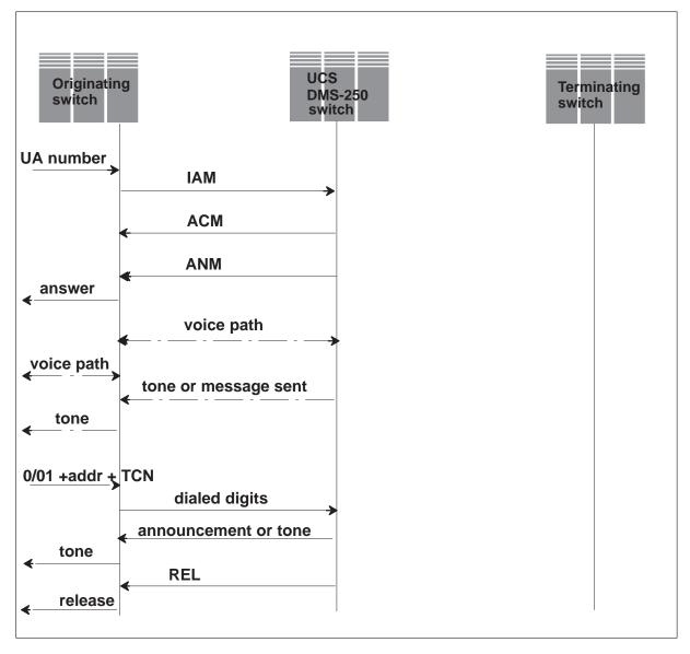
In Figure 6-7, the UCS DMS-250 switch does not start billing. The call detail report's (CDR's) field TRMTCD is set to the treatment code and the COMPCODE field is set to 1, which indicates the call was treated.
