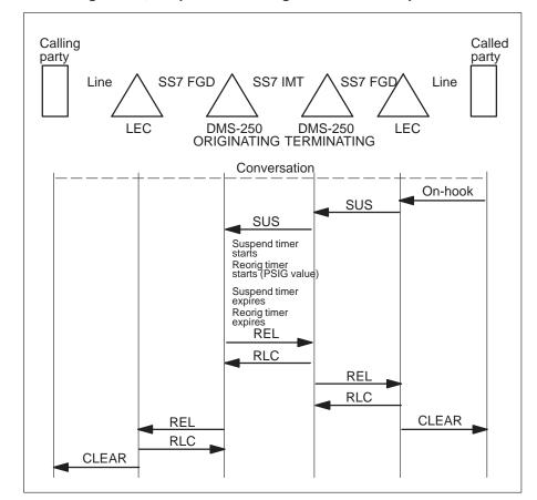
Figure 15-9 Manual reorigination, suspend and reorigination timers expire
