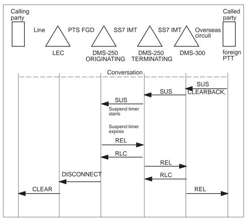
• If the originating UCS DMS-250 switch receives an SUS for the terminating circuit and then receives an RES before receiving either an on-hook on the originating circuit or an REL for the terminating circuit, it cancels the suspend timer and returns the call to the talking state.
