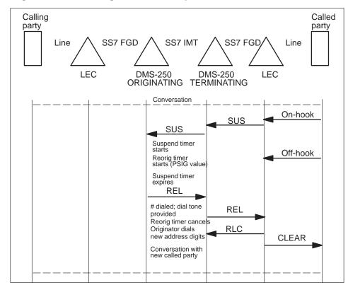
Figure 15-10 Manual reorigination, suspend timer expires and calling party reoriginates before reorigination timer expires
