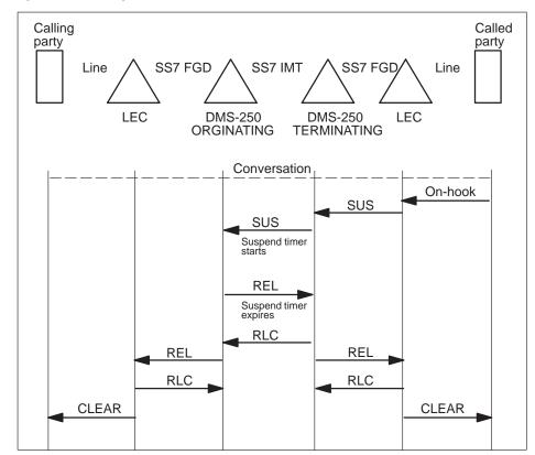
Figure 15-1 Suspend timer expiration, end-to-end SS7
