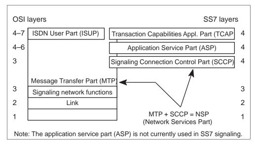
Figure 16-1 Open Systems Interconnect (OSI) and SS7 comparison
