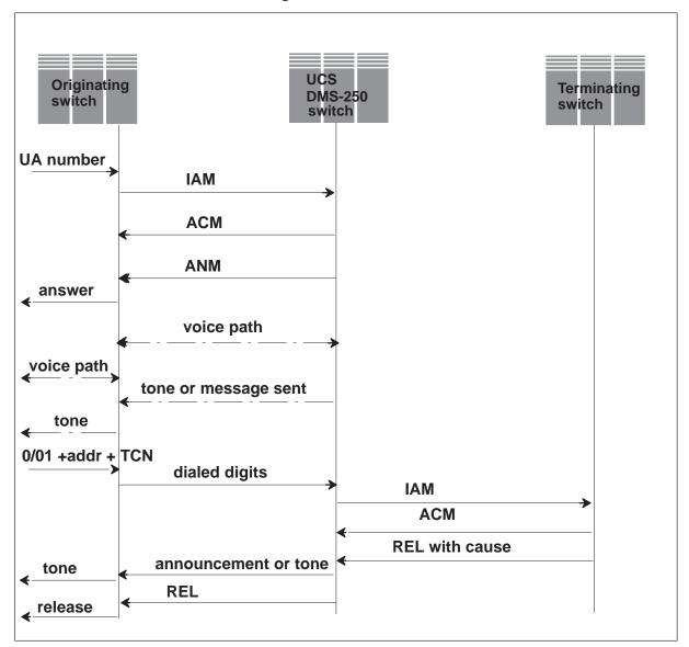
Figure 6-8 Unsuccessful UA call at the terminating switch
