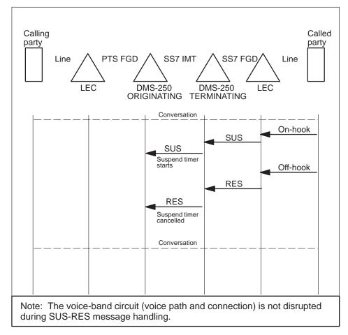
• If the originating switch receives an SUS and then receives an on-hook for the originating circuit before it receives an RES or an REL for the terminating circuit, it idles the originating circuit and sends an REL for the terminating circuit.
