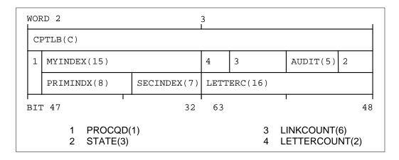
The field CPTLB extends across WORDS 2 and WORDS 3. Beneath CPTLB are two rows of field names, one beginning with field MYINDEX and the other with field PRIMINDX. The numbers in parentheses identify the fields' size in bits.
