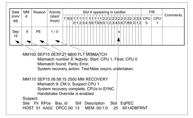
To complete the trend table, add the information from the virtual registers field of the MM100 log. The virtual registers field displays the following information:
