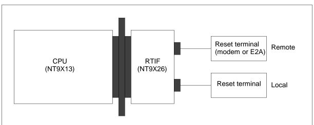
The NT9X26 card contains the OOB link interface that collects OOB reset code bits. The system assembles the bits and sends them to the CPU of the RTIF. This CPU determines the type of reset to perform. The RTIF contains a CPU, RAM, and EPROM. The OOB link between modules allows the CM to reset other nodes.
