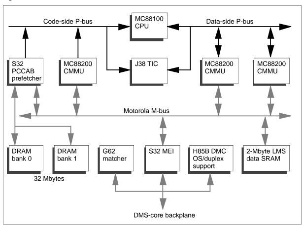
Figure 6-1 NT9X10AA BRISC CPU card architecture
