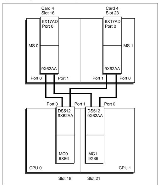
Figure 1-6 SuperNode SE CM-to-MS port connection diagram
