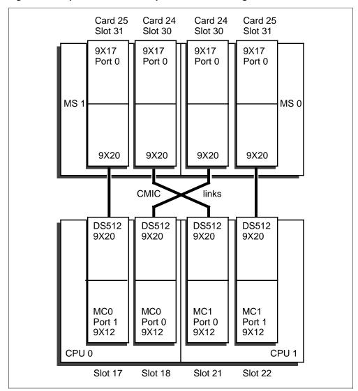
Figure 1-5 SuperNode CM-to-MS port connection diagram
