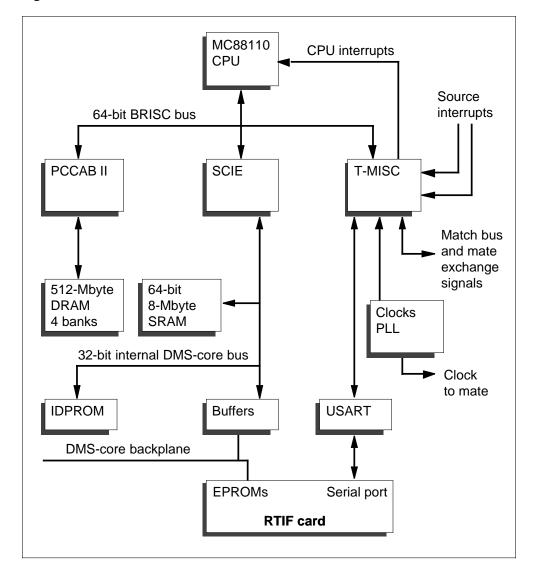
Figure 6-4 NT9X10DA BRISC CPU card architecture
