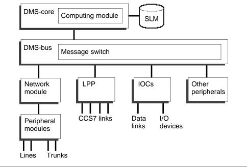
Figure 1-2 SuperNode SE system architecture
