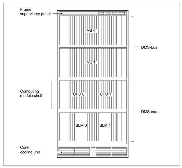
Figure 1-4 SuperNode SE SCC cabinet layout
