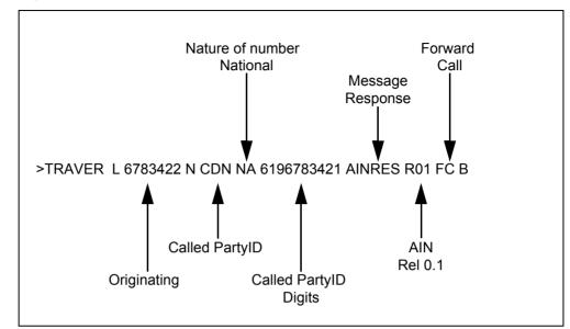
Figure 475 TRAVER command line for AIN forward call response example
