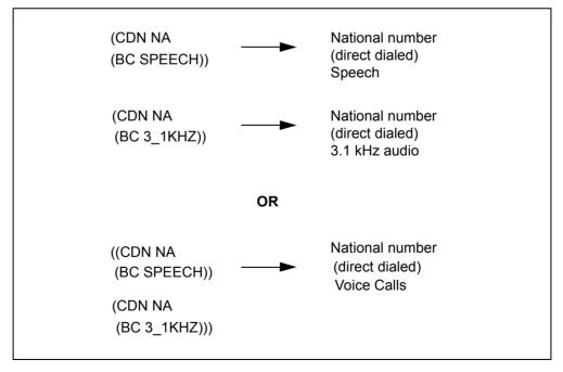
Though both methods are correct, the one shown in Figure 49 is preferred because it minimizes datafill in the tables that use RCNAME.
