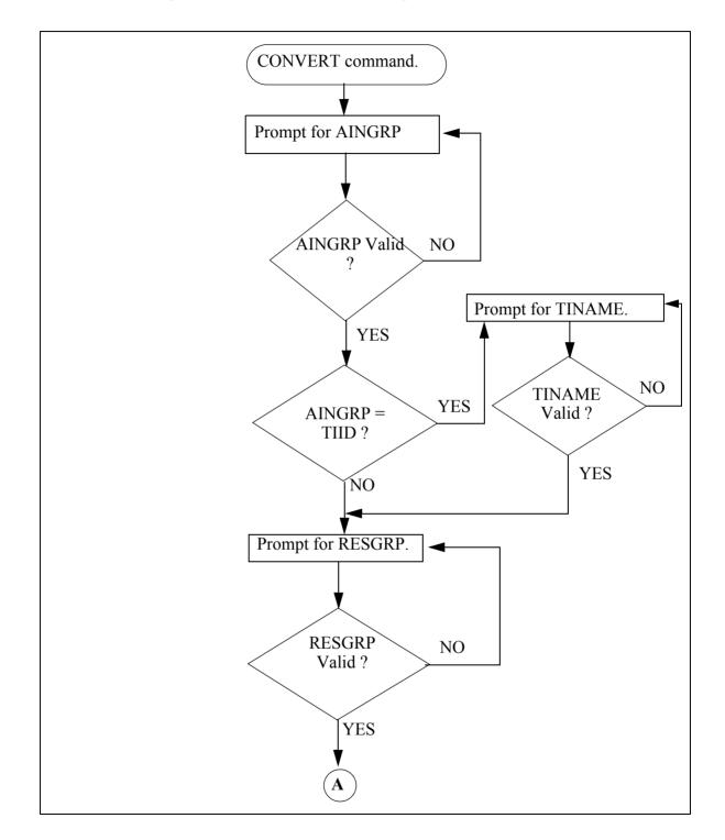
Figure 543 Functional behavior diagram of AINSCT tool
