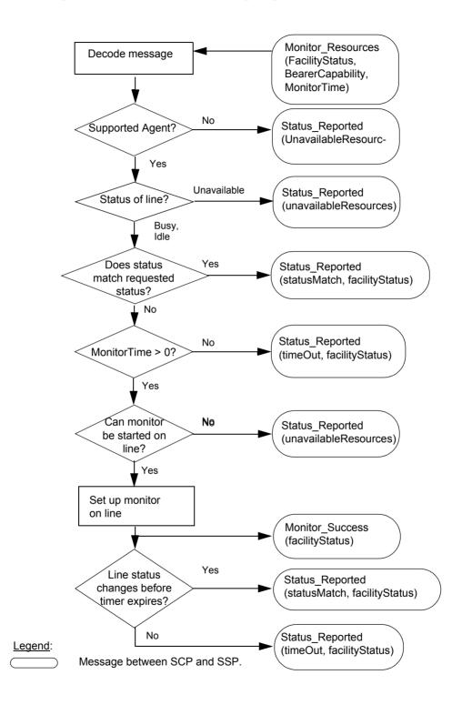
Figure 104 Process for monitoring single lines
