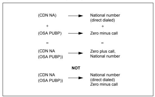
Figure 48 Example #1: combining routing characteristics
