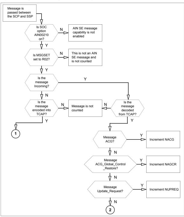
Figure 118 Logic flow for OM group AINNCR registers
