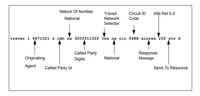
The following figure provides sample TRAVER output for PXLAMAP ISDN digit conversion.
