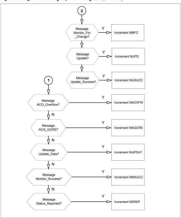
Figure 118 Logic flow for OM group AINNCR registers (continued)
