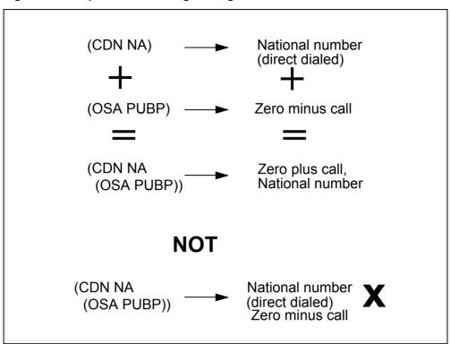
Figure 2 Example #1: combining routing characteristics
