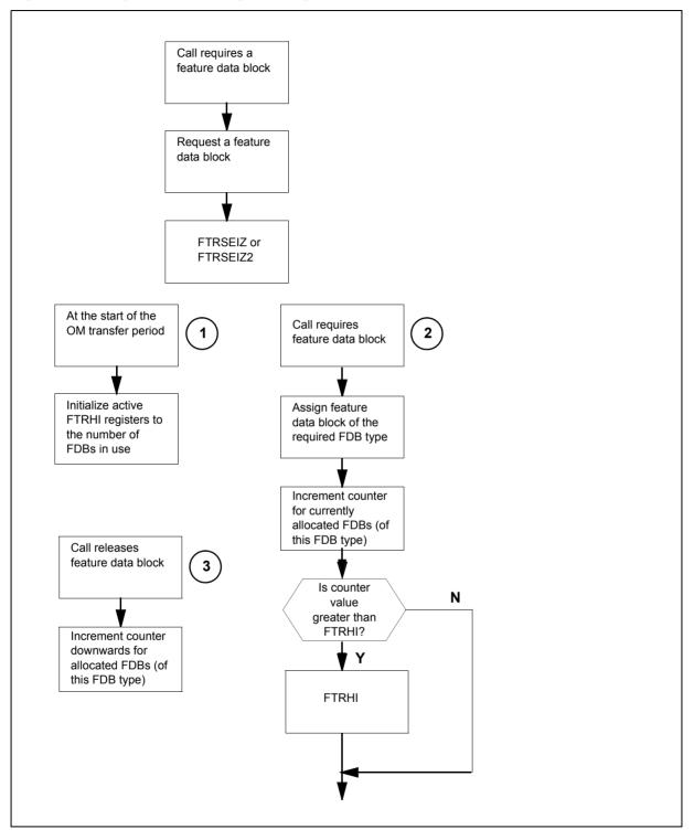
Figure 122 OM group FTROM registers logic flow
