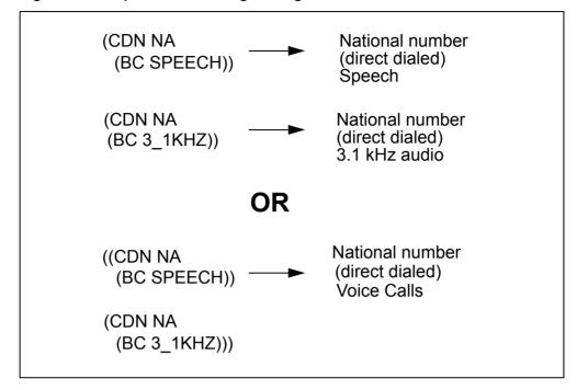
Figure 3 Example #2: combining routing characteristics
