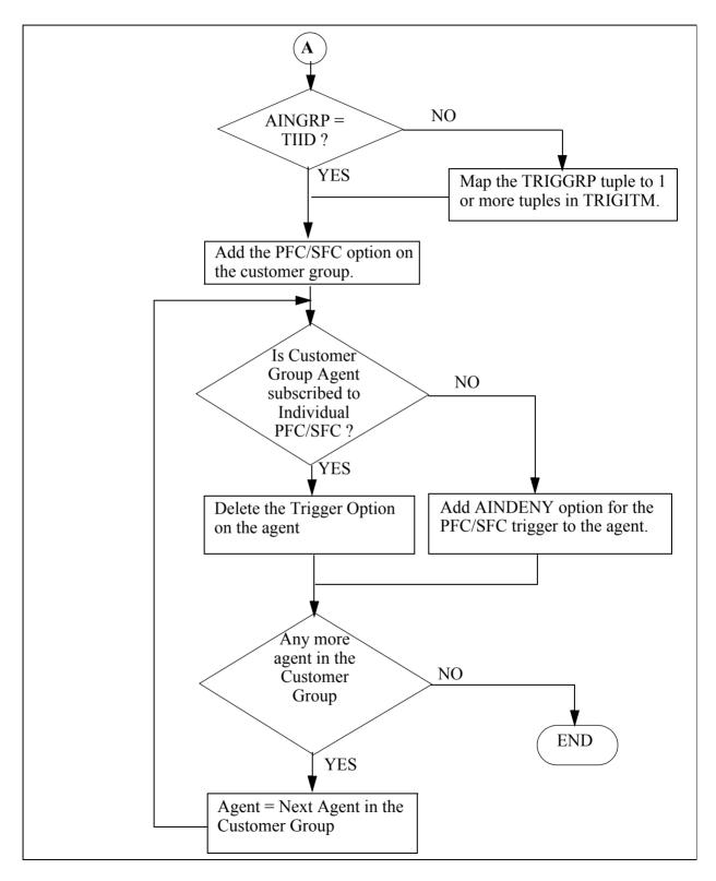
Figure 544 Functional behavior diagram of AINSCT tool (continued)
