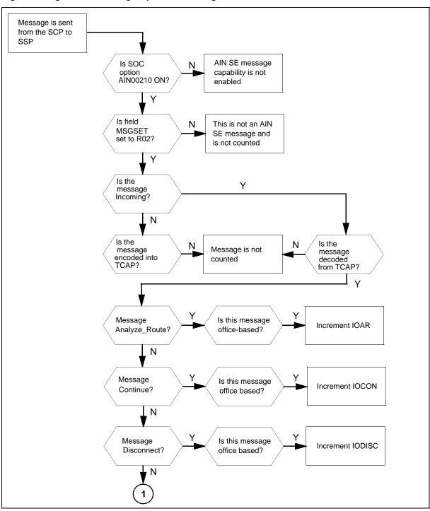
Figure 2 Logic flow for OM group AINICOFF registers
