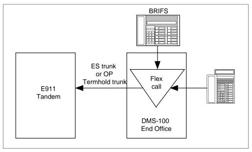
The E911 Tandem must support incoming trunks with 911 traffic, as well as local lines and any 911 traffic these lines generate. When a line on an E911 Tandem calls 911, the call is routed to a PSAP using an OP or ES loop around trunk because the E911 Tandem does not support direct, line-to-PSAP connections.
