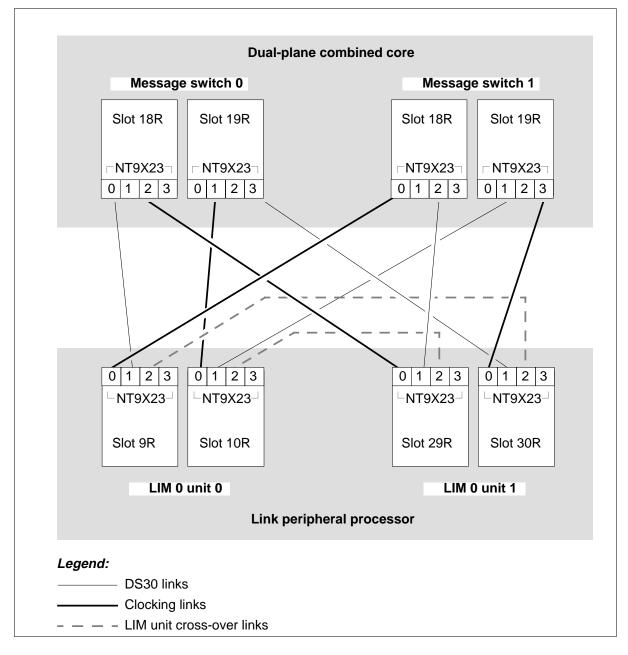
The following table lists the slots and ports for each LIM. On the MS, slots 18R and 19R have been used in the example. However, any slots from 6 to 26 can be used. Those links marked with an asterisk (\*) indicate clocking links.
