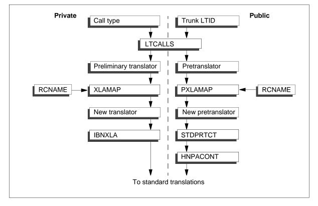
For the incoming circuit-switched call, table CLLI identifies the trunk group, and table TRKMEM determines the physical location of the circuit carrying the call. The trunk identifier (CLLI) is used to access table TRKSGRP, which defines the signaling protocol used by the trunk, and table TRKGRP, which provides the LTID of the trunk group. The LTID of the PRI trunk group and the call type from the SETUP message are used to access table LTCALLS.
