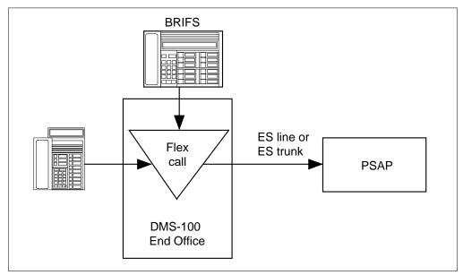
Enhanced 911 concentrates all 911 calls from a number of end offices to a centralized DMS-100 switch, known as E911 Tandem. When the calls arrive at the E911 Tandem, they are routed to an appropriate PSAP.
