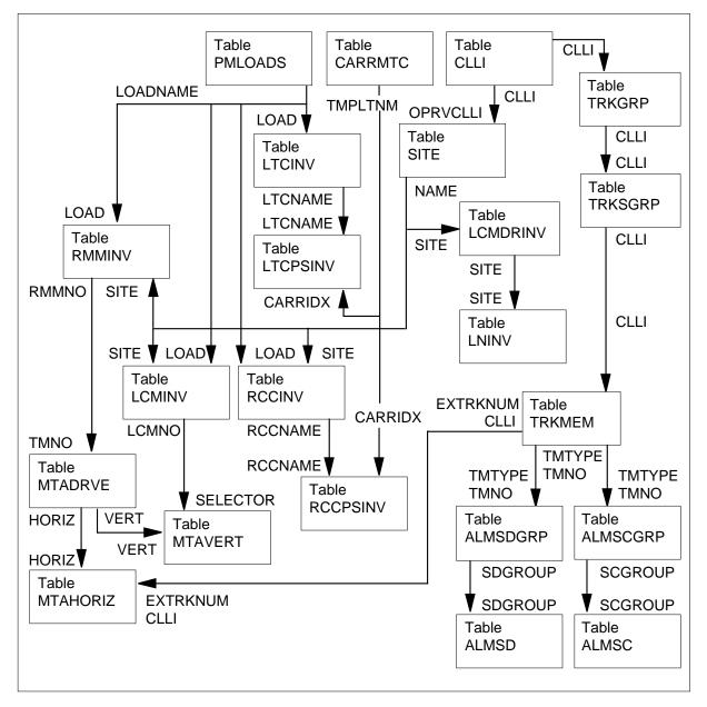
The following figure illustrates the table flow to datafill HSTP0 DMS ADSL Capability.
