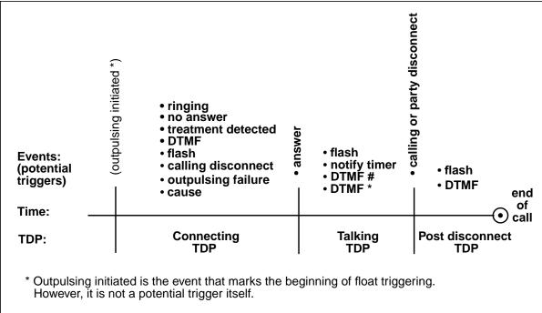
The answer trigger event is special because it causes trigger processing to transition from the connecting TDP to the talking TDP. Similarly, a disconnect from either party causes trigger processing to transition from the talking TDP to the post disconnect TDP.
