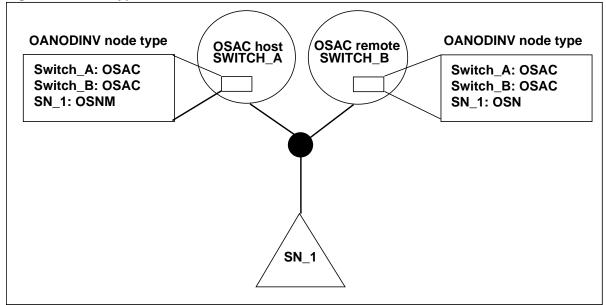
In addition to identifying the node type, table OANODINV also provides the relationship of the OSAC switch to the other OSAC switch (or switches) in the network. A relationship of SELF applies to the switch where the datafill exists. A relationship of OTHER applies to all other switches.
