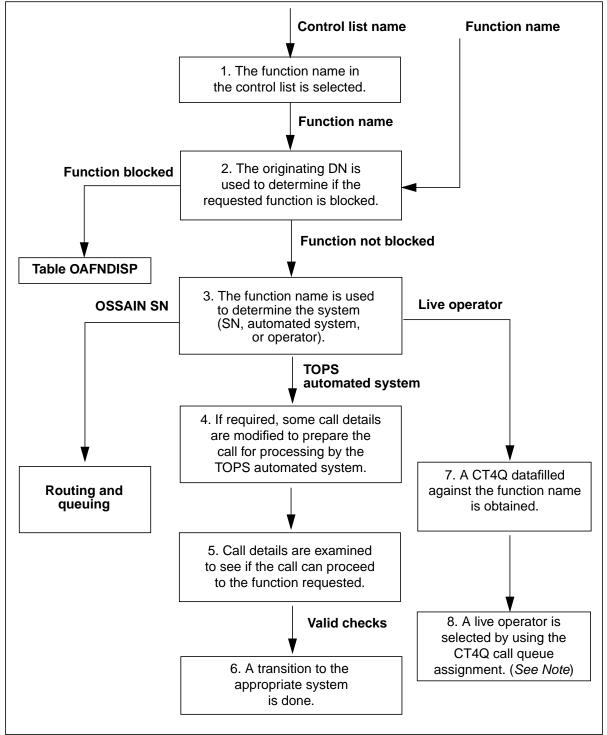
*Note:* Additional CT4Q refinements can be applied to OSSAIN calls that are routed to an operator. This option affects the CT4Q assignment. For details, refer to Chapter 4: "OSSAIN enhancements."
