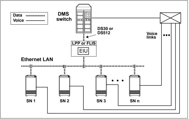
A switch can support a maximum of eight EIUs. Only four EIUs can be provisioned on a single LPP; however, up to eight can be spanned across multiple LPPs. A maximum of eight EIUs can be provisioned on a single FLIS or spanned across multiple FLISs. EIUs act as routers between the DMS CM and the LAN subnets. They are not intended to be used as routers between different LANs.
