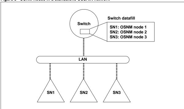
Figure 3 OSNM nodes in a standalone OSSAIN network
