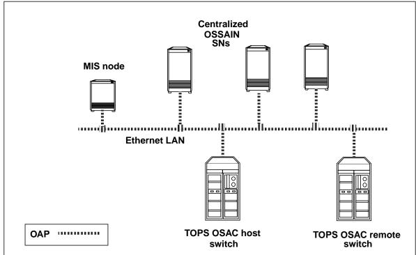
The following figure shows an MIS node in a simple OSAC topology.
