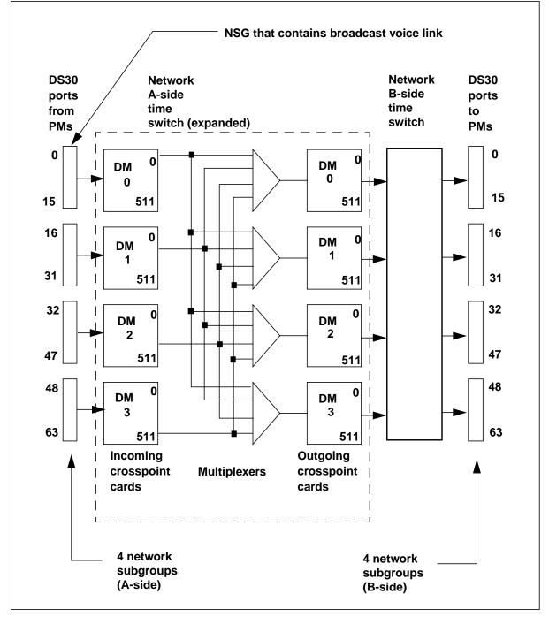
The figure shows two NT5X13-type JNETs (an A-side and a B-side network). A total of 64 P-side ports are on each NM. Ports 0 to 15 make up the first NSG, ports 16 to 31 the second, ports 32 to 47 the third, and ports 48 to 63 the fourth.
