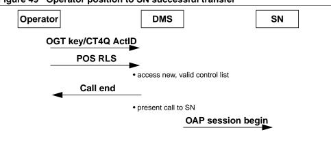
Figure 49 Operator position to SN successful transfer
