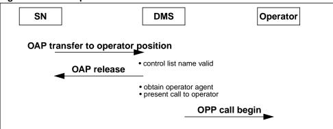
Figure 47 SN to operator successful transfer
