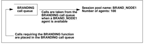
*Note:* Although this figure shows a branding call queue, it should be noted that calls are *not* queued if an agent is immediately available. Furthermore, queuing is optional and can be prevented through switch datafill. However, all calls requiring an OSSAIN agent are assigned a call queue so that an agent can be requested from the CAM.
