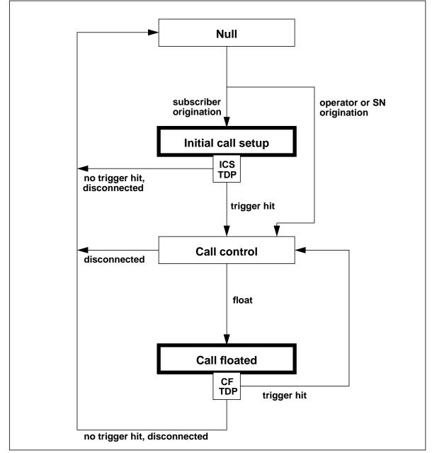
*Note:* DMS switch trigger processing occurs only for those PICs where the SN or operator is not linked to the call.
