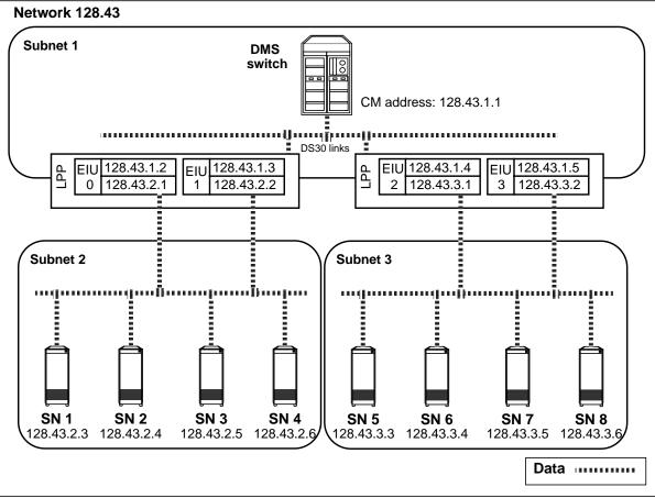
In Network 2, two EIUs support subnet 2 and two support subnet 3. IP traffic between the DMS SuperNode and subnet 2 is exchanged on either EIU 0 or EIU 1; and IP traffic between the DMS SuperNode and subnet 3 is exchanged on either EIU 2 or EIU 3.
