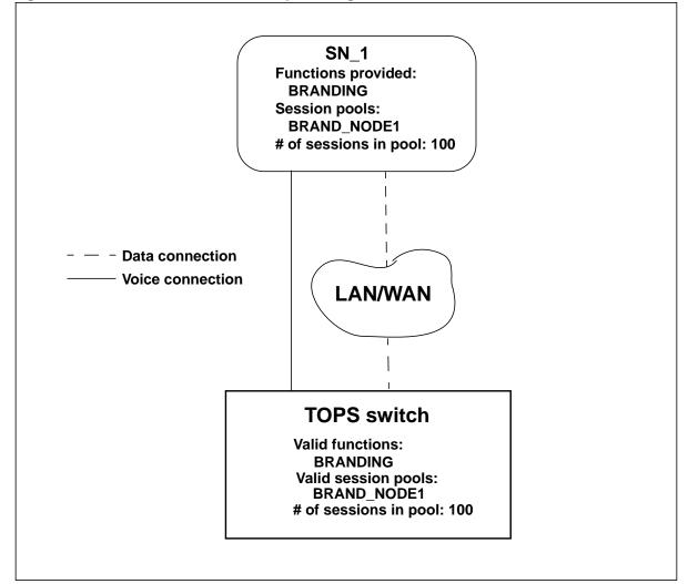
Figure 8 One function on one SN sample configuration
