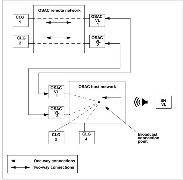
In Figure 78, the OSAC host switch also functions as a standalone switch. Four separate calls are shown connected to a single broadcasting SN voice link. Two of these calls originated in the OSAC remote switch (calls 1 and 2) and two originated as standalone calls in the OSAC host switch (calls 3 and 4).
