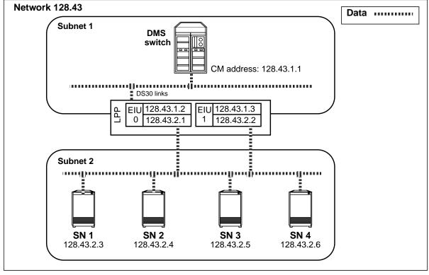
EIU routing software uses only one EIU at a time to carry IP traffic to its LAN subnet. This EIU is referred to as the *primary* EIU.
