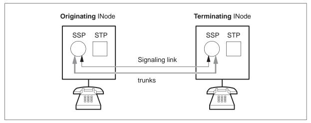
*Note*: The DMS-INode is performing an SSP function in this configuration.
