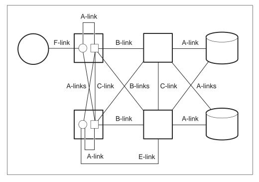
Figure 1-5 SNA7 DMS-INode within a typical CCS7 network
