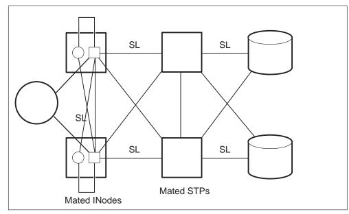
Figure 1-6 MNA7 DMS-INode within a typical CCS7 network
