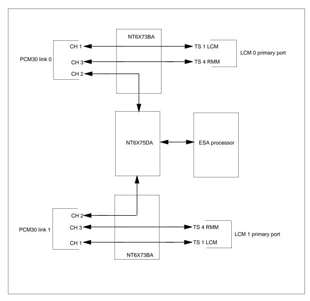
Under normal operation, an ESA uses time slot 3 (PCM30 channel 2) on PCM30 link 0 or 1 to host the DMS-X message channel. The next diagram displays the NT6X75DA in ESA mode.
