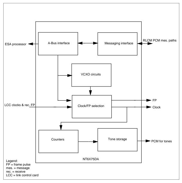
The NT6X75DA circuit card interfaces with the ESA processor in the ESA subsystem. This interface occurs through circuits on the NT6X75DA circuit card which conforms to the A-Bus standard. The ESA processor provides control information for adjusting the voltage controlled crystal oscillator (VCXO) and selection data for selecting the clock source which synchronizes the VCXO, clock and frame pulse signals.
