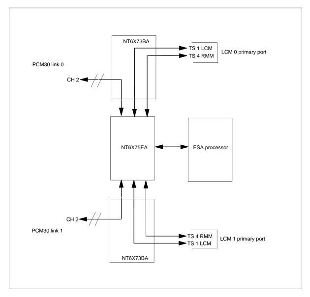
When the LCC is in ESA mode, time slot 1 from each LCM switches to the NT6X75EA from its normal PCM30 path. The ESA processor replaces the LGC as the host and the LCM continues to function as before.
