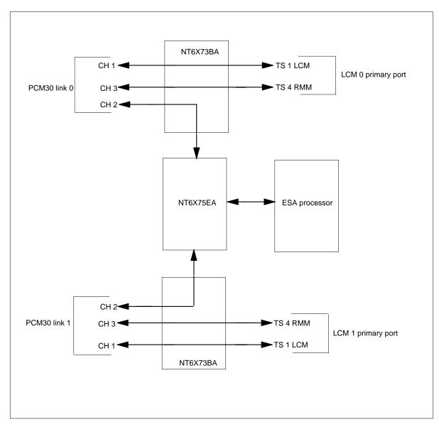
Under normal operation, an ESA uses time slot 3 (PCM30 channel 2) on PCM30 link 0 or 1 to host the DMS-X message channel. The next diagram displays the NT6X75EA in ESA mode.
