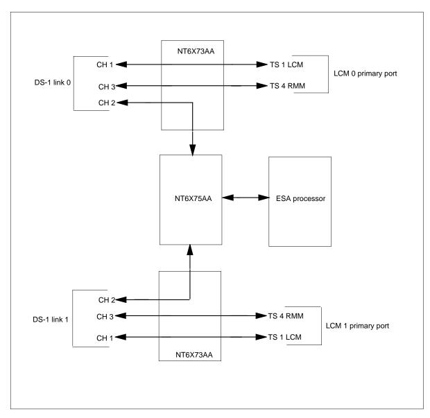
Under normal operation, an ESA uses time slot 3 (DS-1 channel 2) on DS-1 link 0 or 1 to host the DMS-X message channel. The next diagram displays the NT6X75AA in ESA mode.
