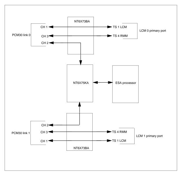
Under normal operation, an ESA uses time slot 3 (PCM30 channel 2) on PCM30 link 0 or 1 to host the DMS-X message channel. The next diagram displays the NT6X75KA in ESA mode.
