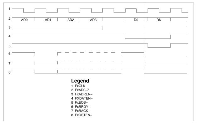
The LIU7 to RA F-bus protocol timing for the NT9X73AA appears in the following figure.
