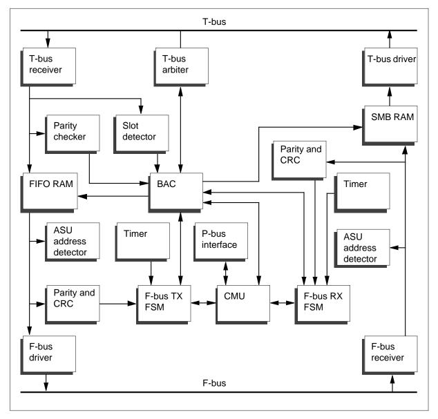
The BAC stores and retrieves messages when either the F-bus or the T-bus interface requests an operation. The BAC connects to the SMB RAM in order to store messages from the F-bus and to transmit messages on the T-bus. It also
