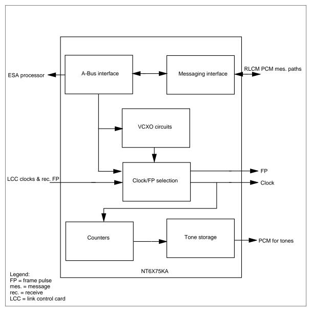
The NT6X75KA circuit card interfaces with the ESA processor in the ESA subsystem. This interface occurs through circuits on the NT6X75KA circuit card which conforms to the A-Bus standard. The ESA processor provides control information for adjusting the voltage controlled crystal oscillator (VCXO) and selection data for selecting the clock source which synchronizes the VCXO, clock and frame pulse signals.
