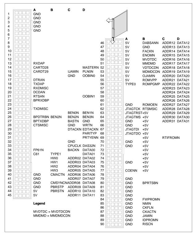
The following tables show the pin outs for the J1 (local interface connector) and the J2 (remote connection signal description) connectors.
