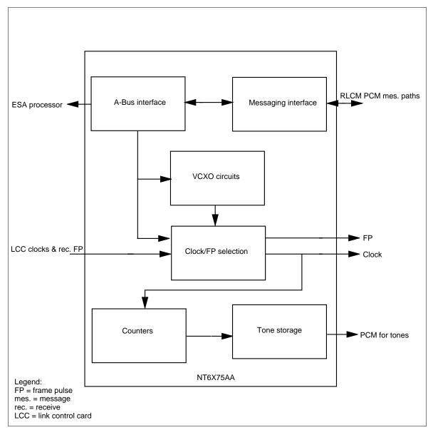
The NT6X75AA circuit card interfaces with the ESA processor in the ESA subsystem. This interface occurs through circuits on the NT6X75AA circuit card which conforms to the A-Bus standard. The ESA processor provides control information for adjusting the voltage controlled crystal oscillator (VCXO) and selection data for selecting the clock source which synchronizes the VCXO, clock and frame pulse signals.
