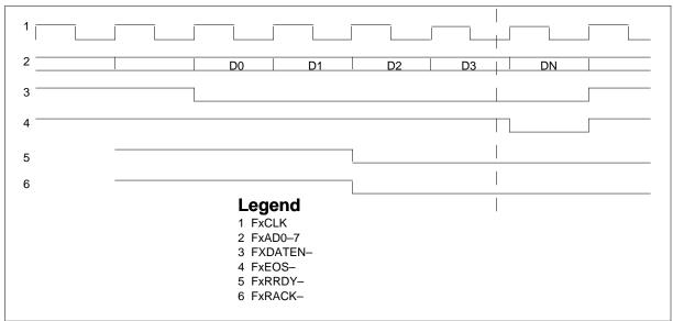
The F-bus arbitration timing for the NT9X73AA appears in the figure that follows.
