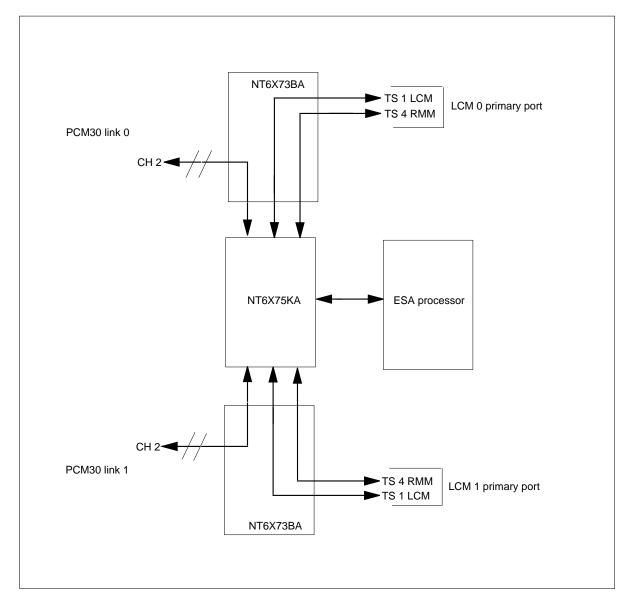
When the LCC is in ESA mode, time slot 1 from each LCM switches from its normal PCM30 path to the NT6X75KA. The ESA processor replaces the LGC as the host and the LCM continues to function as before.
