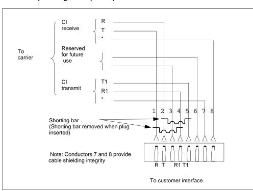
Figure 2-9 Connector pin assignment (RJ48X)
