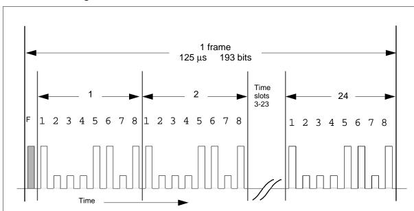
Figure 2-7 DS-1 frame bit assignment
