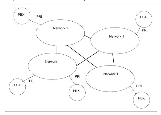
Figure 1-1 PRI provides access to the switched telephone network
