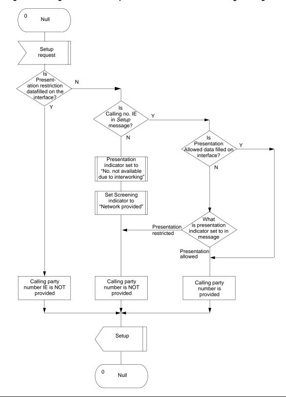
Figure 5-2 SDL diagram for calling line identification presentation/restriction at terminating exchange
