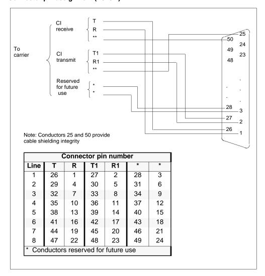
Figure 2-10 Connector pin assignment (RJ48M)
