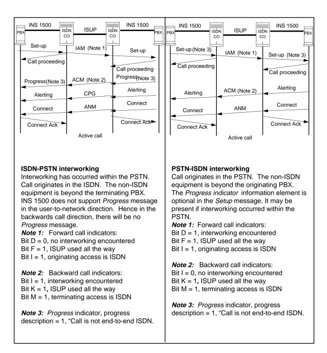
Figure 6-6 Message flow sequence diagram: Successful call setup procedure (continued)
