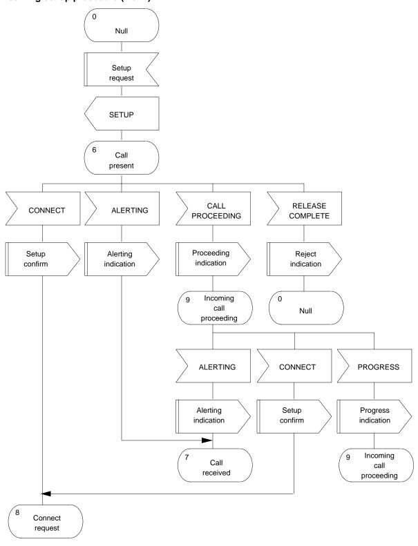
Figure 4-54 Overview protocol control: Network side (3 of 6) Incoming set up procedure (1 of 2)
