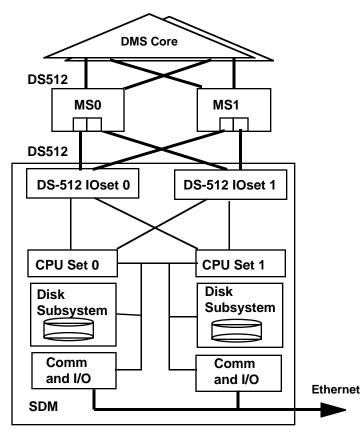
Fault Tolerant SDM/FT Block Diagram
